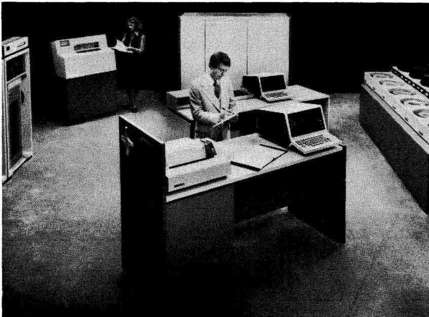
*The 1100/60 System supports up to four central processors and up to 8192K words of main memory. A single processor configuration can include a maximum of four consoles; a multiprocessor configuration, a maximum of seven consoles.*
