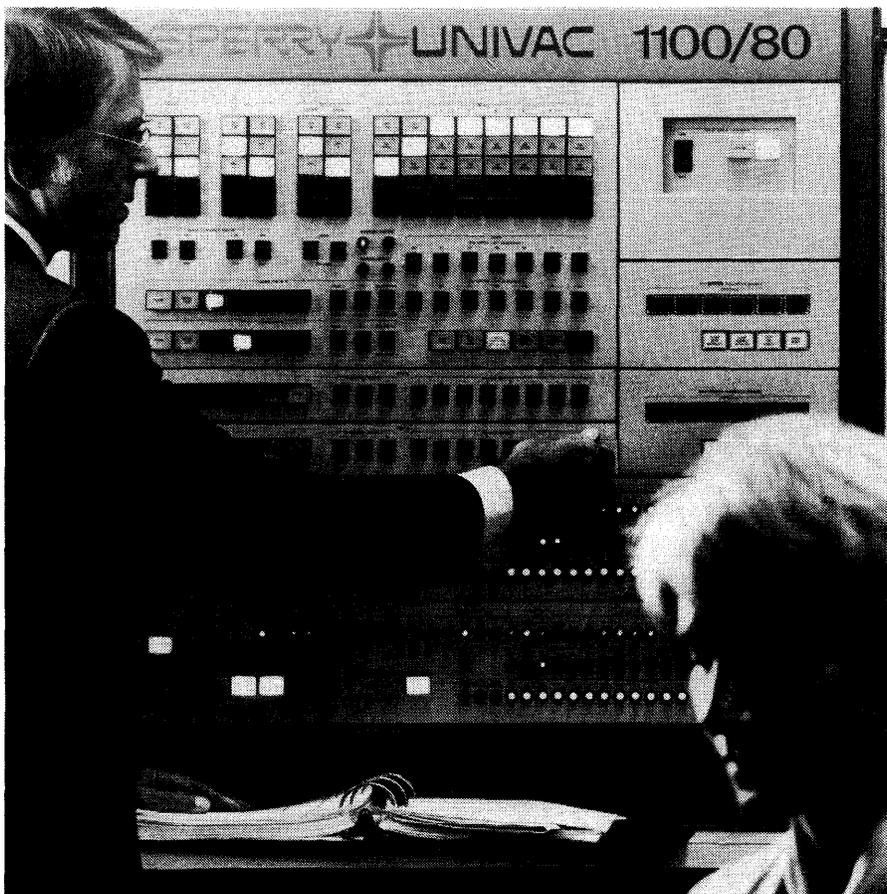
*The Sperry 1100/80 System is available in a number of different configurations and offers a choice of system sizes ranging from one CPU to four CPUs. There are five 1100/80 models with multiprocessing capabilities an integral part of the systems. An array processor subsystem for processing large amounts of arithmetic data is also available.*
