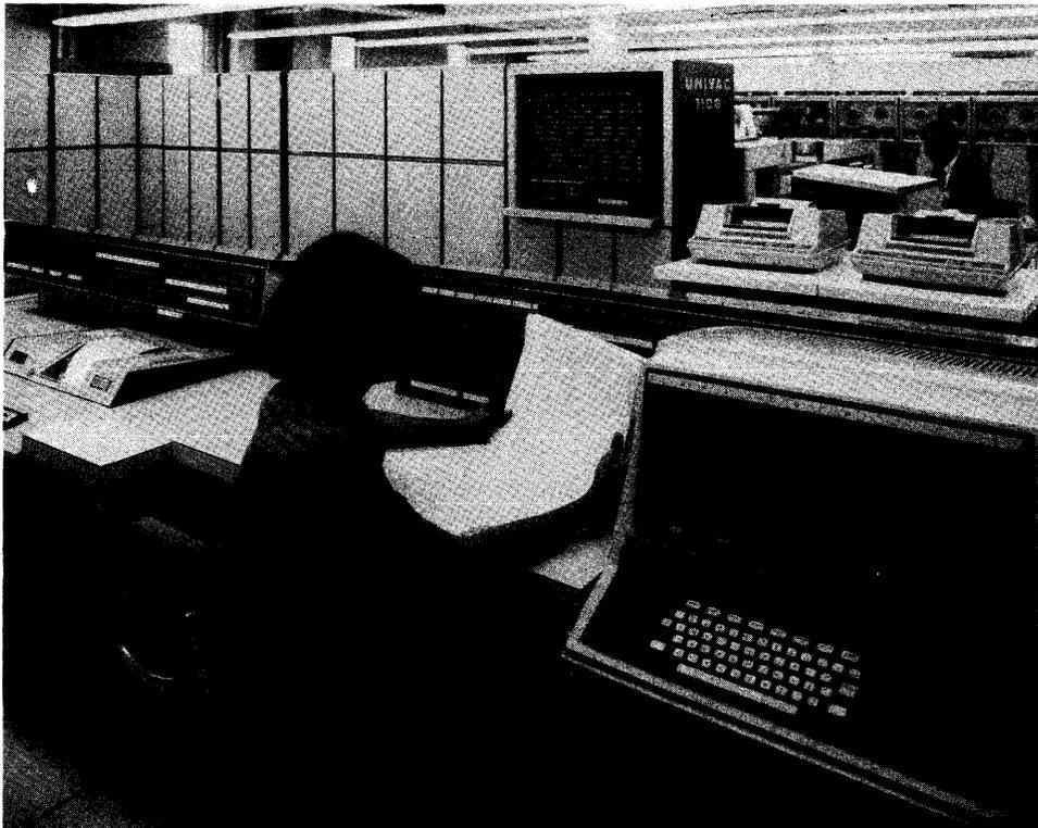
*The UNIVAC 1108 Display Console provides comprehensive system control facilities through a CRT display, Keyboard, Pagewriter, and indicator panel.*
