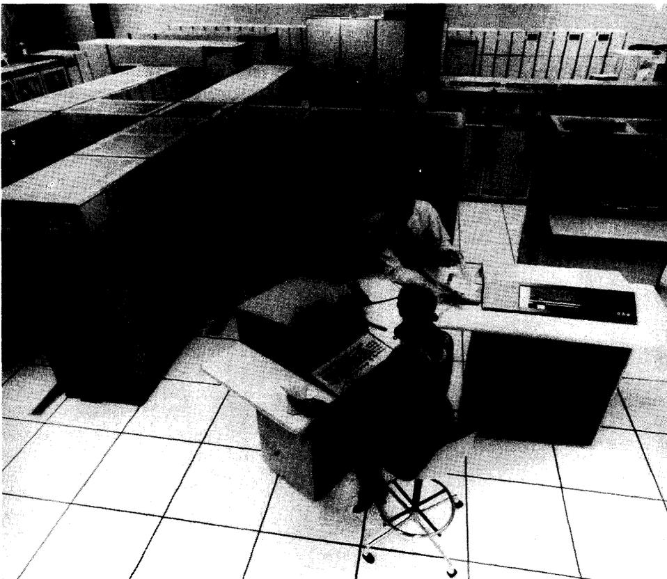
*Dual-processor UNIVAC 1110 systems such as the one shown here are expected to achieve three to five times the performance of UNIVAC 1108 Unit Processor systems.*
