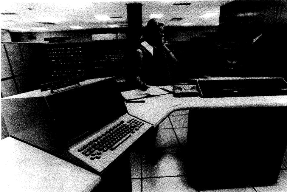
*The 1110 System Console, used to monitor and direct the system's functions, consists of a Uniscope 100 CRT display, keyboard, and Pagewriter printer.*
