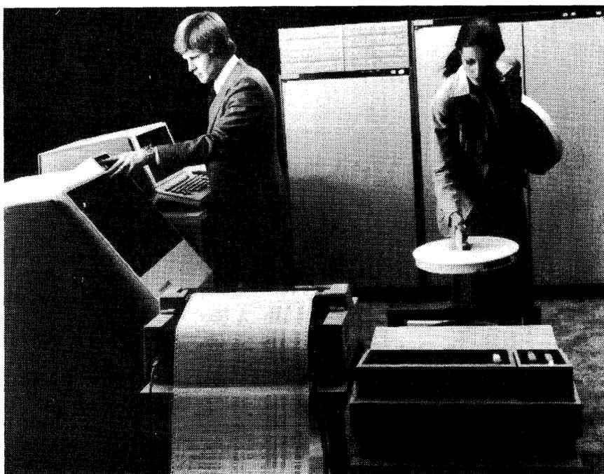
The DCP/40 is constructed with the same multi-microprocessor architecture as the 1100/60 processor. It can have over two million bytes of main-storage and up to 16 I/O processors. Each I/O processor can control up to 16 communications lines. The DCP/40 is the hardware portion of the Telcon Intelligent Communications System.
