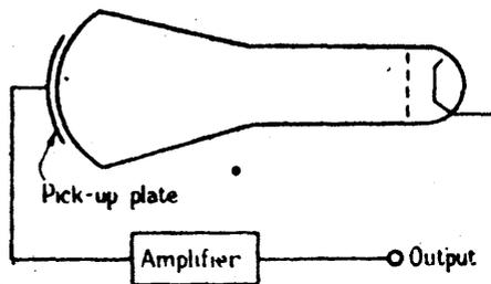
Fig. 3.—Detection of signals.
