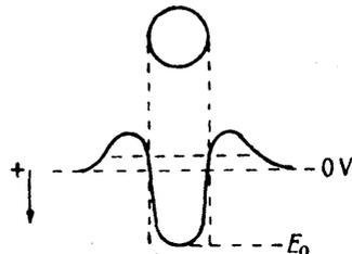
Fig. 7.—Potential distribution with a single spot—a "well."
