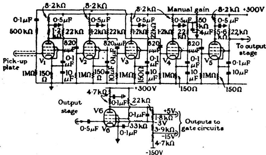
Fig. 31.—The amplifier circuit.
