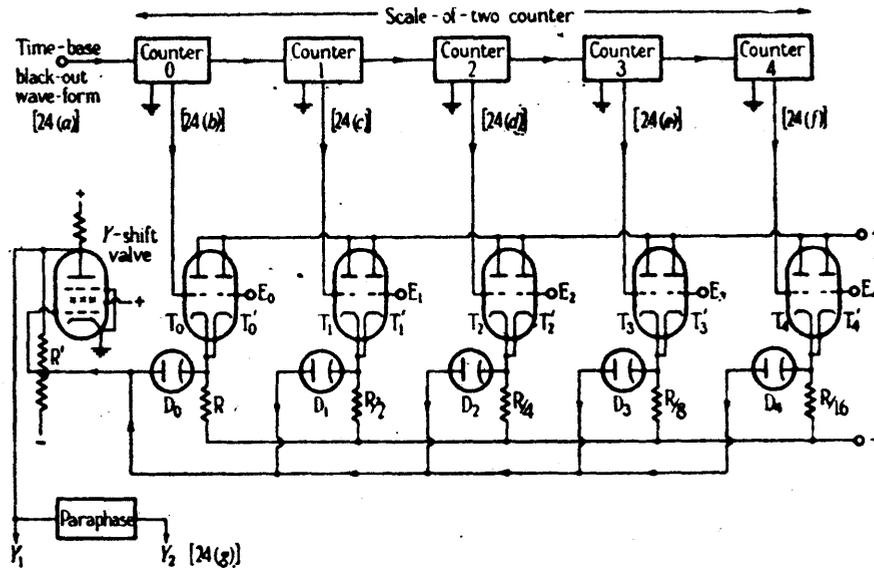
Fig. 23.—Simple Y-shift generator.
