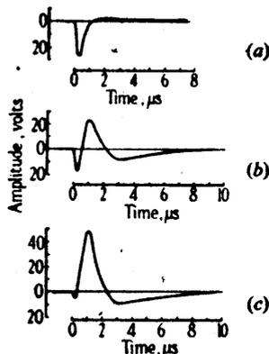
Fig. 13.—Output pulse at beam switch-on.
