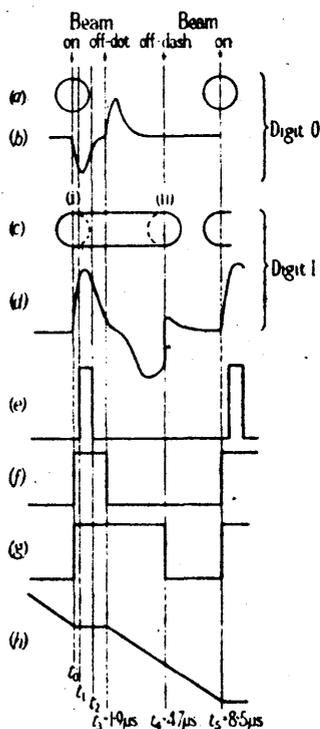
Fig. 14.—Dot-dash waveforms.
