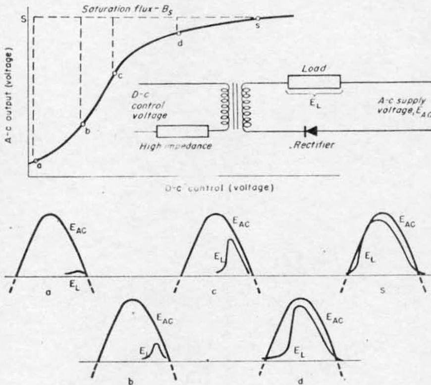
Fig. 2—Magnetization curve of a simple magnetic amplifier, and oscillograph traces of supply voltage relationships at points *a*, *b*, *c*, *d*, and *s* along the curve. The impedance in this circuit minimizes the flow of a-c current resulting from transformer action, and the rectifier prevents demagnetization on the negative half of the power cycle.
