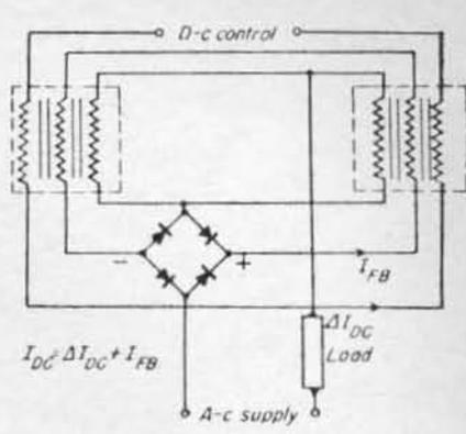
Fig. 5—Amplification factor of a magnetic amplifier can be increased by use of a feedback circuit. Saturation current is equal to the quantity shown.
