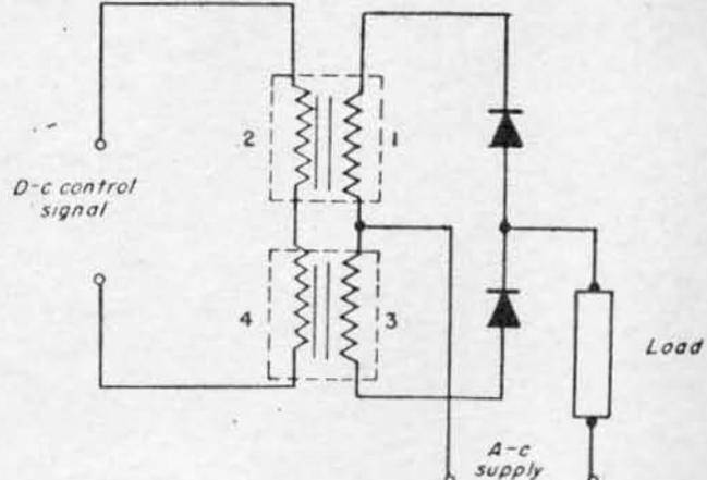
Fig. 9—Magnetic amplifier in which both the d-c feedback current and the a-c supply current flow in a common winding. Advantage of this circuit, is little complexity and low cost.
