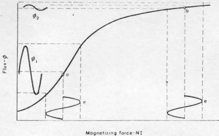
Fig. 1—Effect of saturation on an iron reactor. If *a* is the operating point, the back emf is large and only a small amount of current can flow. The converse is true if *b* is the operating point. A saturable reactor as used in the simplest form of magnetic amplifiers operates in a similar manner to regulate current flow.
