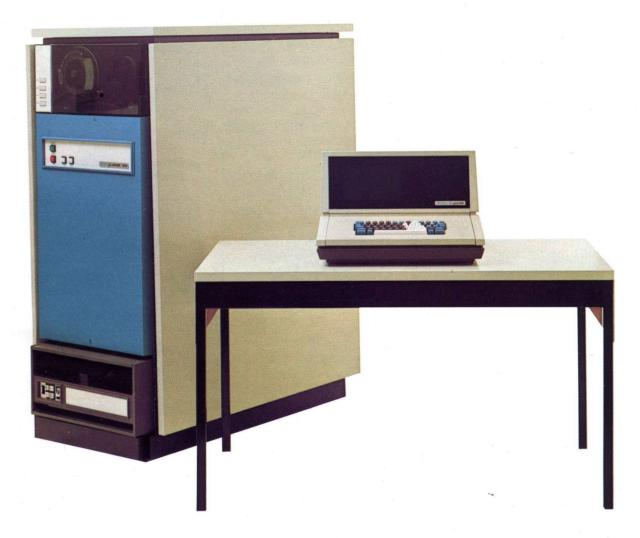
The SPERRY UNIVAC™ 1900 Computer-Assisted Data-Entry System (CADE) combines the versatility of a processor specifically designed for data entry with advanced solid-state storage and low-cost disc and tape subsystems to give you advantages of speed, economy and operating ease.
