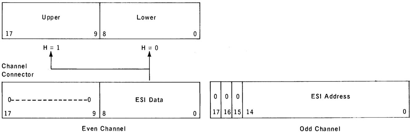
The following shows how 9-bit ESI data is transferred from main storage.
