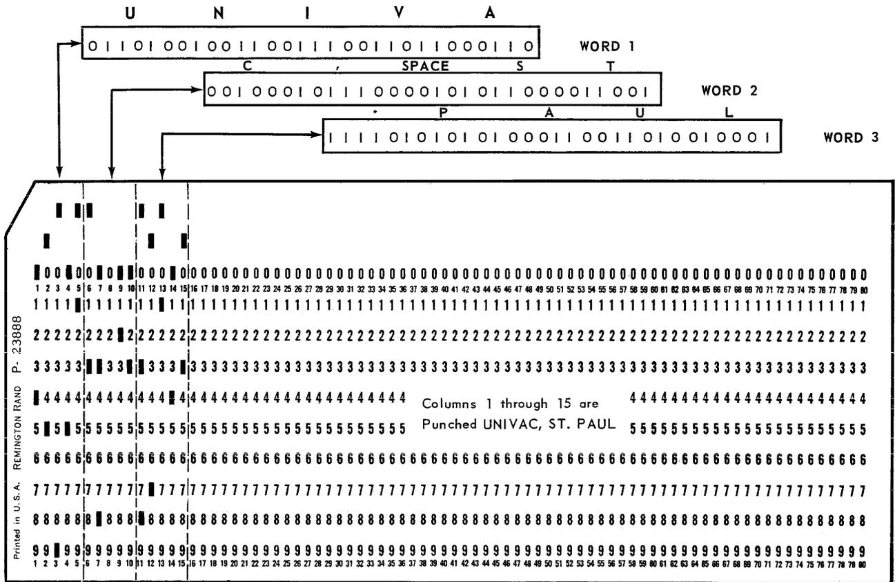
The data transfer to the Central Processor in this mode requires a minimum buffer area of 16 words for each card.
