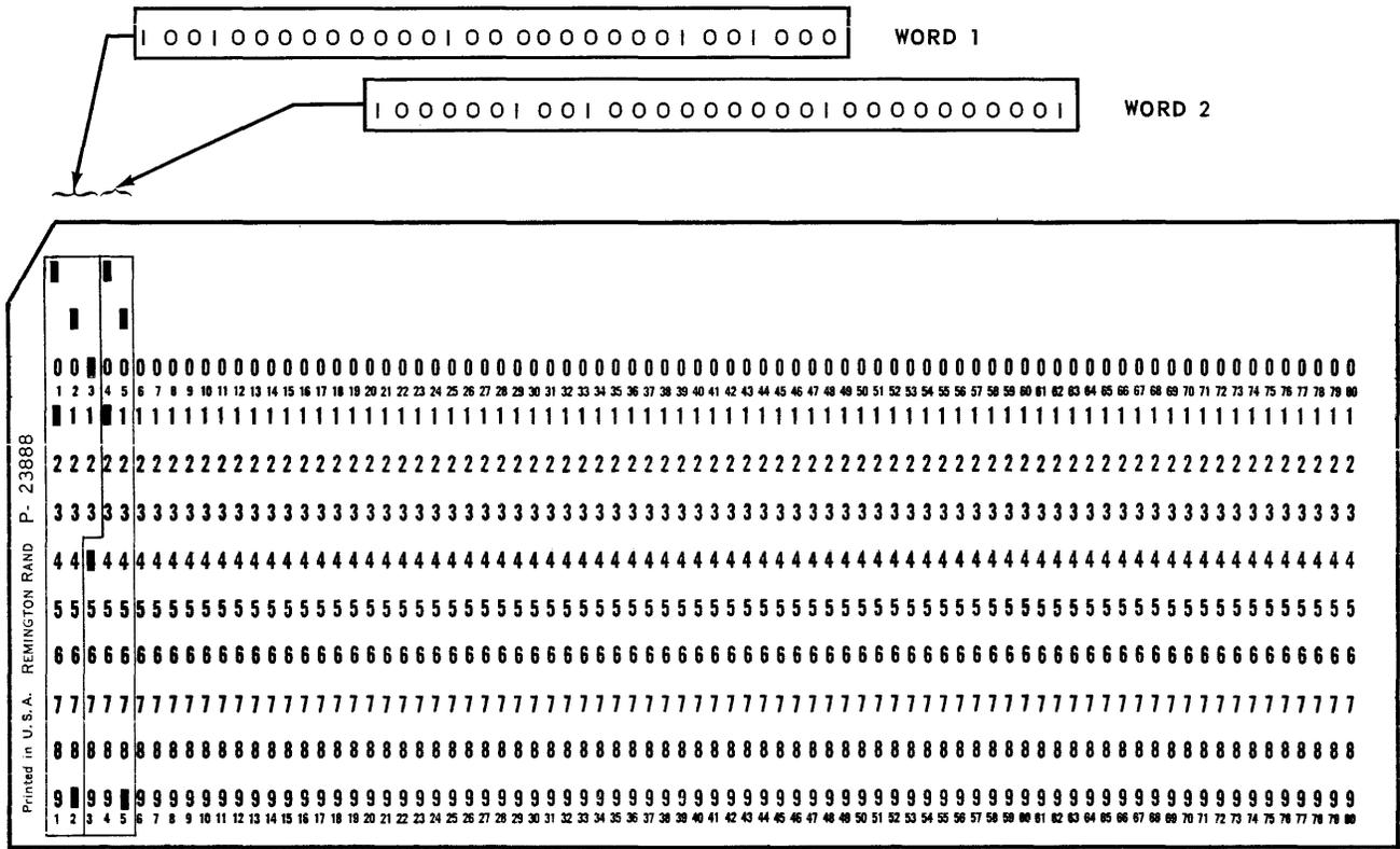
When data are transferred to the Central Processor in this mode, a minimum buffer area of 32 words is required for each card.
