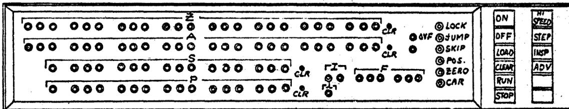
Power is applied to the 9140 Computer by depressing the ON switch. The switch lights when power is applied. If the OFF switch is depressed, the ON switch will become dark and power is removed. The procedure to start the 9140 Computer, high speed, is as follows:
