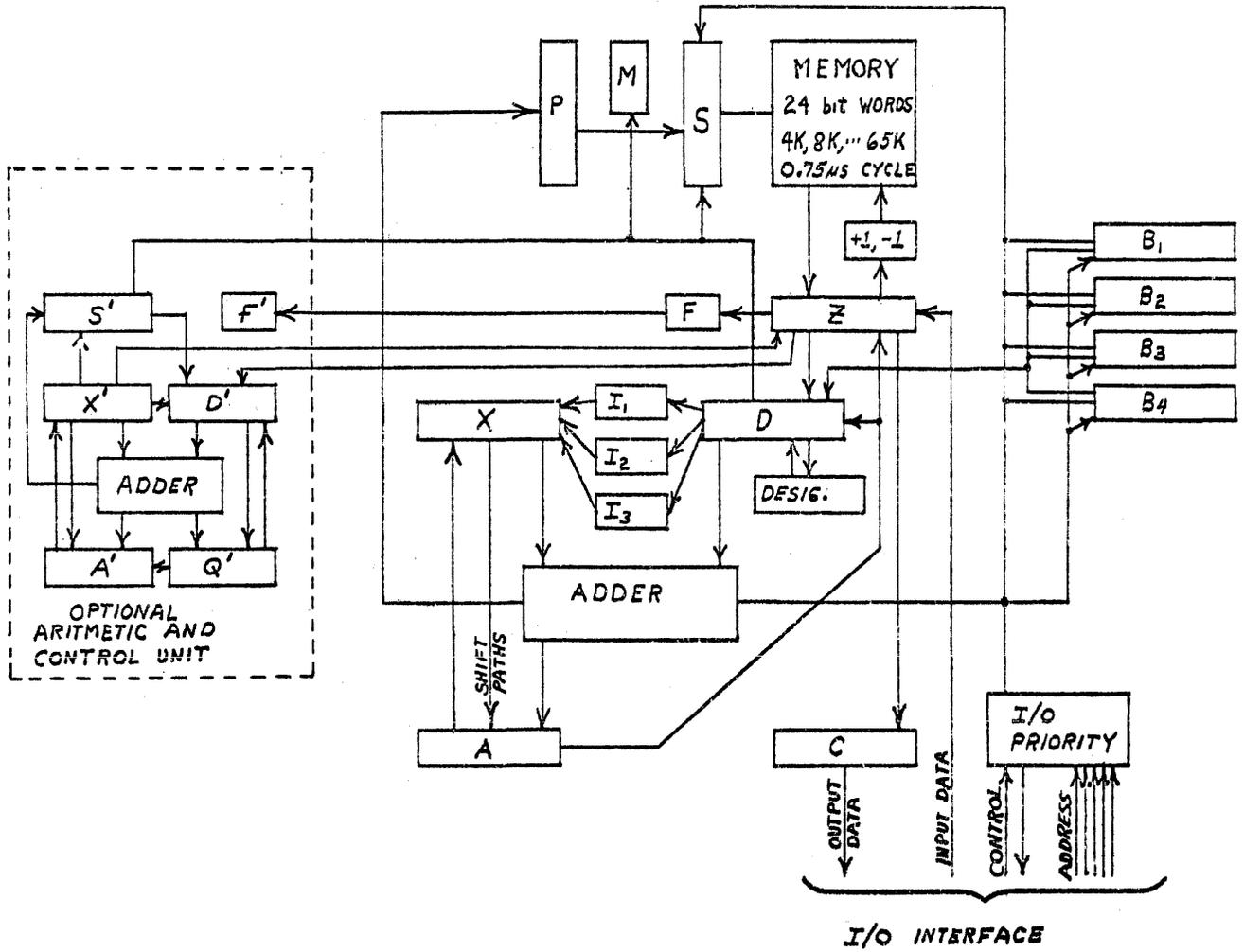
A - Accumulator Register. The A Register is twenty-four bits in length. It is normally used to hold the results of arithmetic and logical operations between instructions. The A Register is explicitly addressable by most instructions by setting  $Y = 1$ . The A Register is implicitly addressed and automatically accessed by those instructions which specify its use. The A Register is displayed on the operator panel as an aid for program debugging.
