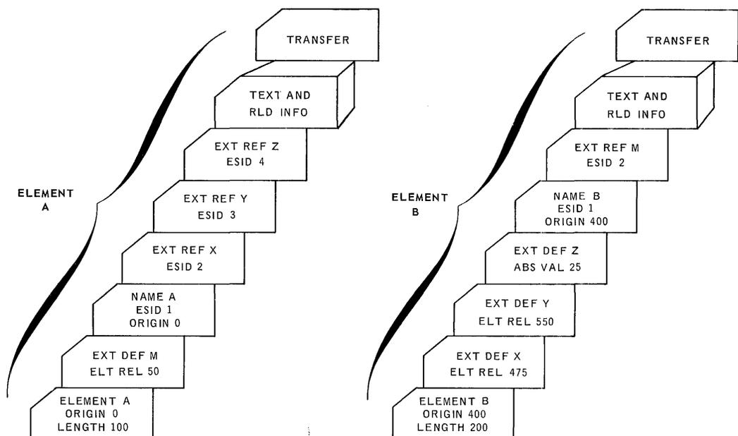
Figure 5-1. Elements A and B Deck Structure
