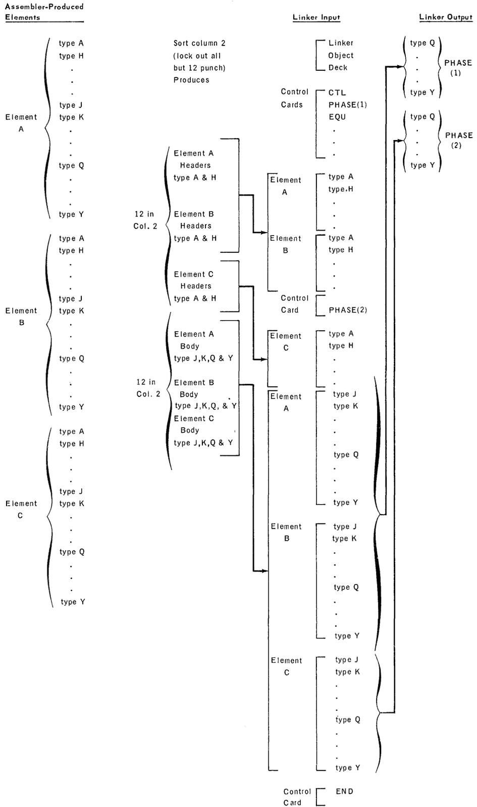
Figure 5-7. Linker Input Deck Sequence for One-Pass Operation
