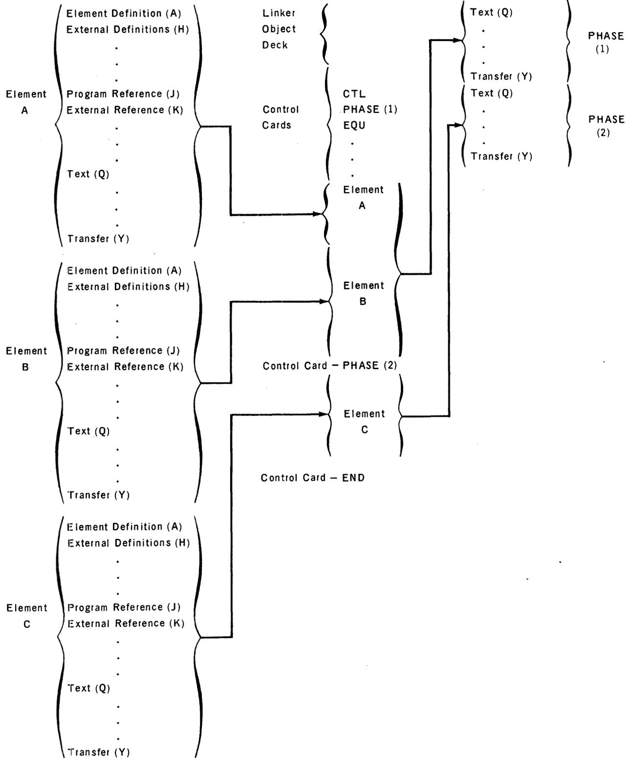
Figure 5-6. Linker Input Deck Sequence for Two-Pass Operation
