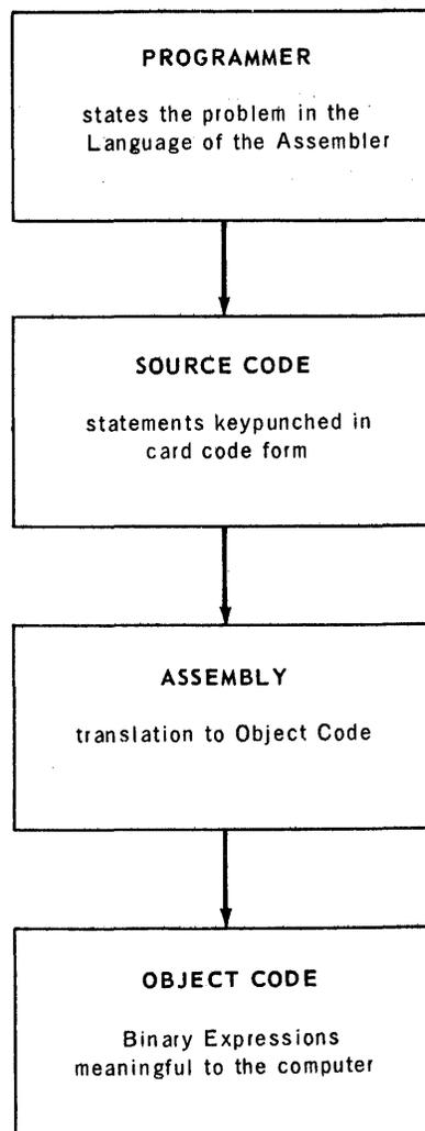
Figure 1-1. Source-to-Object Code Translation with Assembler
