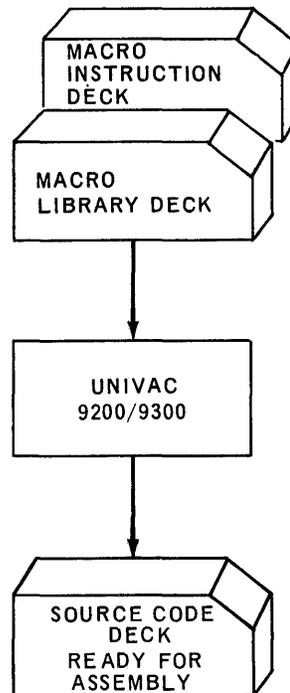
Figure A-1. Schematic of Preassembly
