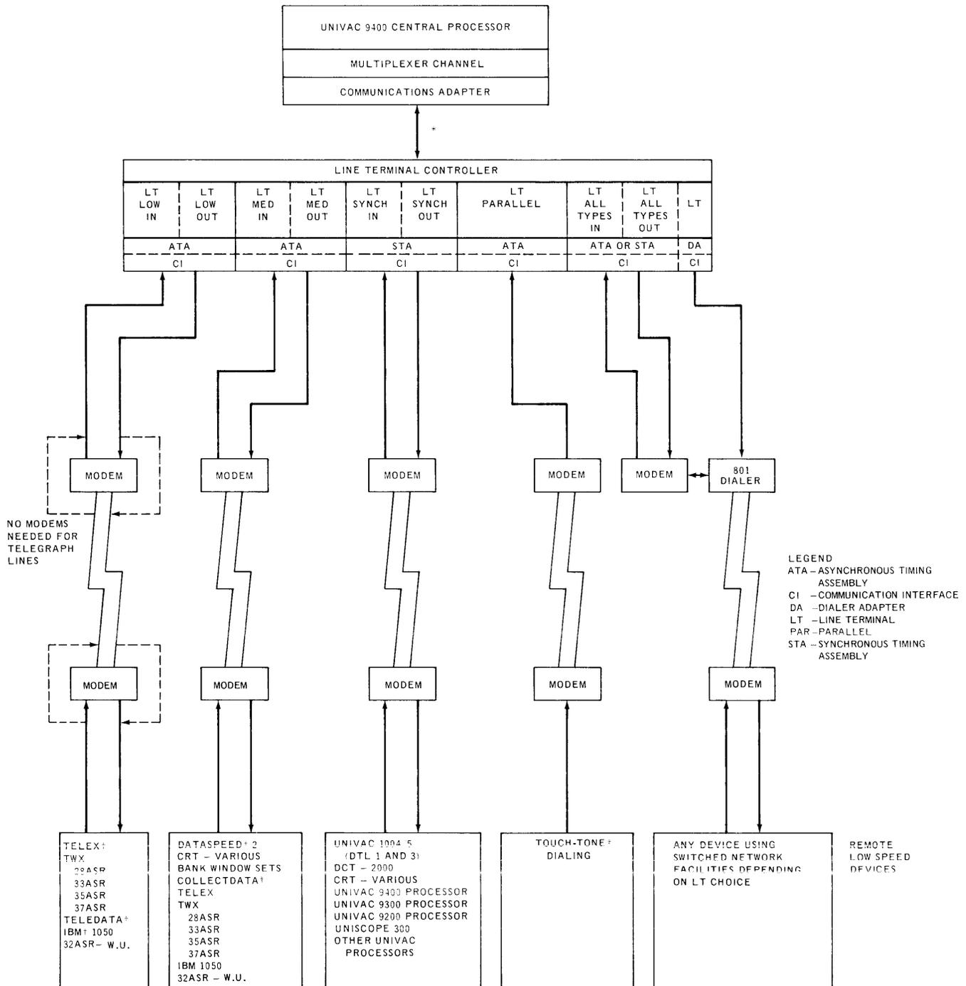
\* A SECOND UNIVAC 9400 CENTRAL PROCESSOR CAN BE CONNECTED TO THE DATA COMMUNICATION SUBSYSTEM (DCS-16) THROUGH THE USE OF THE DUAL CHANNEL ADAPTER. THIS CONNECTION IS MANUALLY SWITCHED AND ALLOWS ONLY ONE PROCESSOR AT A TIME TO INTERFACE WITH THE DATA COMMUNICATION SUBSYSTEM.
