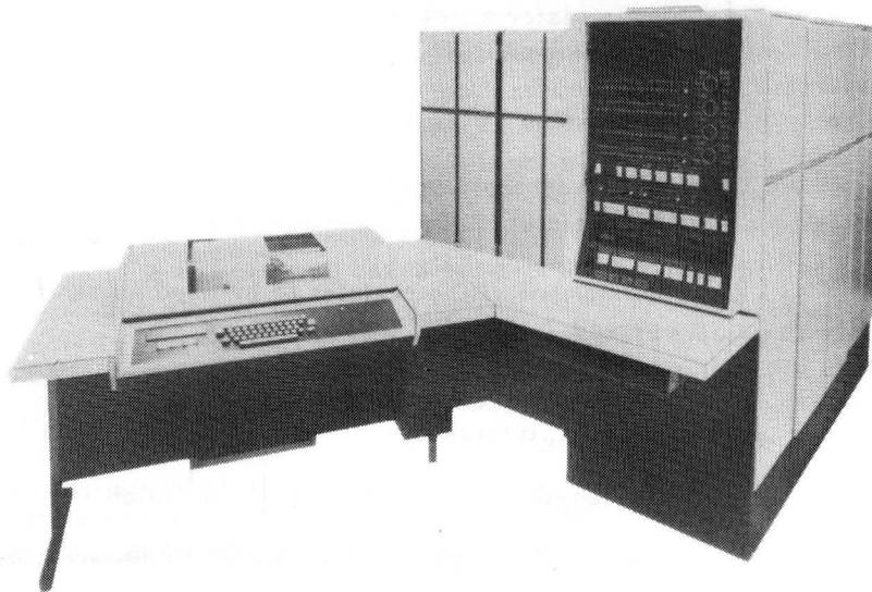
Figure 2-2. UNIVAC 9480 System Console
