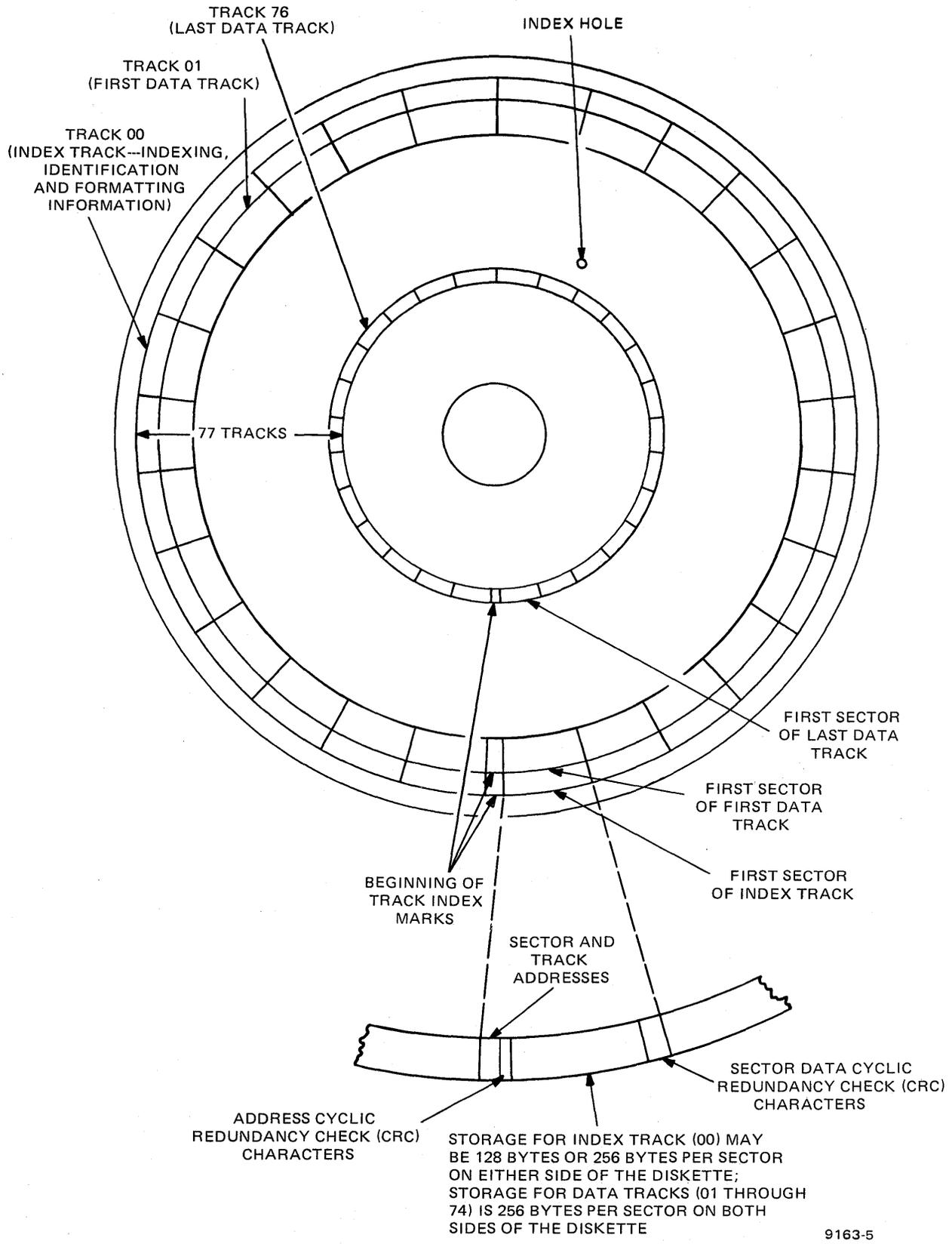
Figure 3-1. Diskette Track and Sector Format for Double Density (256 Bytes per Sector)
