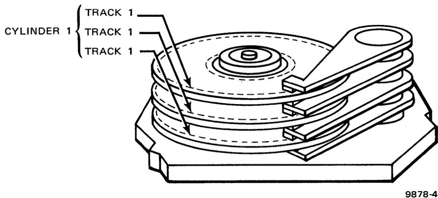
Figure 1-4. Disk Track and Cylinder Location
