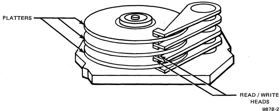
Figure 1-2. Disk Drive Assembly
