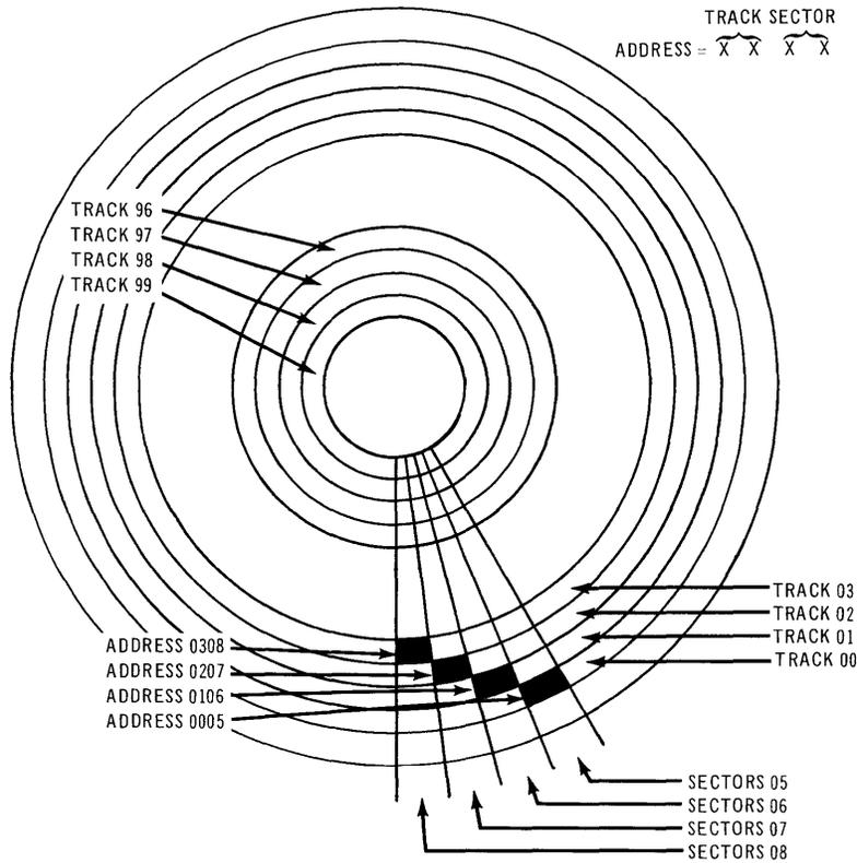
Figure 2-2. Disc Address Structure
