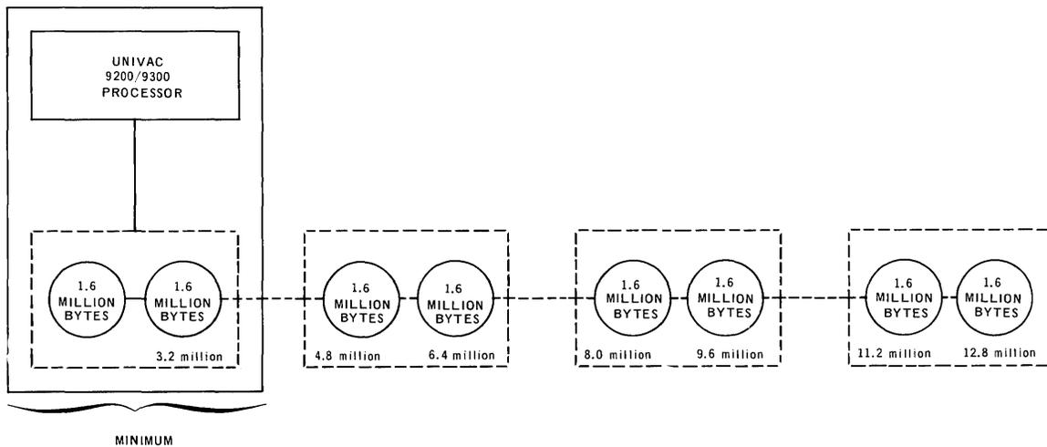
Figure 1-1. Minimum/Maximum Configuration
