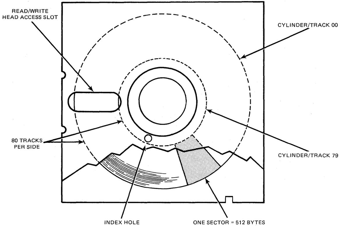
Figure 3-3. Track and Sector Format for Double-Density Diskettes (512 Bytes per Sector)
