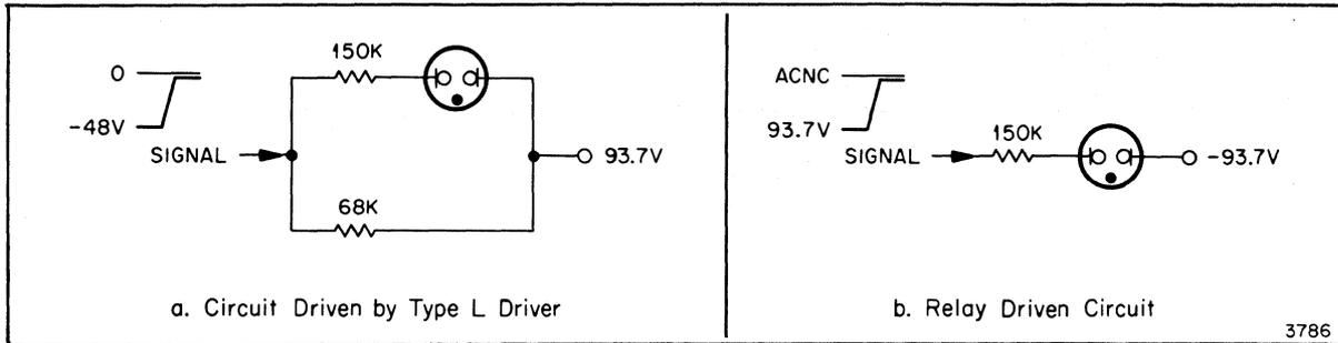
Figure 7-1. Neon Indicator Circuits
