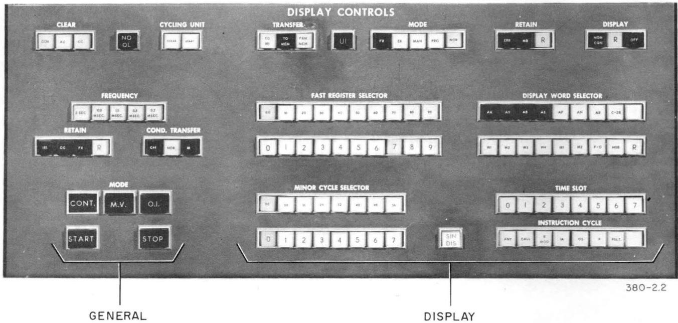
Figure 3-3. Computing-Unit Display-Control Panel
