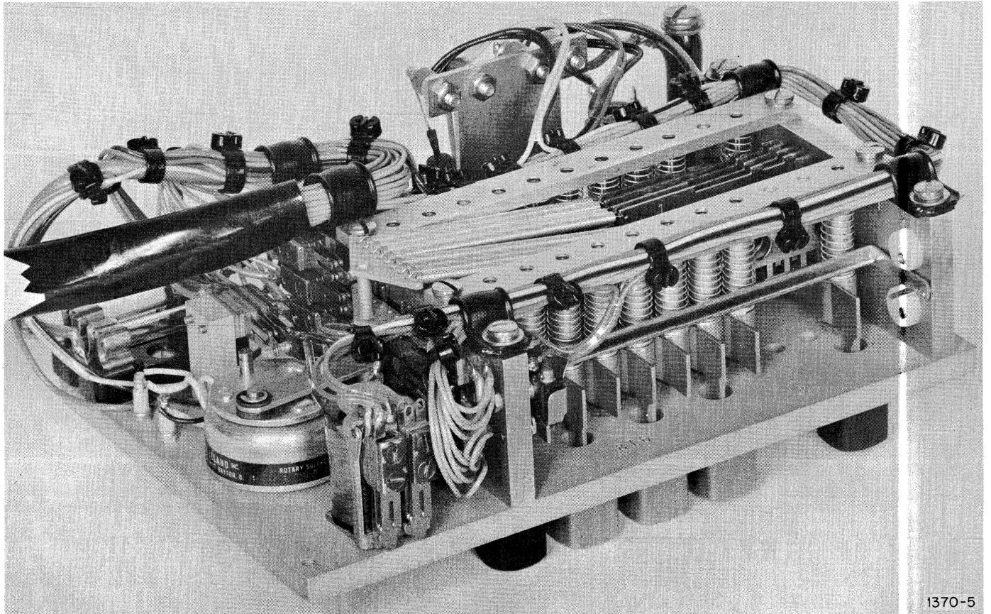
exercised in replacing the microswitch to avoid distortion of the microswitch bail. It should be noted that careful removal of the microswitch generally will not affect adjustment of the bail.
