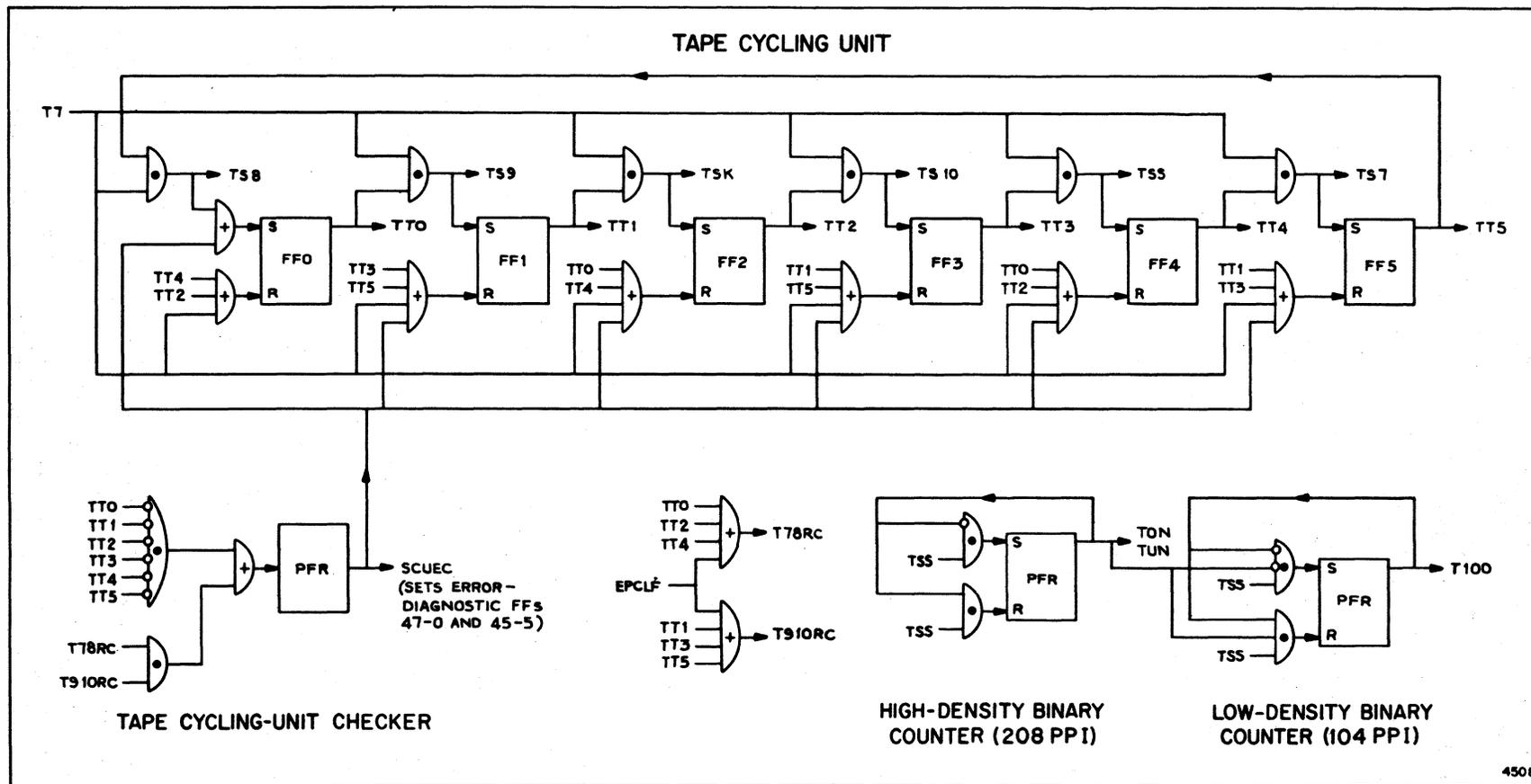
Figure 3-2. Tape Timing Signal Generator in Larc System, Serial 1 (D807 850)
