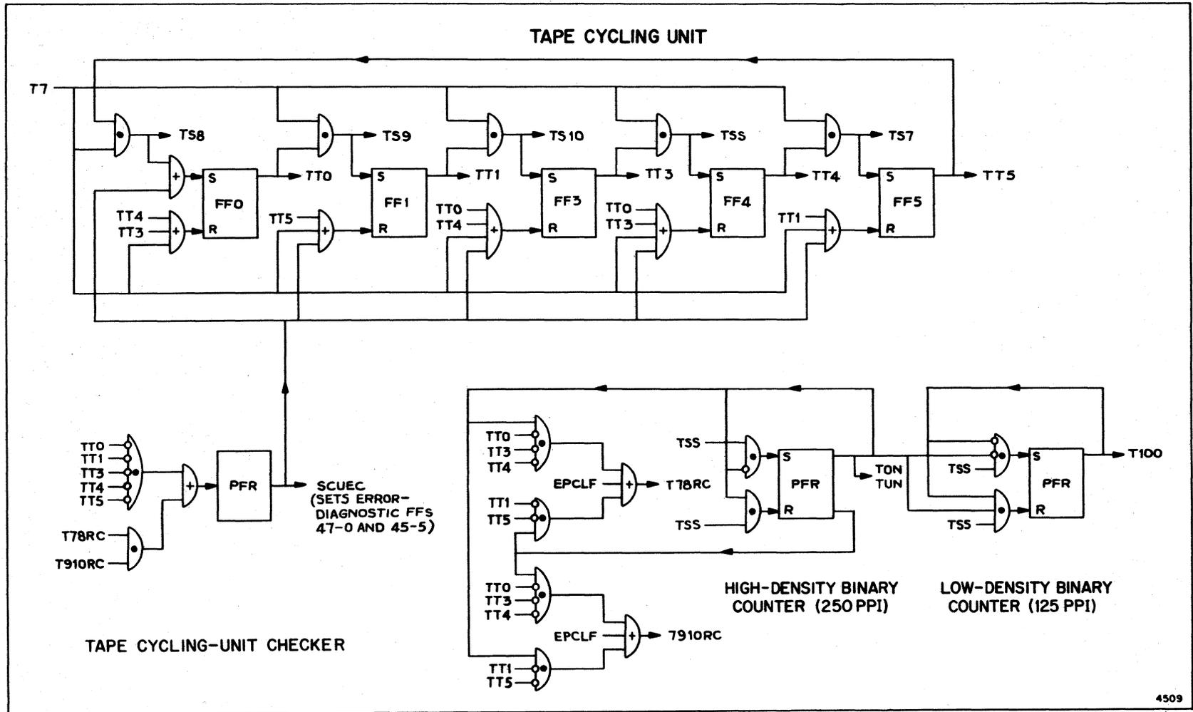
Figure 3-3. Tape Timing Signal Generator in Larc System, Serial 2 (D807 950)
