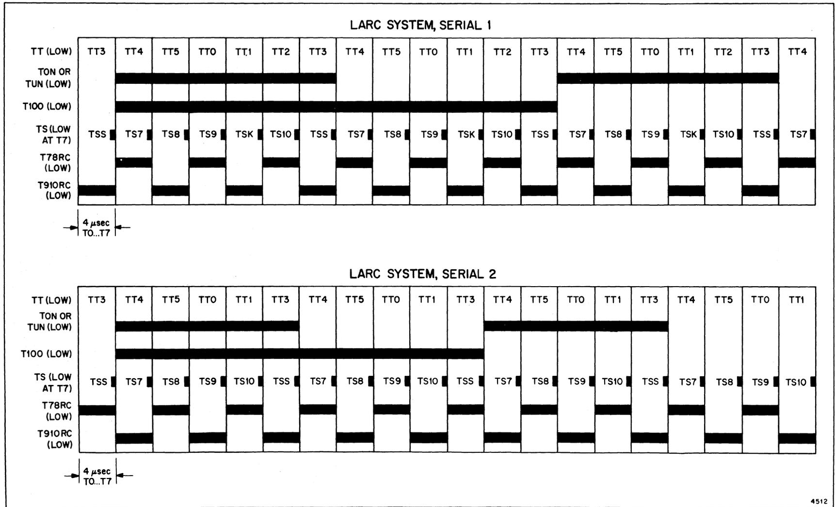
Figure 3-4. Tape Timing Signal Generator Outputs (Larc System, Serials 1 and 2)
