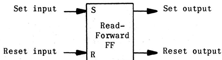
When the flip-flop is set, the set output is considered to be significant. Likewise, when the flip-flop is reset, the reset output is significant. The set and reset outputs are never significant at the same time, since one is always the logical inverse of the other. A setting pulse always overrides a resetting pulse. The flip-flop is assumed to change state 0.5  $\mu$ sec after it is set or reset.
