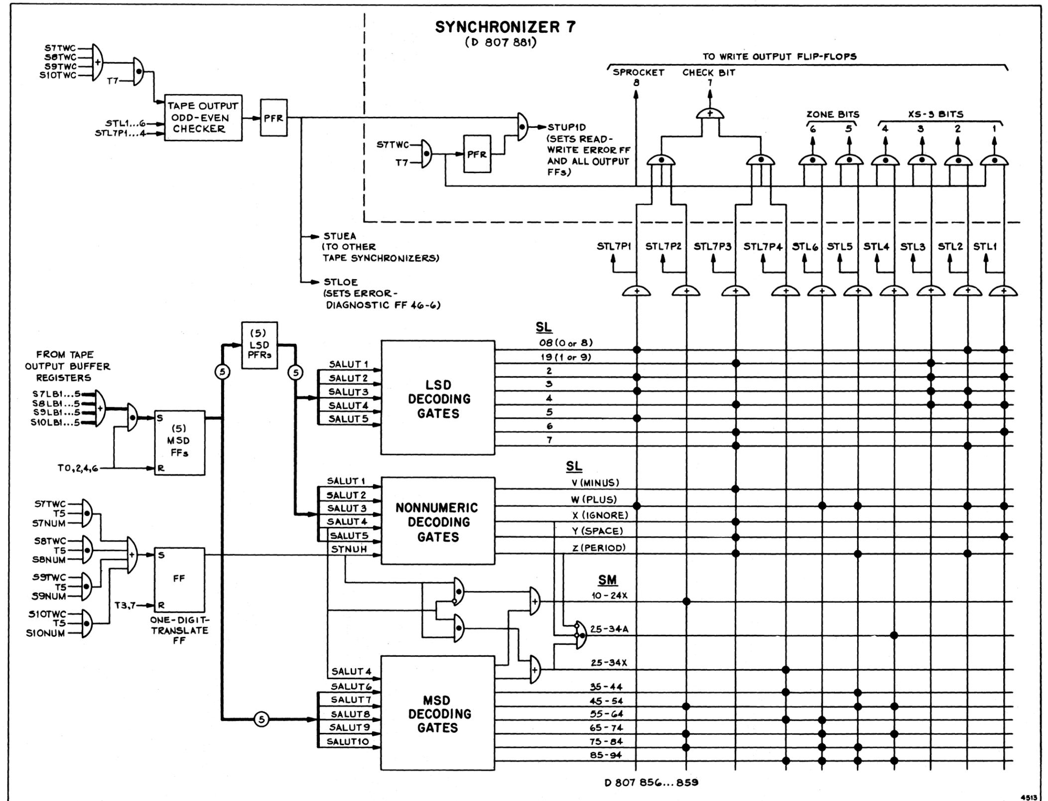
Figure 3-5. Larc-to-Univac Translator and Output Checker
