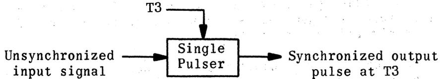
A single pulser is always followed by a pulseformer (PFR). This pulseformer, although not shown on the simplified logic diagrams, is assumed to be present when a single pulser is represented. A timing signal, if present, represents the time at which the synchronized output pulse appears at the output of the pulseformer which follows the single pulser.
