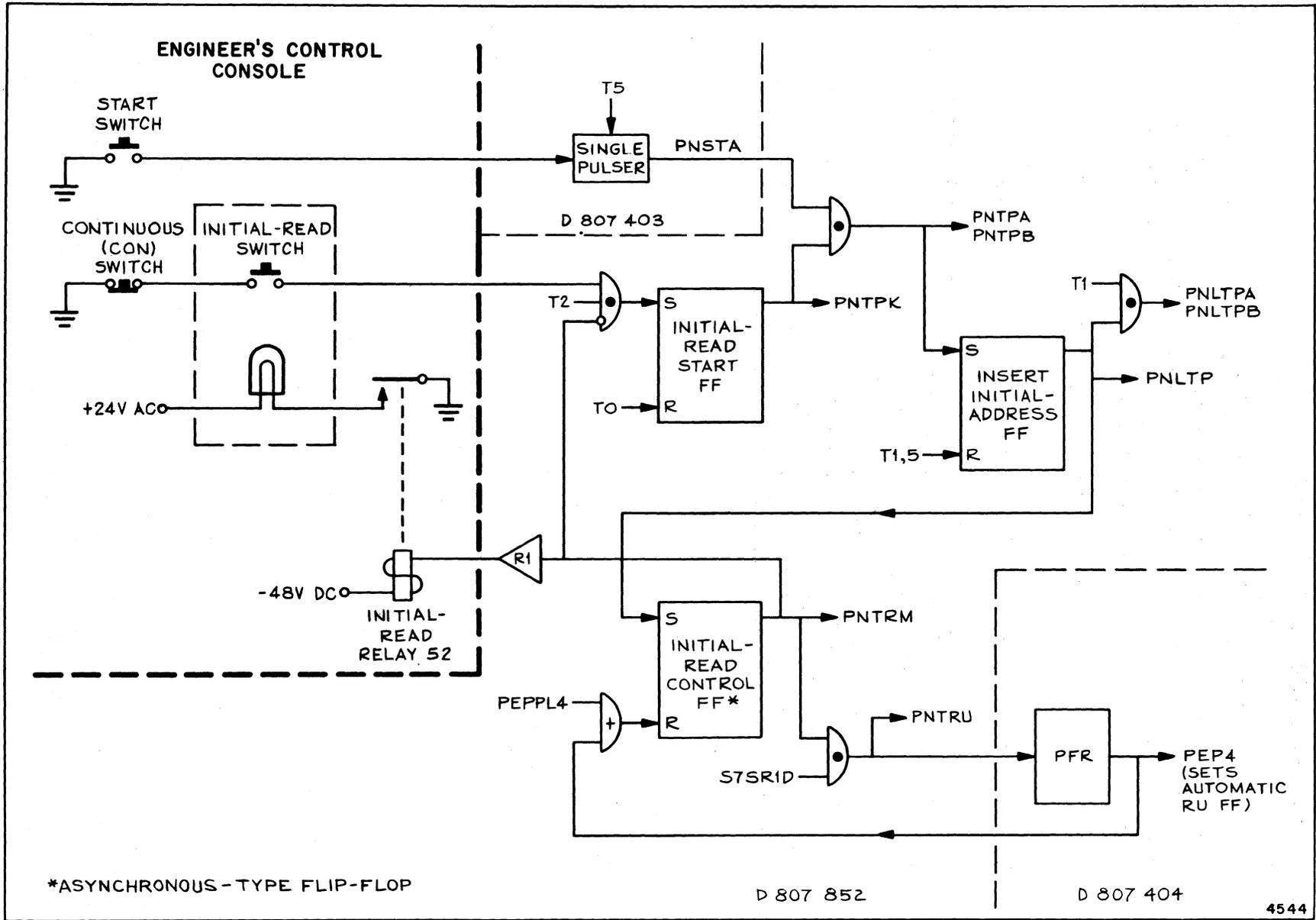
Figure A-1. Initial-Read Circuits (D 807 852)
