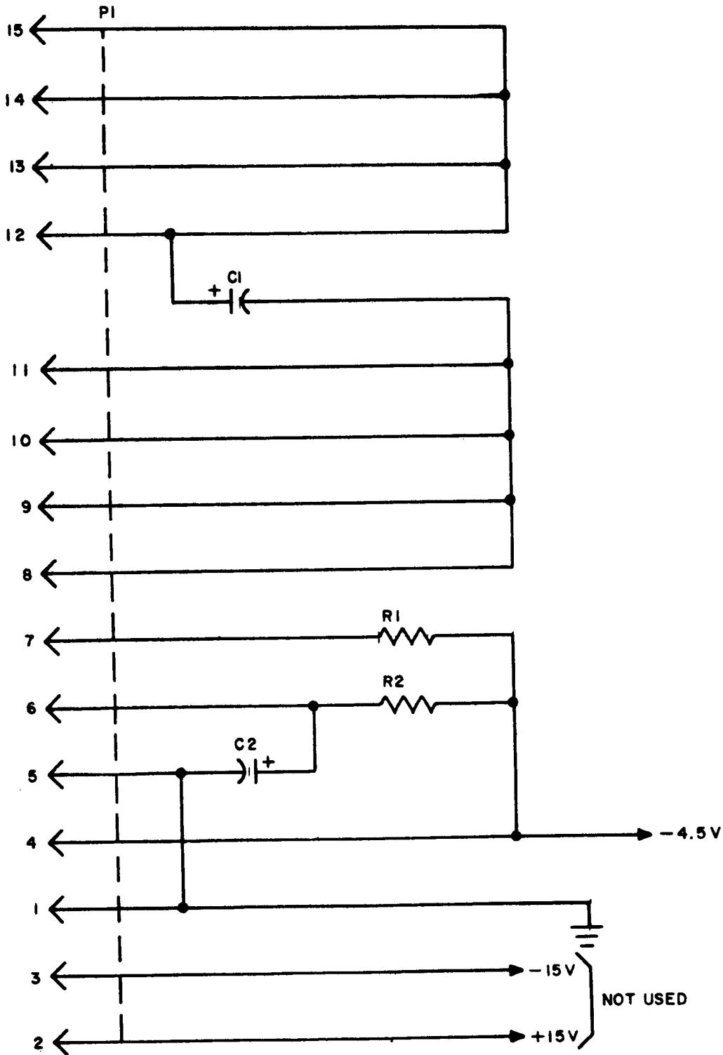
Figure 7-61. Capacitor - Resistor Assembly, Module 7109010 Schematic Diagram
