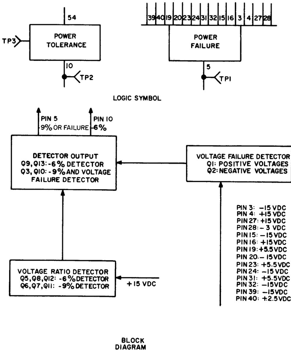
Figure 7-69. Voltage Sensor, Module 7500340
