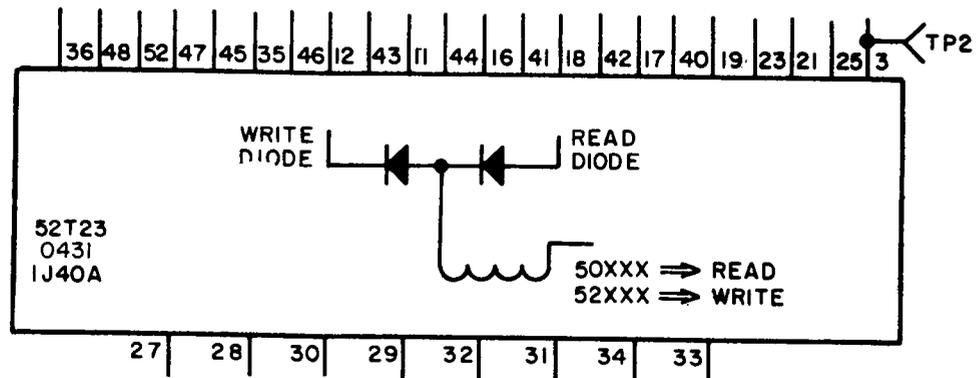
Figure 7-76. Logic Symbol of One Circuit on 7500431 Module
