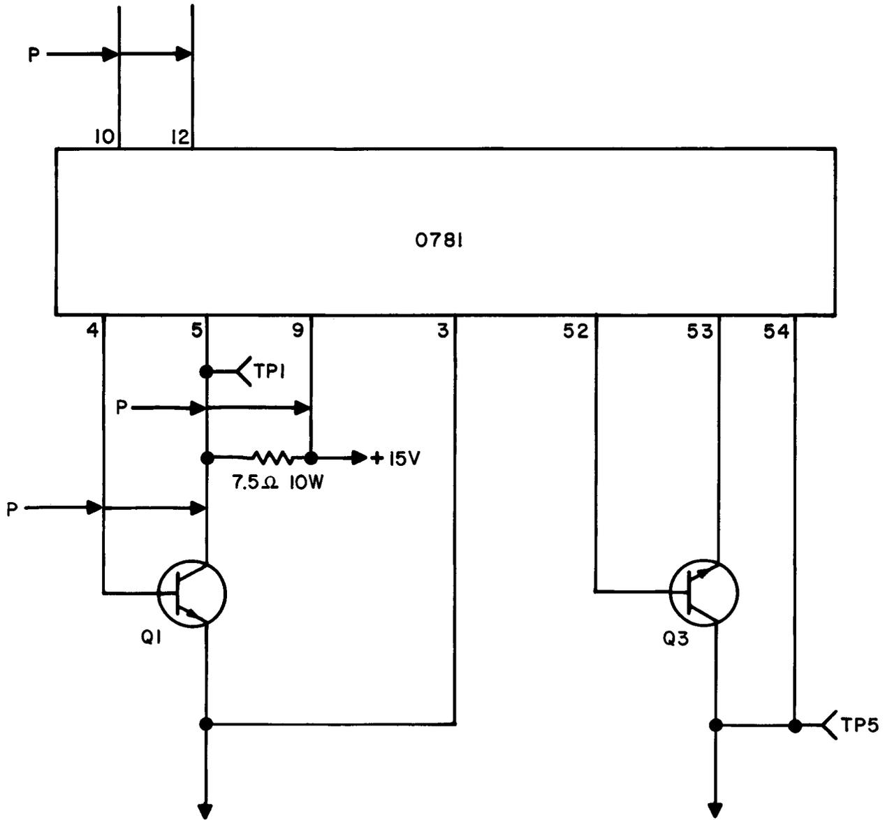
Figure 7-84. Logic Symbol of 7500781 Module
