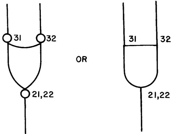
Figure 7-86. Logic Symbol of Noninverting Amplifier Driver, Module 7500900
