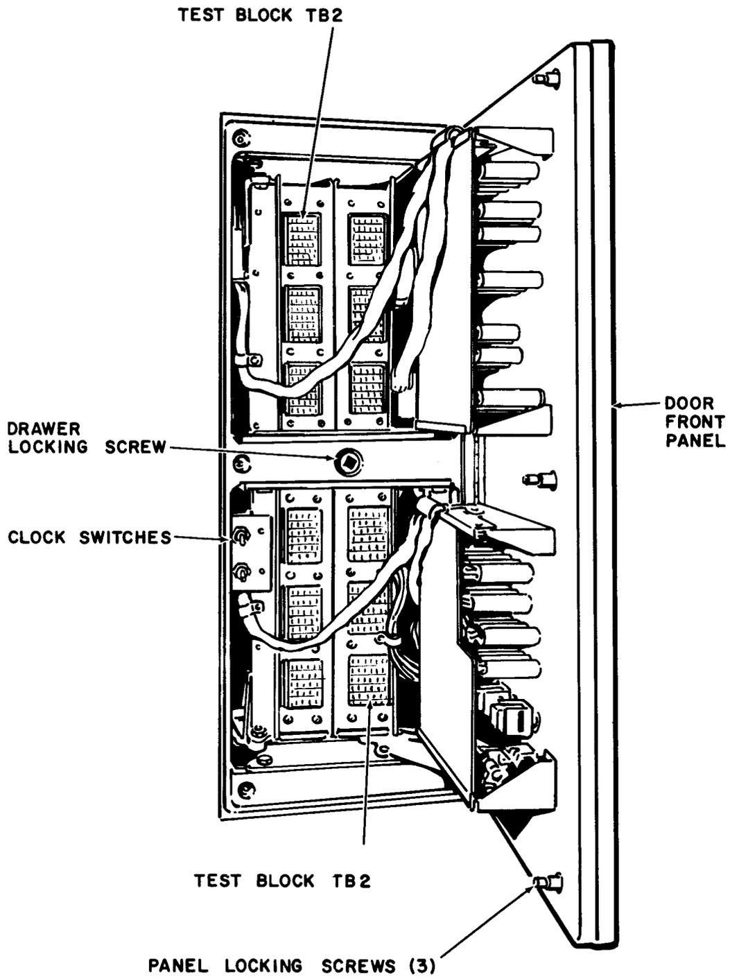
Figure 7-9. Location of Parts in Logic Drawer-Panel Opened
