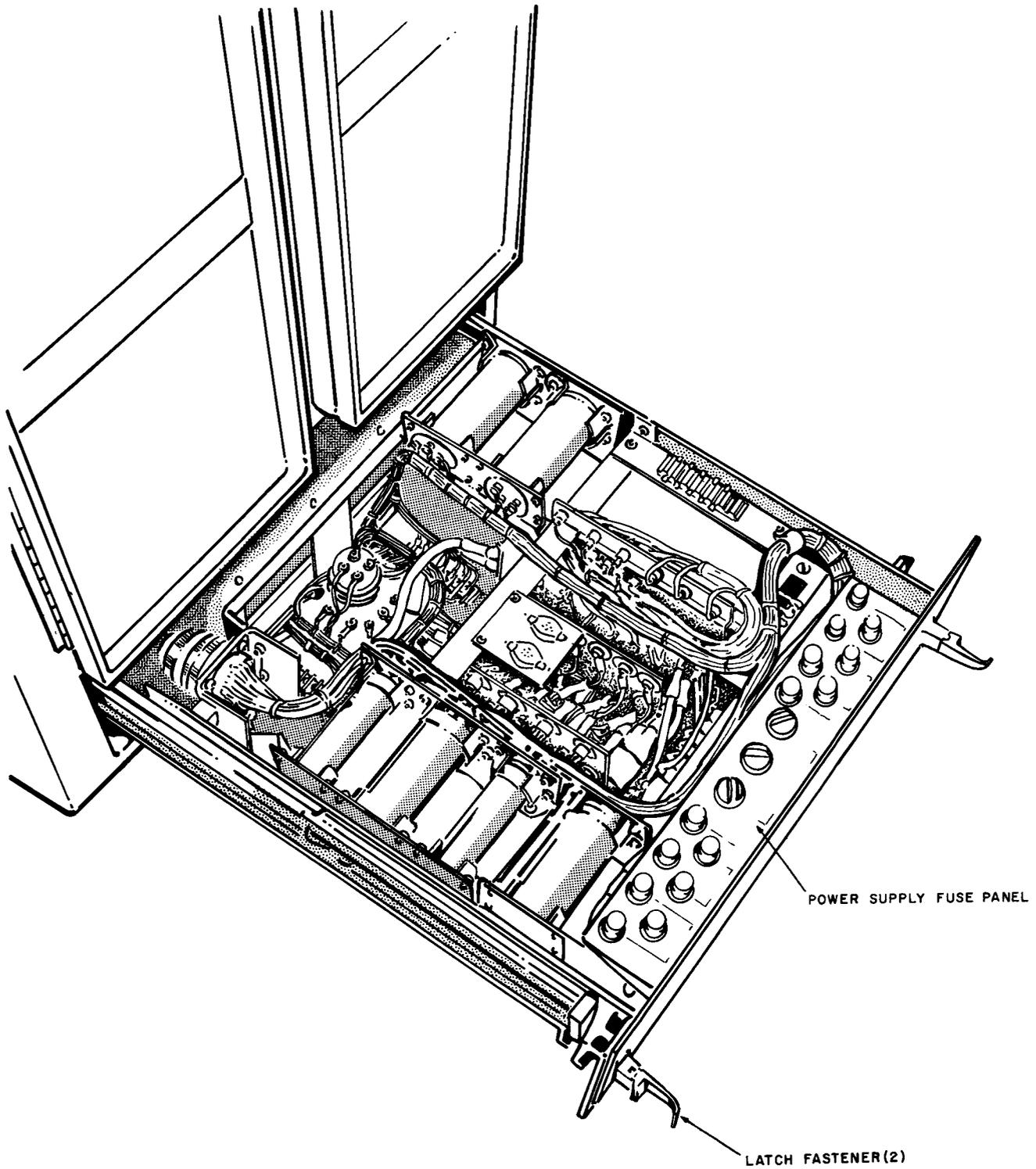
Figure 7-11. Extended Power Supply PS 1
