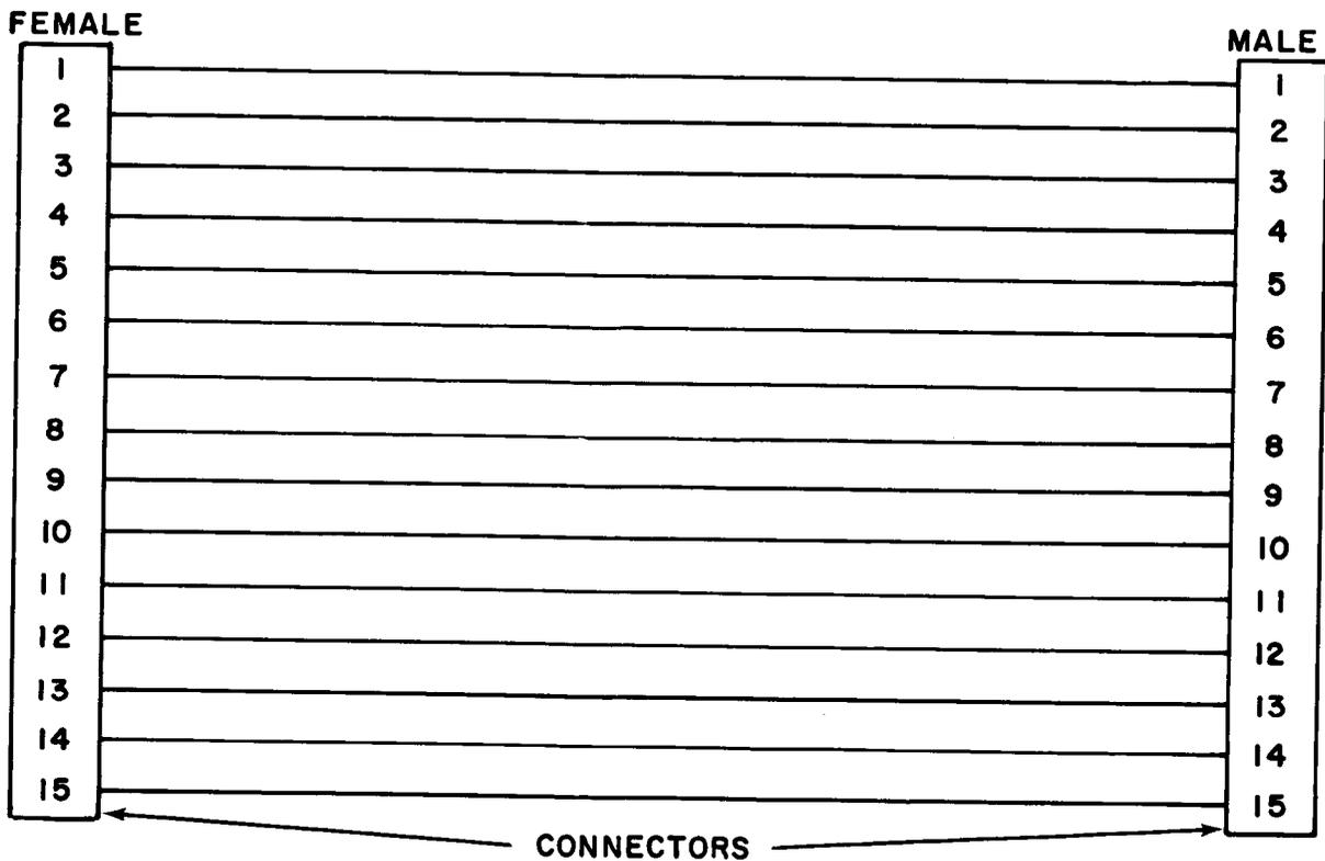
Figure 7-6. Module Extender, Wiring Diagram
