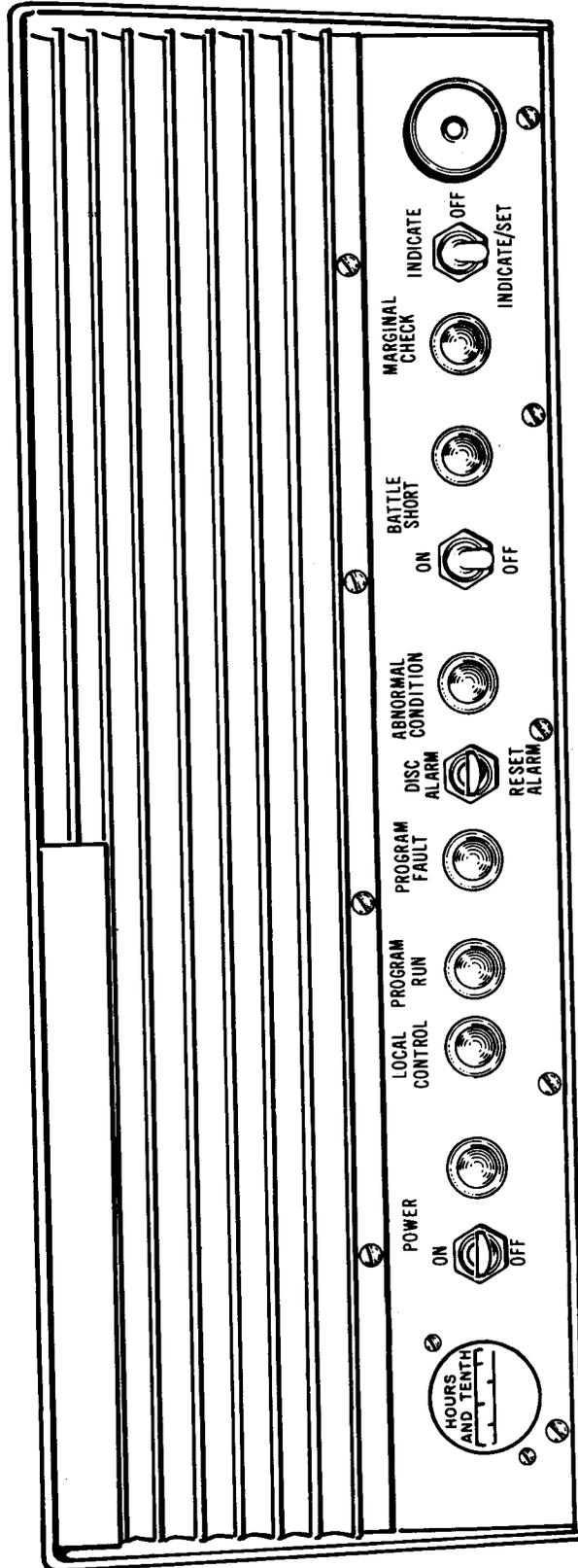
Figure 7-4. Maintenance Controls and Indicators - Power Control Panel (A5)
