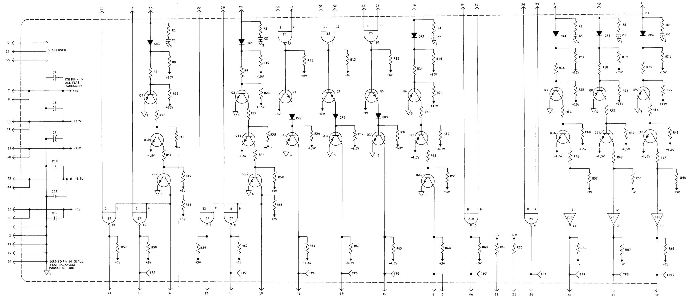
Figure 7-83. Module 7500761 Schematic Diagram
