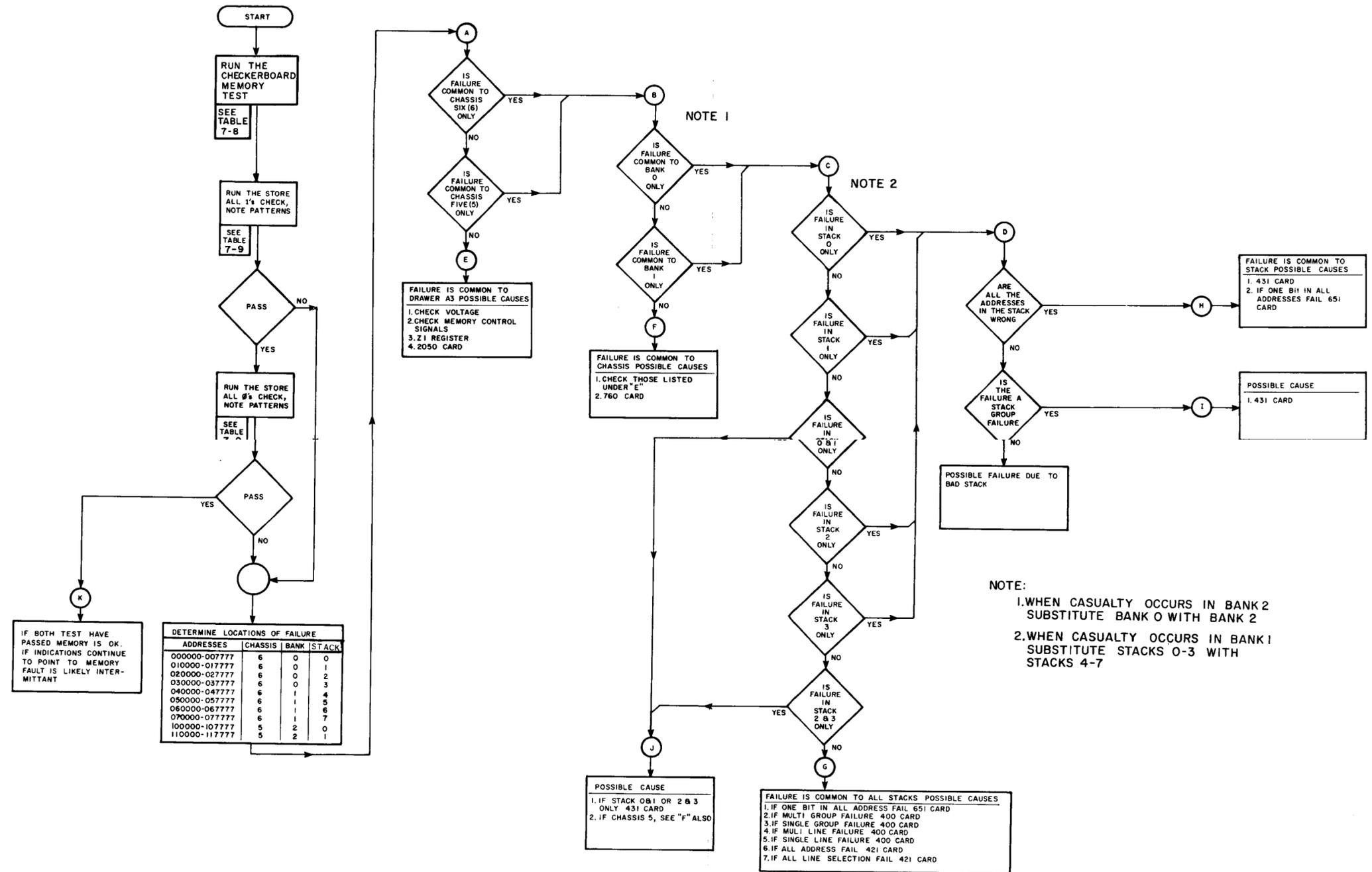
Figure 7-13. Memory Test Flow Chart
