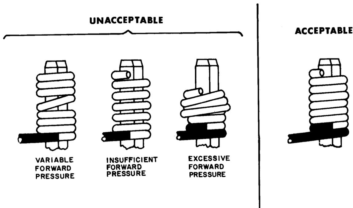
Figure 7-7. Wire-Wrap Connections
