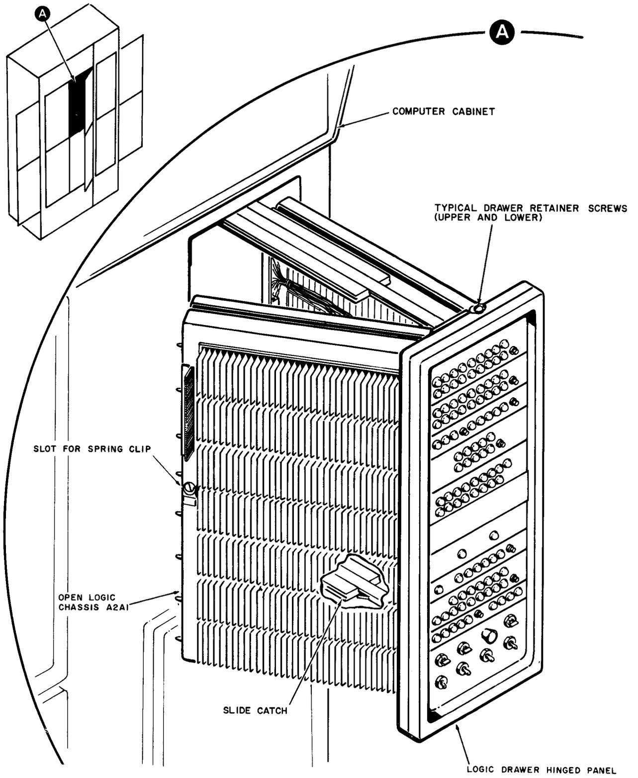
Figure 7-10. Extended Logic Drawer A2
