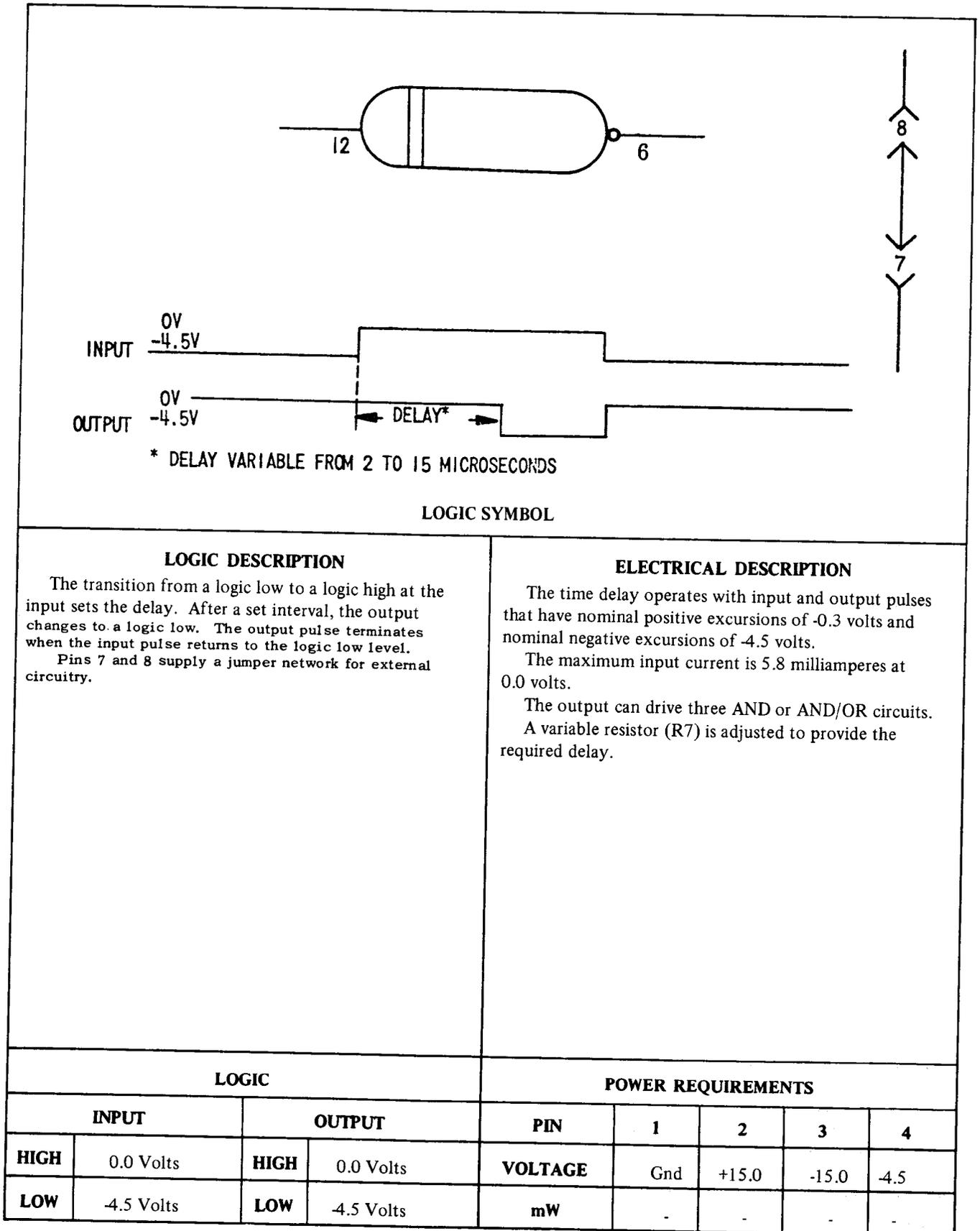
Figure 7-42. Time Delay - 2 to 15 usec, Card Type 7003480
