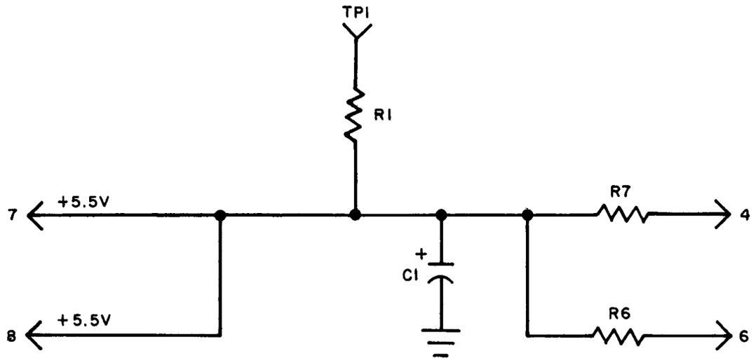
Figure 7-81. Capacitor Assembly Module 7500671, Schematic Diagram
