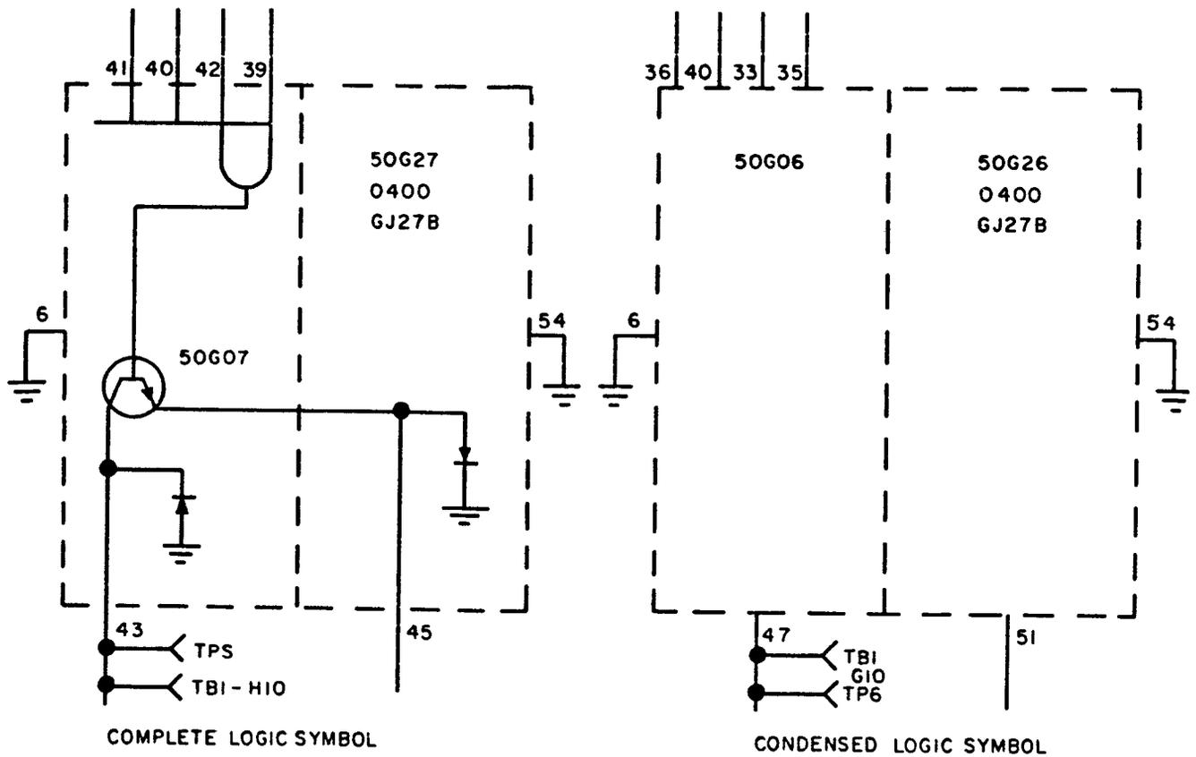
Figure 7-71. Logic Symbol of One Circuit on 7500400 Module
