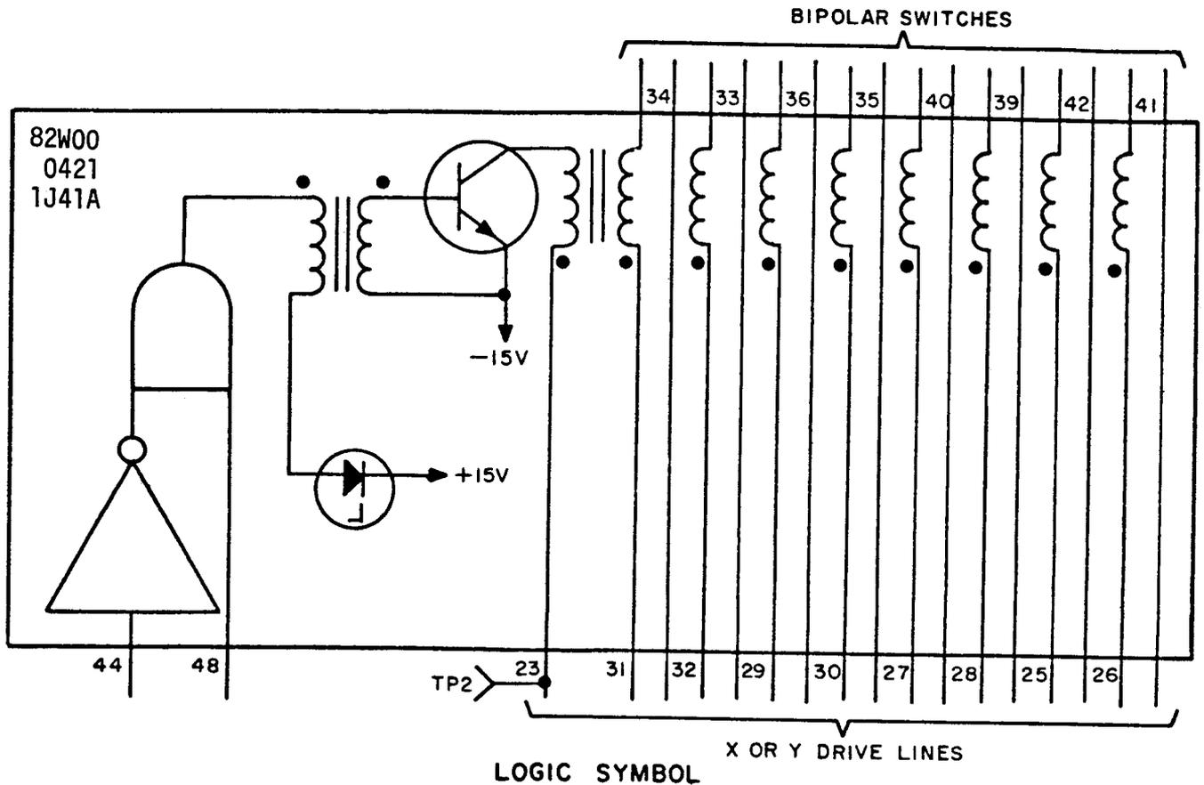
Figure 7-74. Logic Symbol of One Diverter Driver Module 7500421
