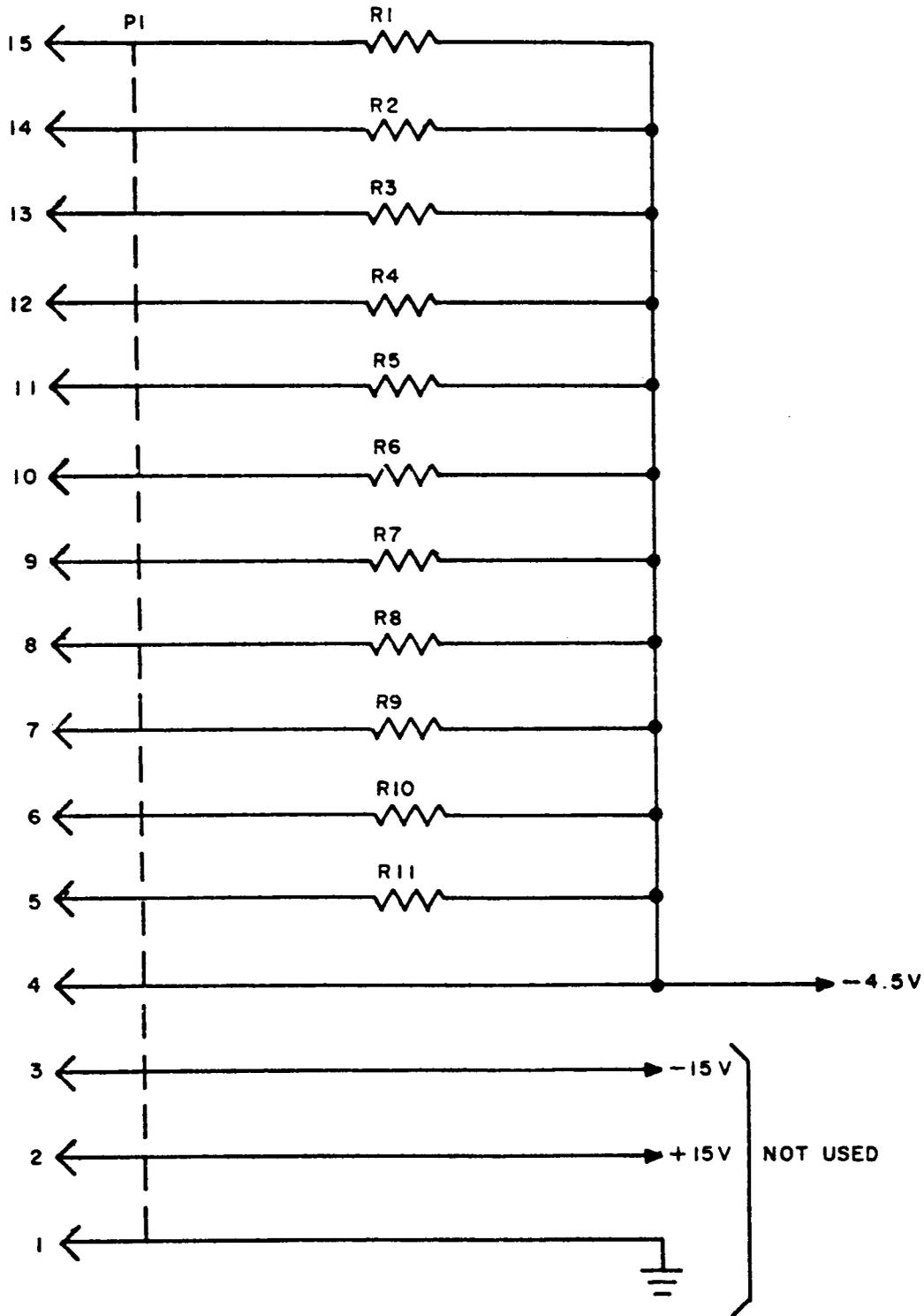
Figure 7-59. Resistor Assembly, Module 7109000 Schematic Diagram
