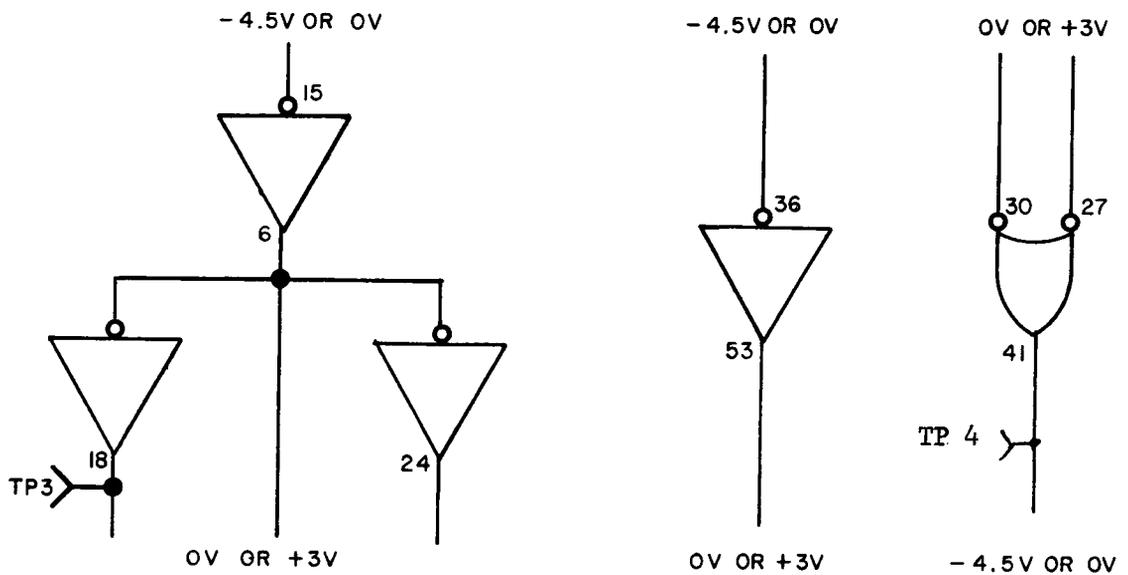
Figure 7-82. Logic Symbol of Level Changer Amplifier, Module 7500761
