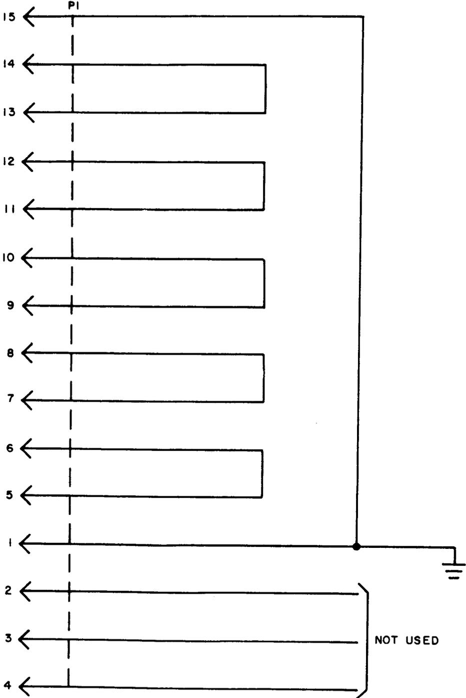
Figure 7-58. Jumper Switch Selector, Module 7104010 Schematic Diagram
