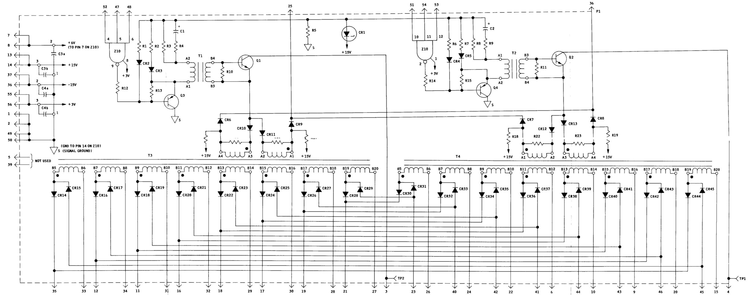
Figure 7-77. Module 7500431 Schematic Diagram
