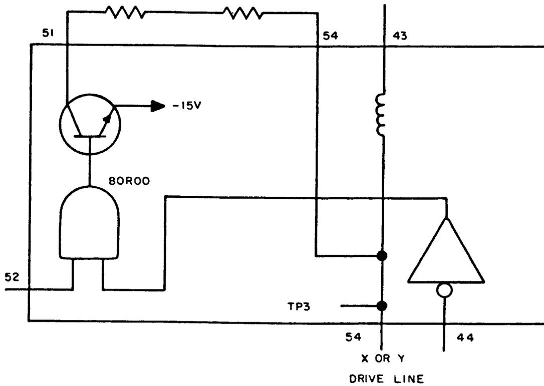
Figure 7-73. Logic Symbol of Read/Write Diverter on Module 7500421
