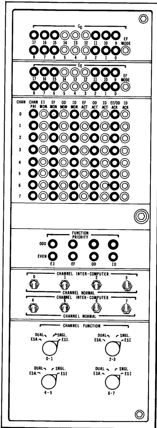
Figure 7-1. Maintenance Controls and Indicators-I/O Panel (A1 or A8)
