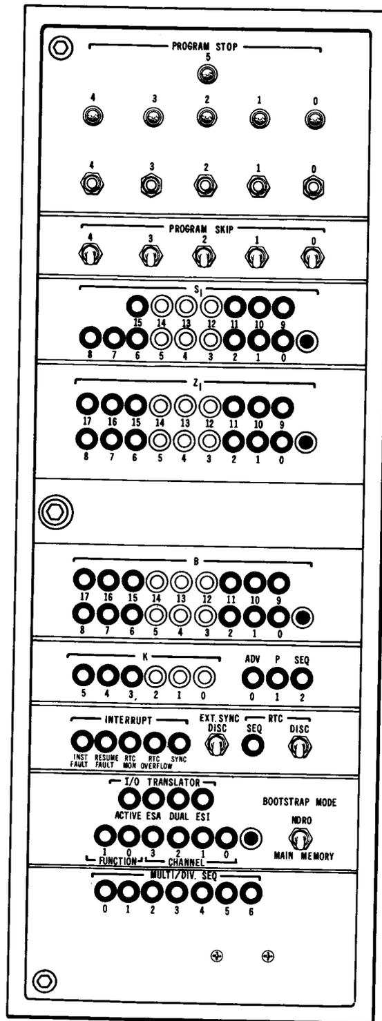
Figure 7-3. Maintenance Controls and Indicators - Control Panel 2 (A4)
