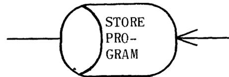
2) Processing Symbols. The specialized processing symbols represent the processing function, and, in addition, identify the specific type of operation to be performed on the data.
