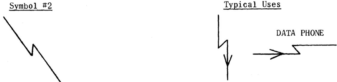
g. Flow Lines. Vertical or horizontal lines between symbols to show the flow of data or control. Arrowheads shall be used for other than top-to-bottom or left-to-right flow, and they may be used on any line for clarity.
