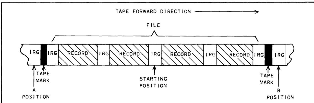
Figure 11. Magnetic Tape Unit – Tape File
