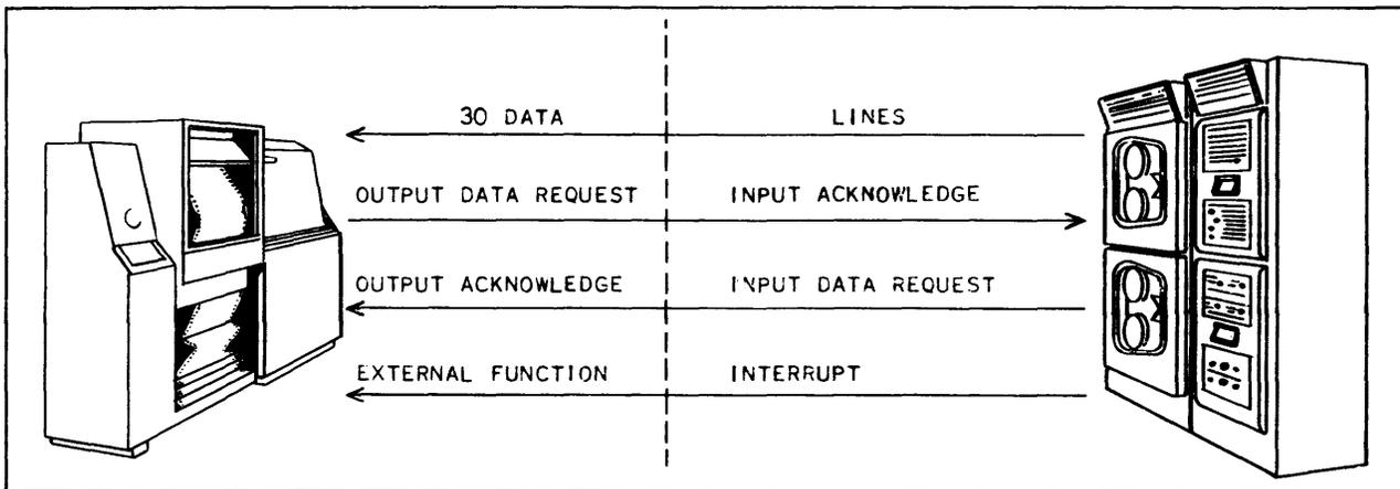
Figure 12. Magnetic Tape – Printer Interface
