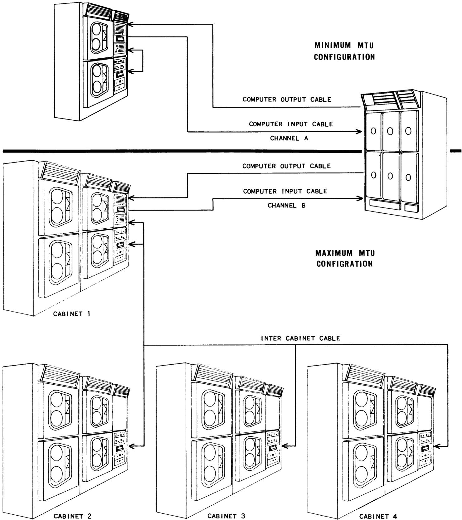
Figure 2. Magnetic Tape Unit and Computer Configurations
