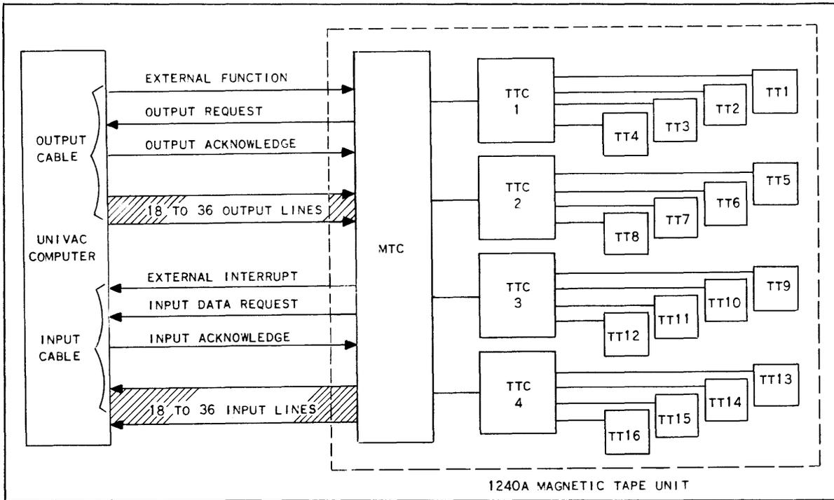
Figure 4. Magnetic Tape Unit - Computer Interface
