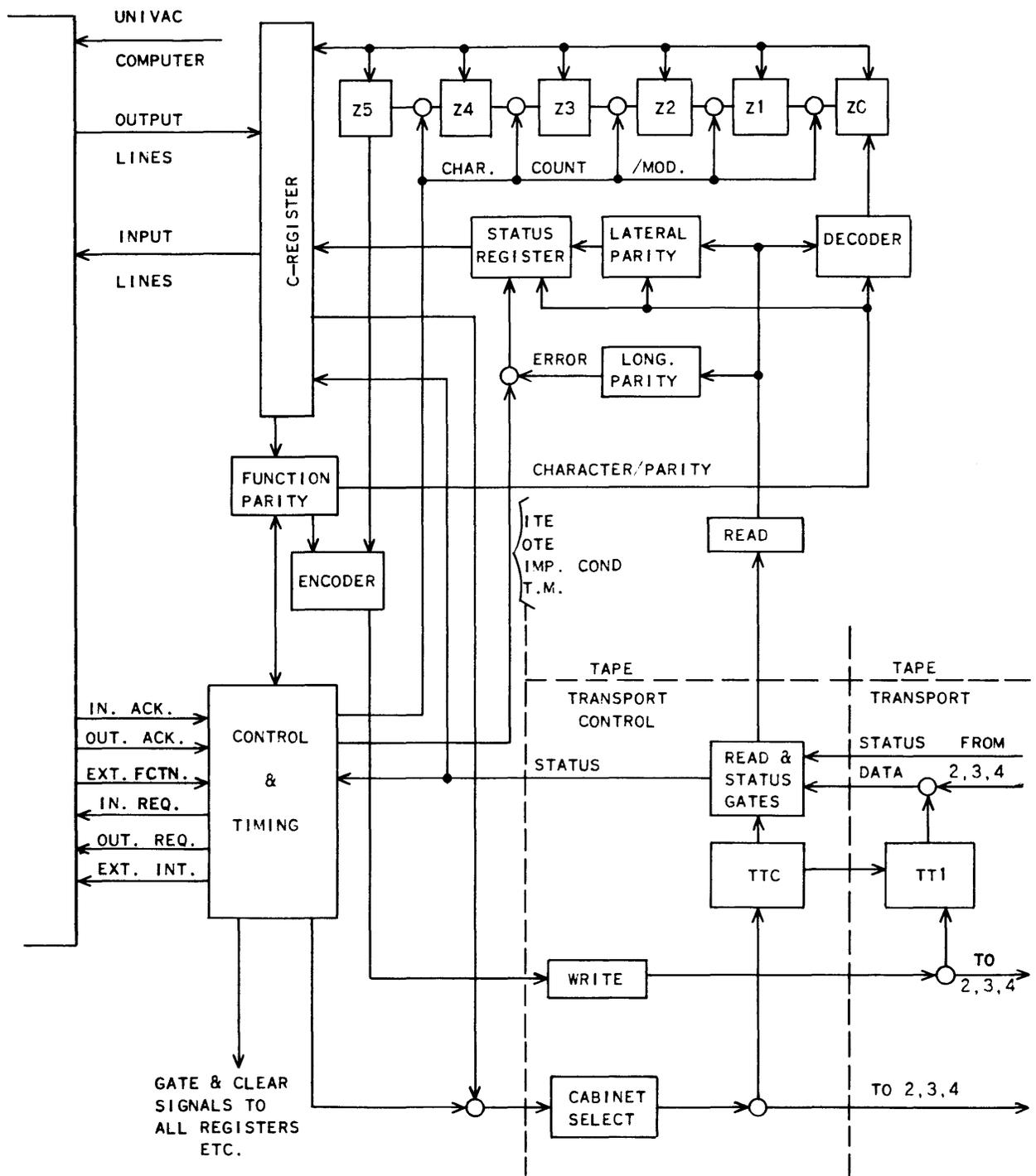
Figure 3. Functional Block Diagram 1240 Magnetic Tape Unit
