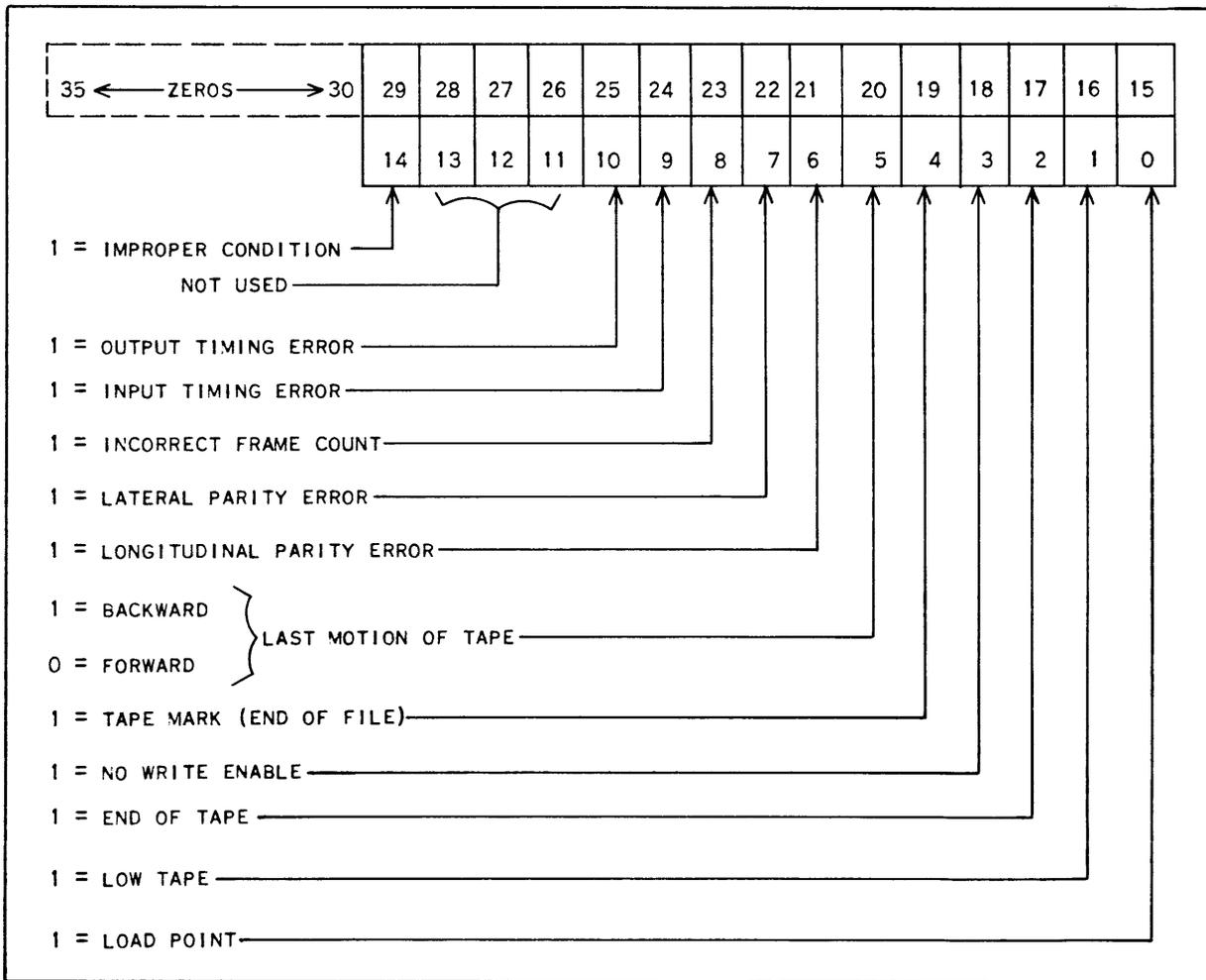
Figure 8. Magnetic Tape Unit - Status Word Format
