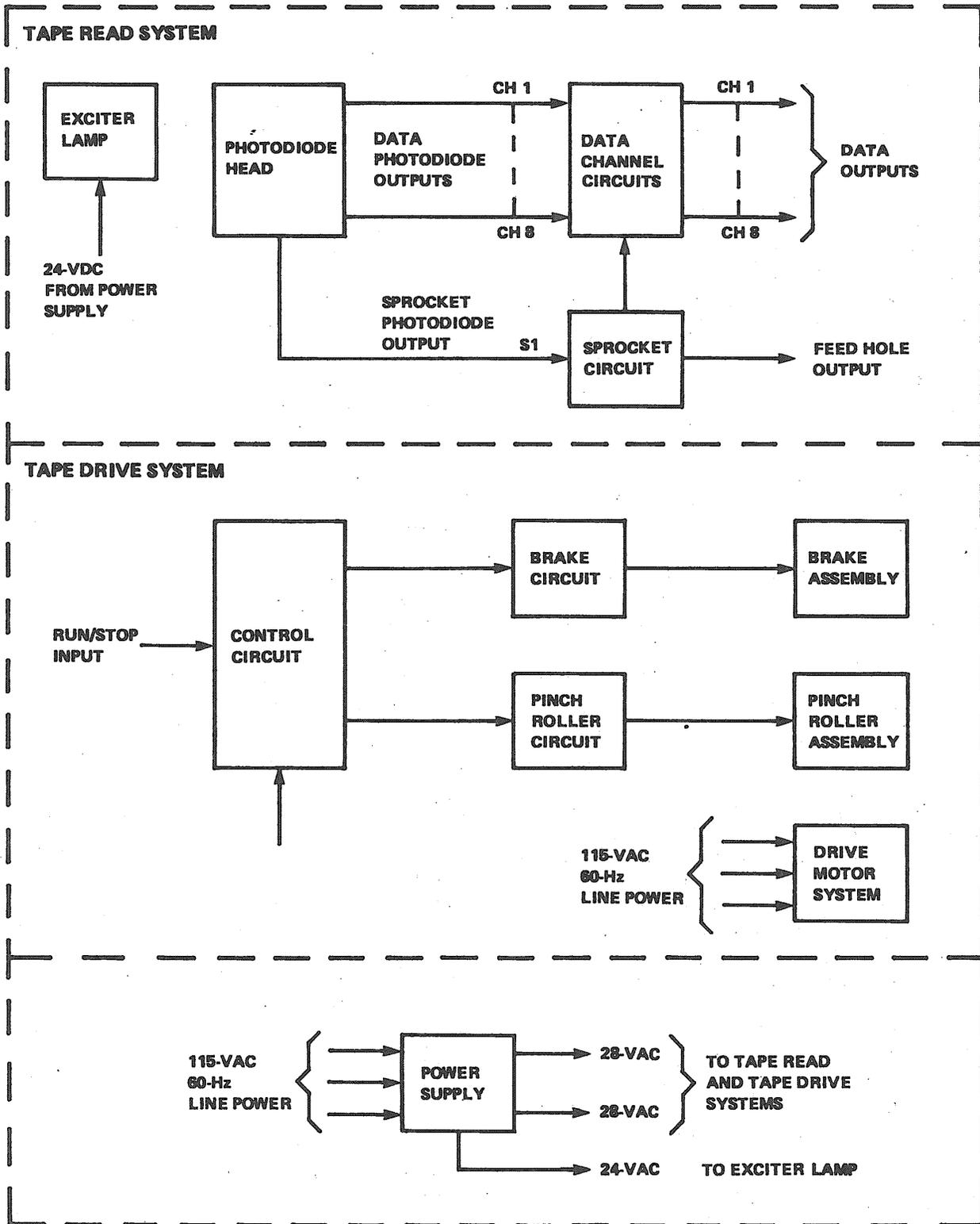
Figure 3-7. Paper Tape Reader Block Diagram.
