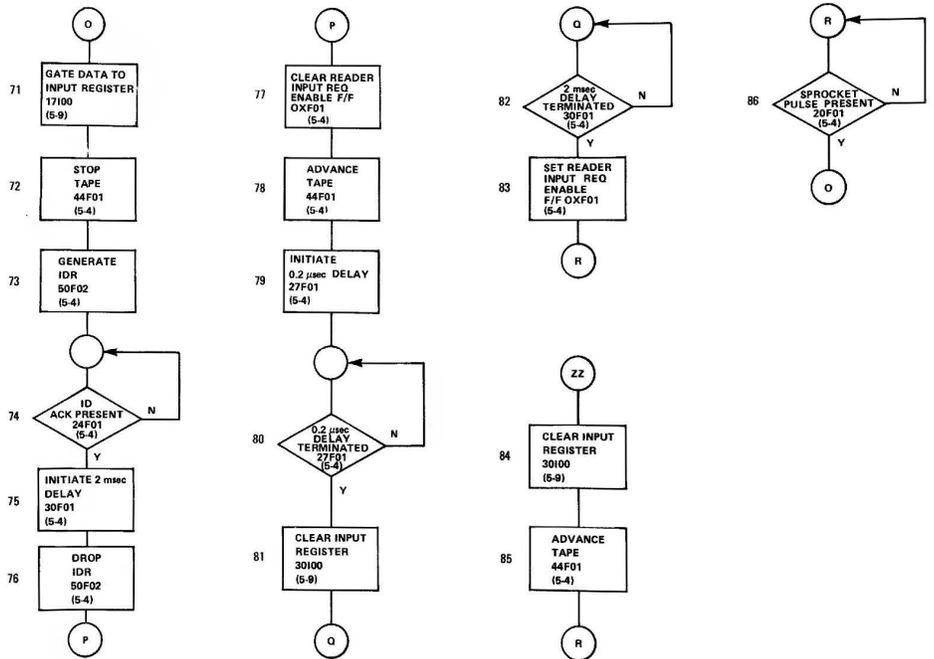
Figure 3-50. I/O Console Operational Sequence Flow Diagram (Sheet 4 of 4).
