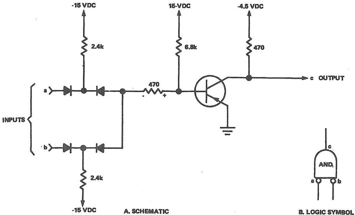
Figure 3-13. Low Input, High Output AND Gate.
