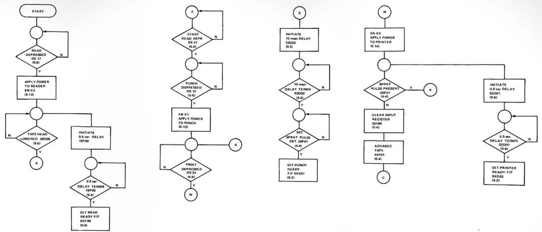
Figure 3-54. Off-Line Reader-Punch-Printer, Operational Flow Sequence Diagram (Sheet 2 of 2).
