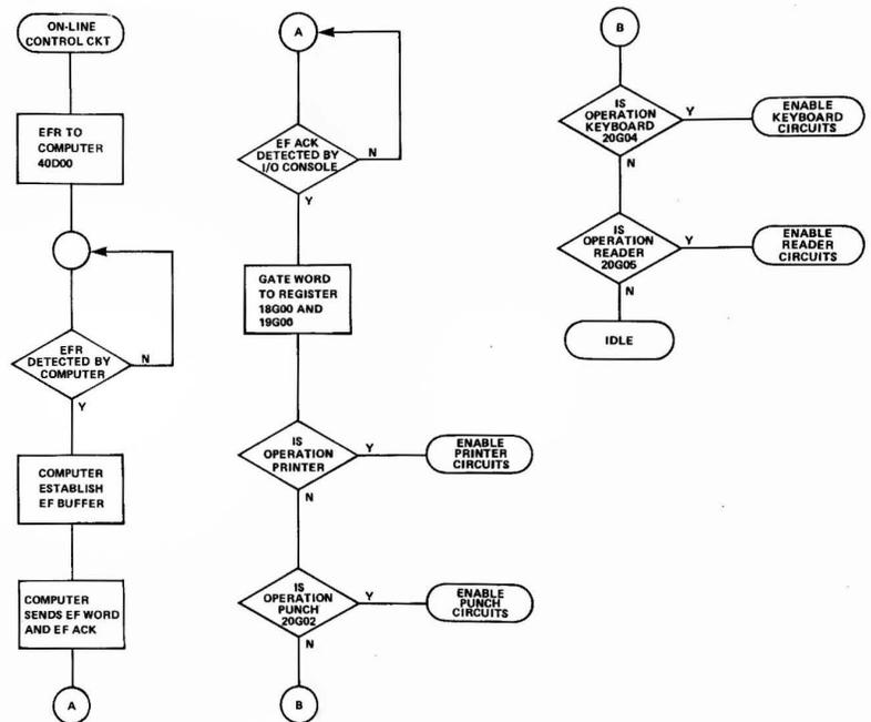
Figure 3-49. On-Line Control Circuits, Operational Flow Sequence Diagram.
