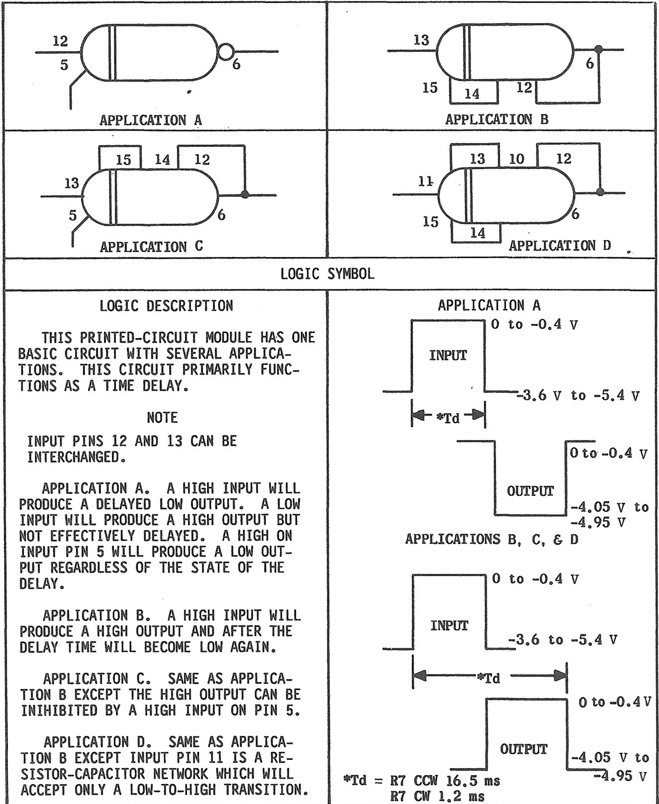
Figure 3-47. Time Delay, 1.5 to 15 msec, Card Type 7003580.
