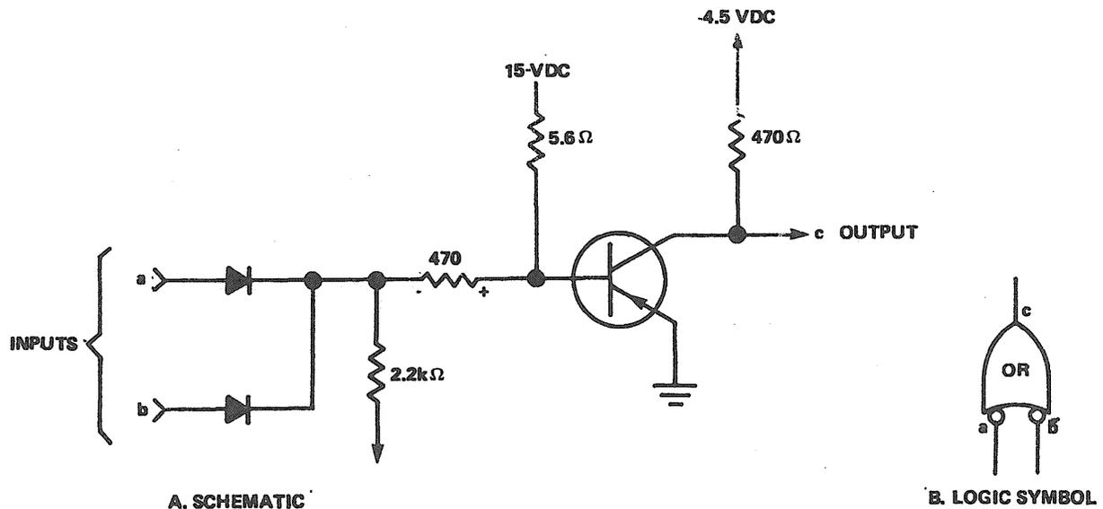
Figure 3-15. Low Input, High Output OR Gate.
