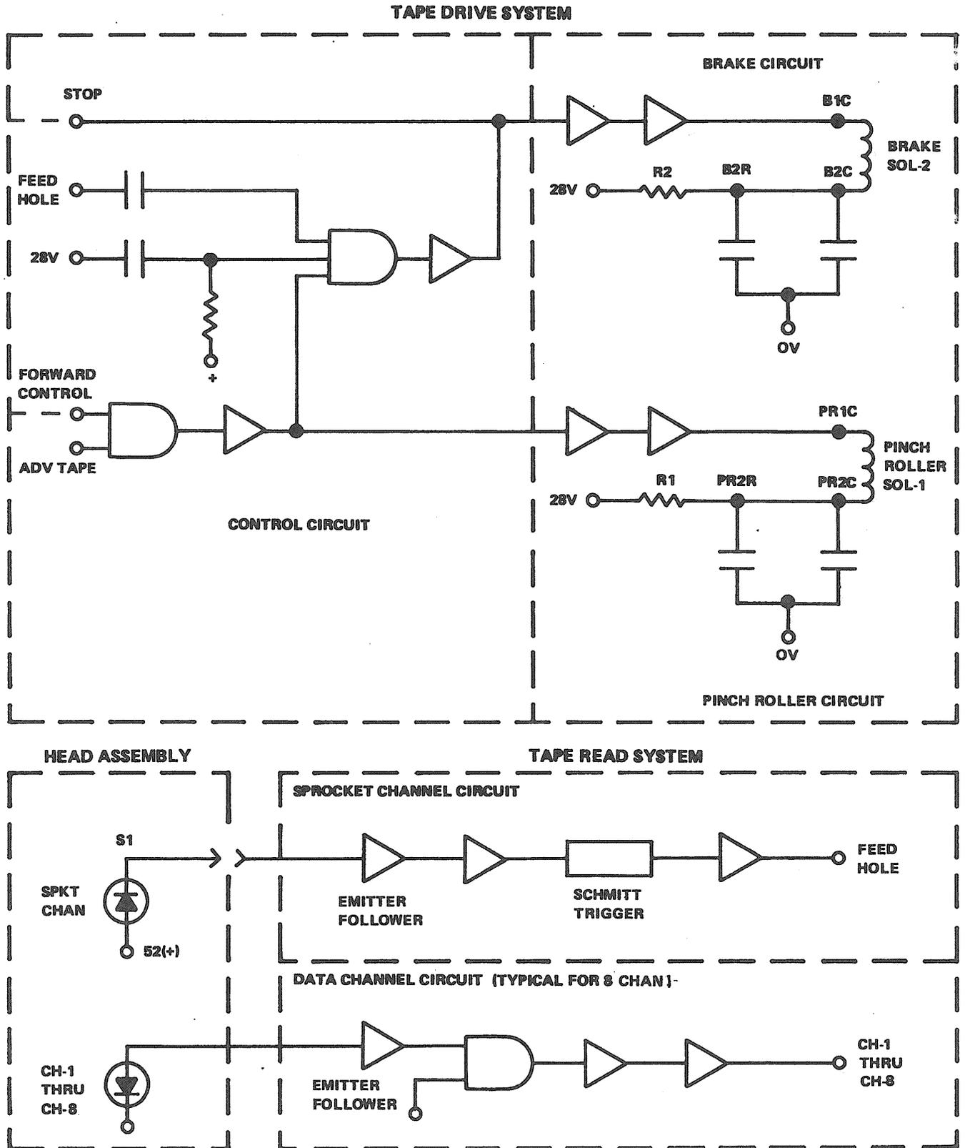
Figure 3-8. Paper Tape Reader Logic Diagram.
