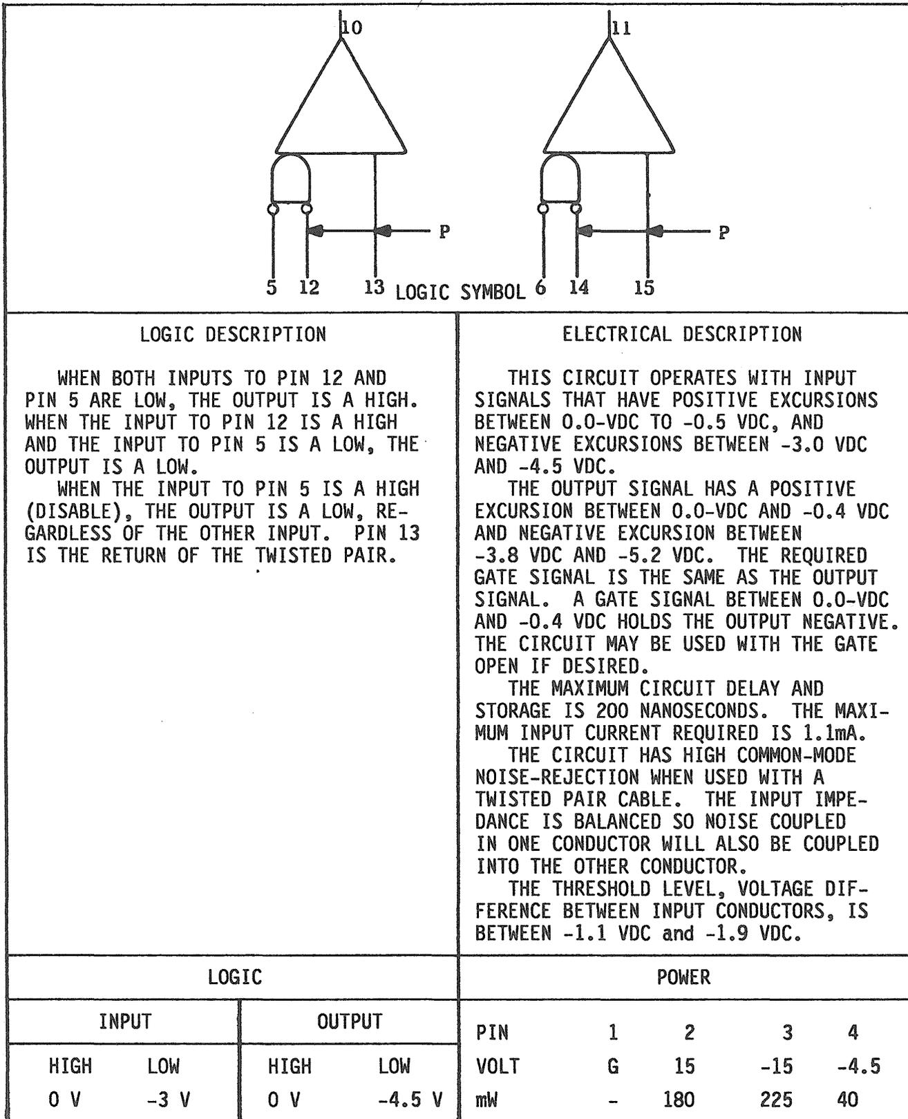
Figure 3-32. Amplifier, Differential, Card Type 7002321.
