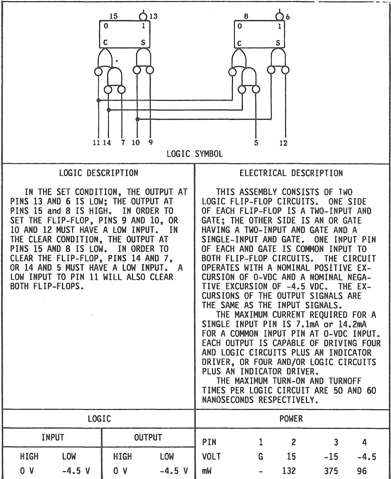
Figure 3-41. Flip-Flop, Card Type 7002930.
