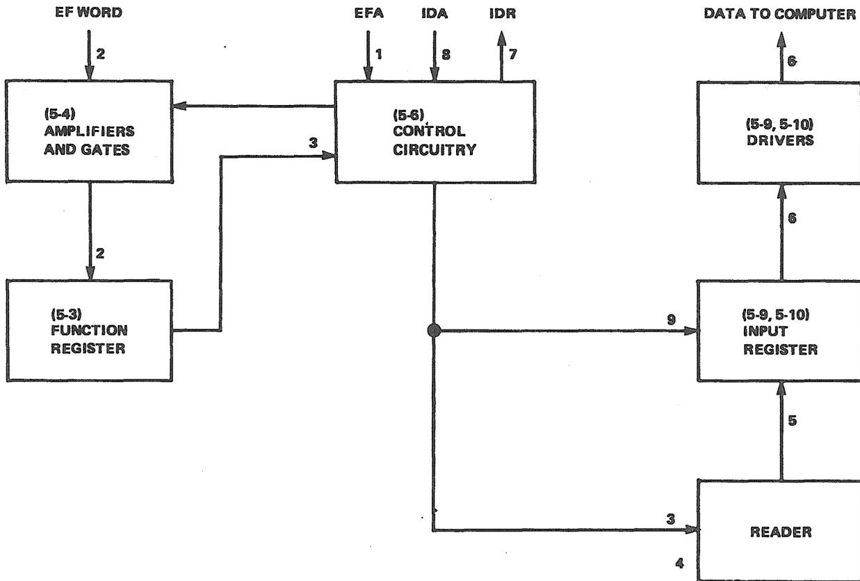
Figure 3-4. Paper Tape Reader Operation.
