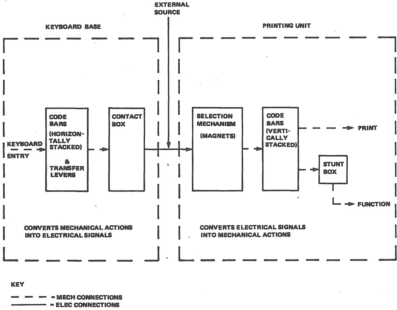
Figure 3-6. Block Diagram of Keyboard/Printer Operation.
