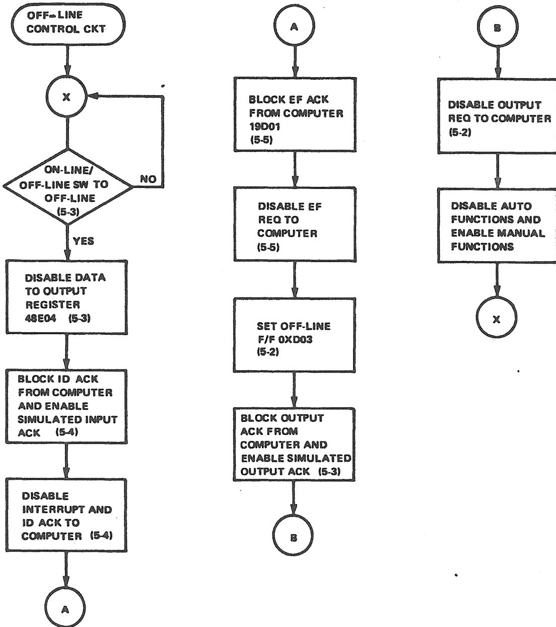
Figure 3-53. OFF-LINE Control Circuits, Operational Sequence Flow Diagram.
