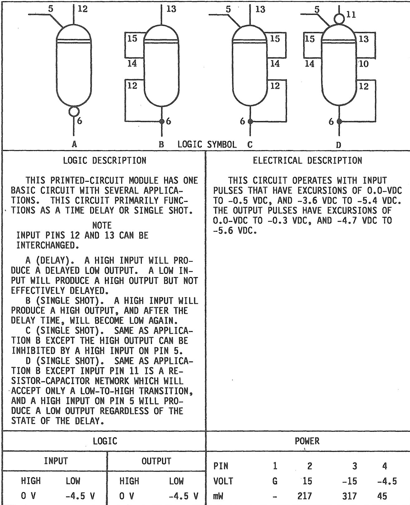
Figure 3-46. Time Delay, 1.2 to 16.5 msec, Card Type 7003480.
