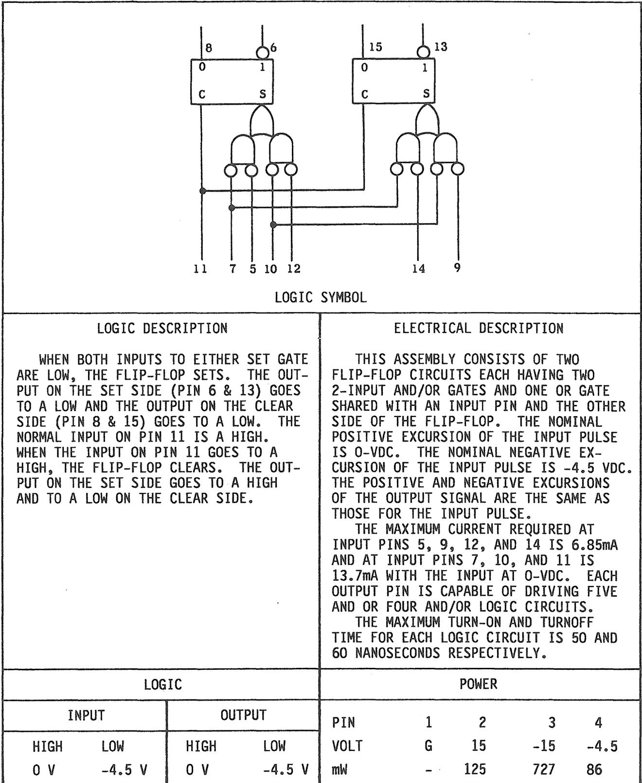
Figure 3-39. Flip-Flop, Card Type 7002900.
