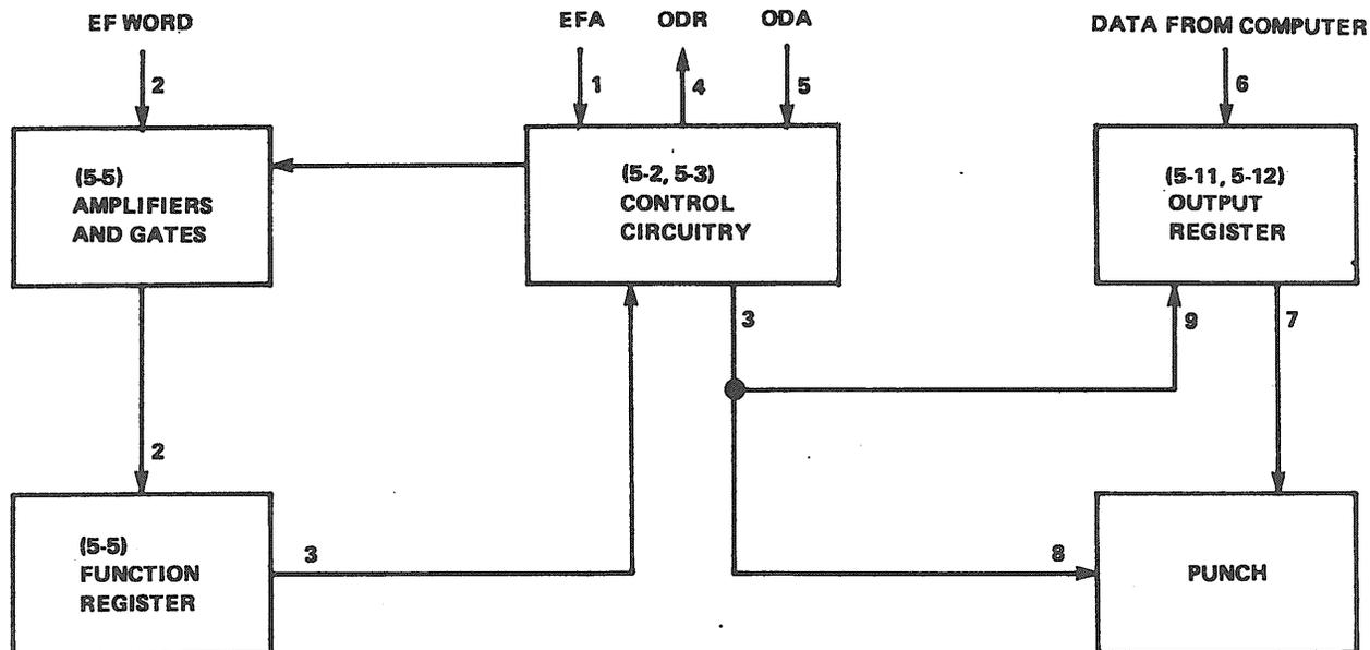
Figure 3-5. Paper Tape Punch Operation.
