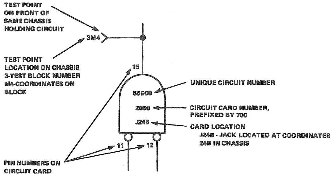
Figure 3-19. Logic Gate Notation.
