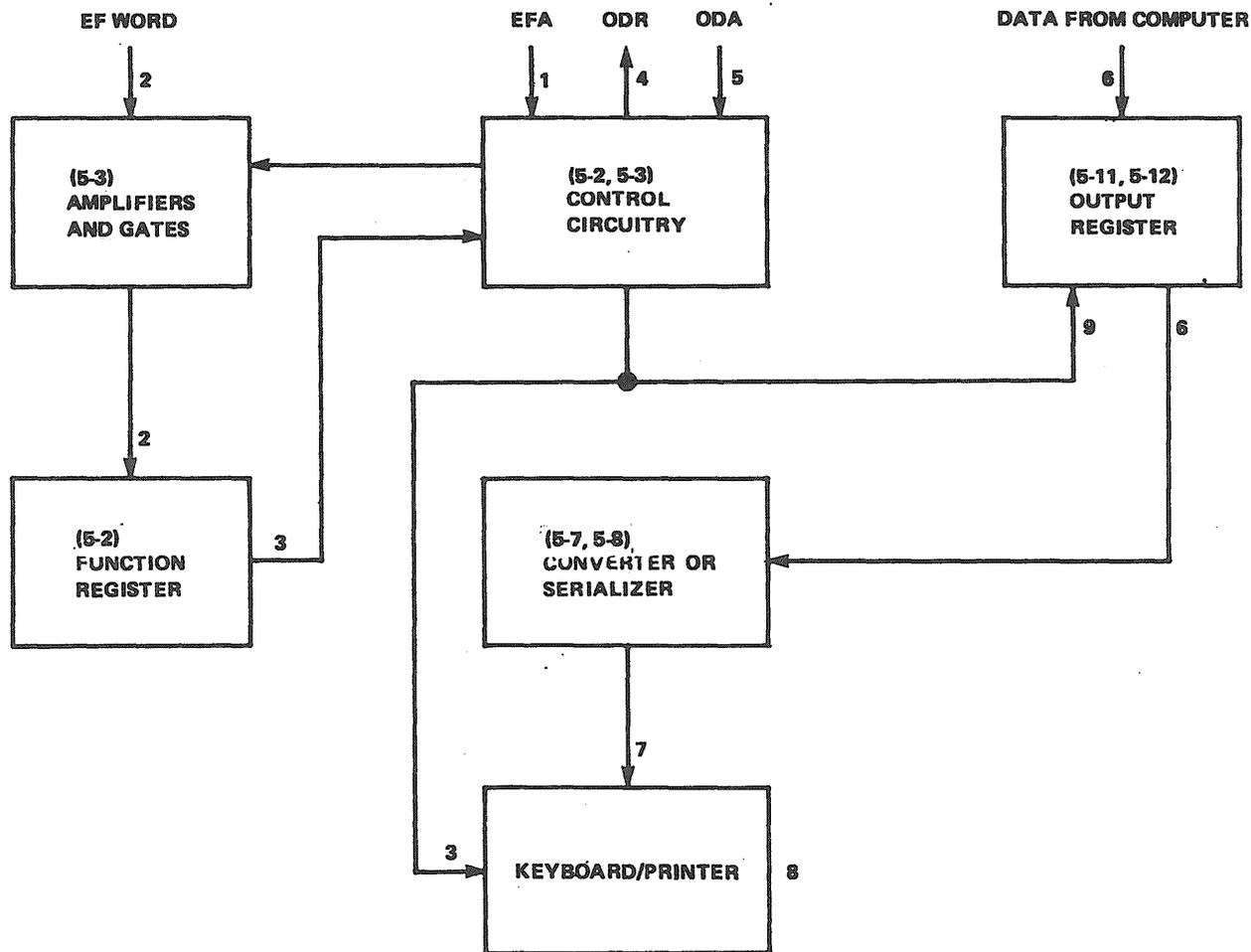
Figure 3-3. Printer Operation.
