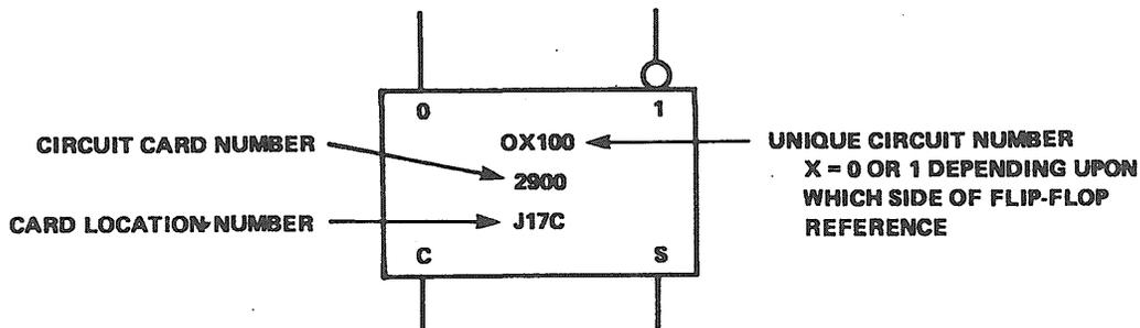
Figure 3-18. Flip-Flop Notation.
