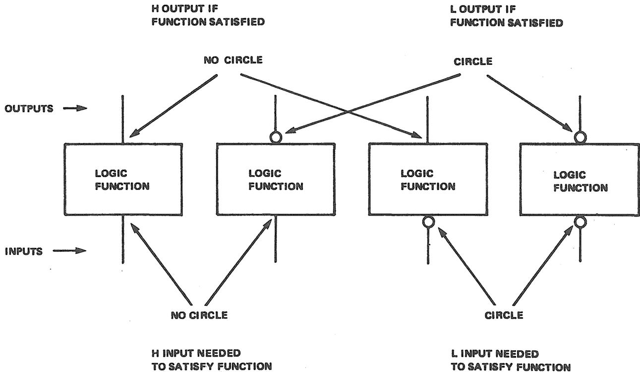
Figure 3-11. Illustration of Circle Level Notation.
