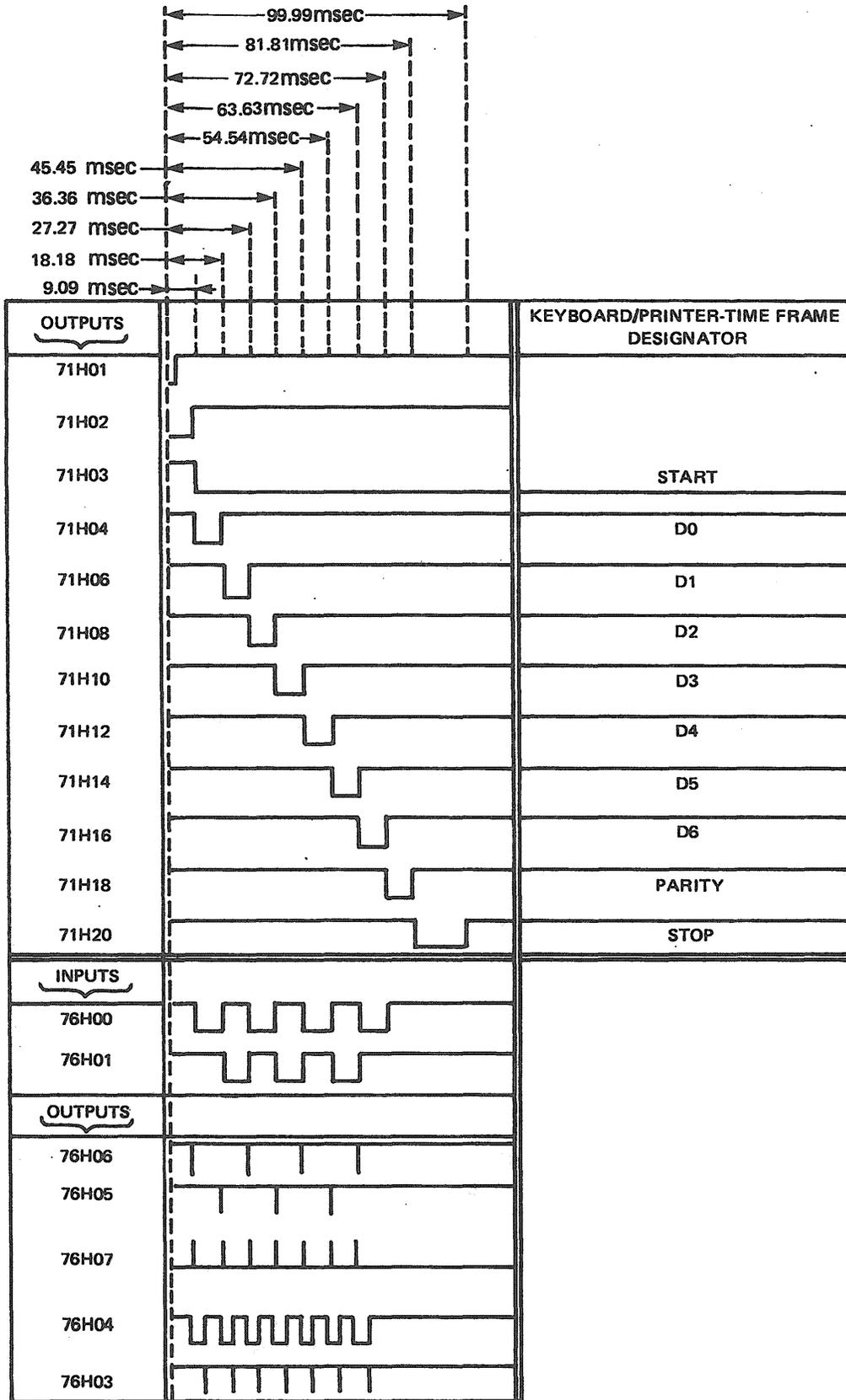
Figure 3-51. Serializer Timing Gates and Pulses.
