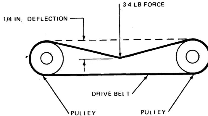
Figure 6-17. Drive Belt Tension Adjustment.
