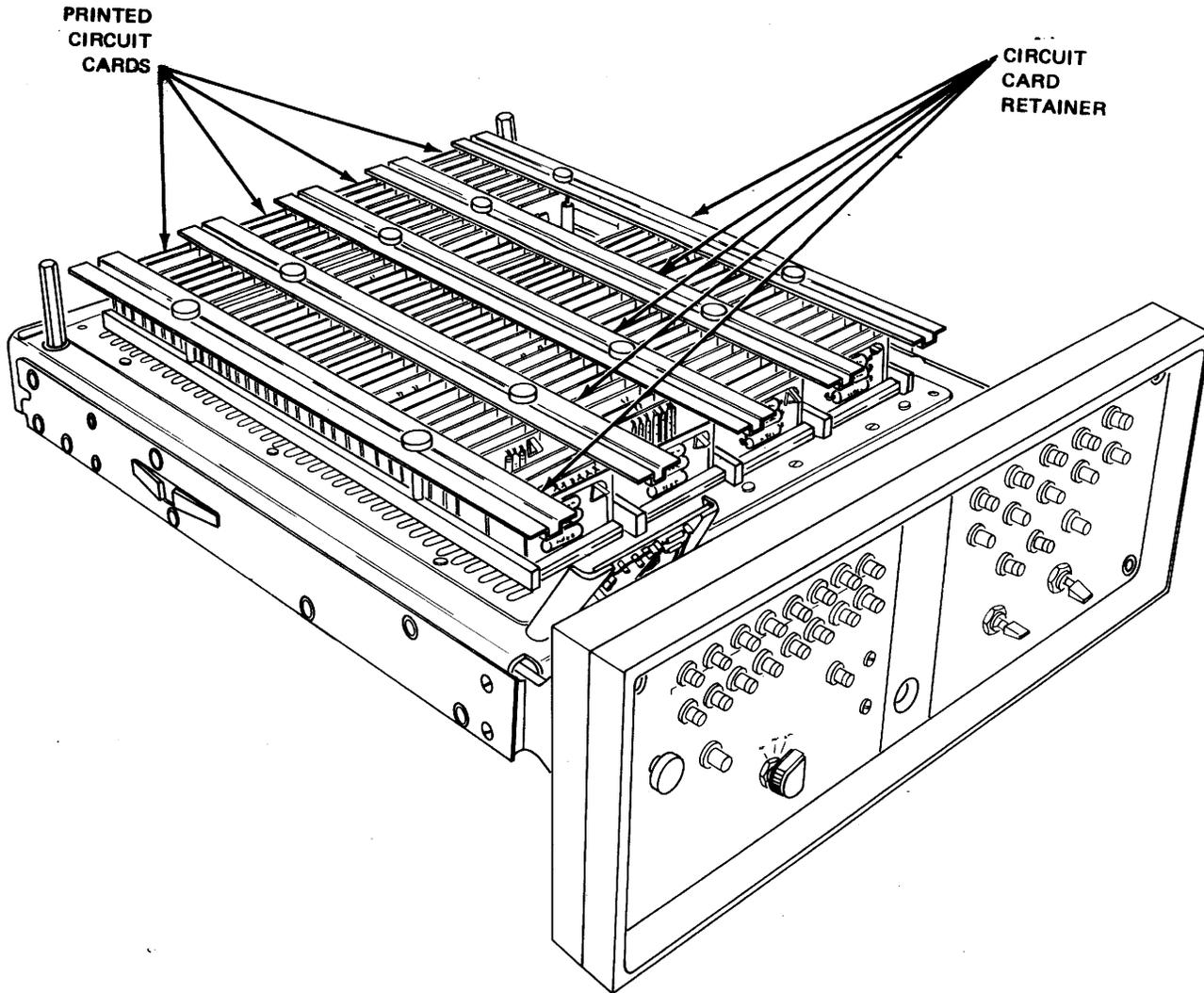
Figure 6-36. Logic Chassis and Printed Card Location.
