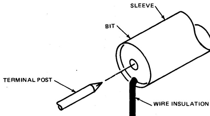
(B) POSITIONING OF GUN, WIRE INSULATION AND TERMINAL POST
