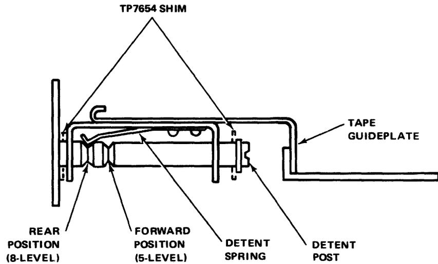
Figure 6-65. Tape Guide for LHA-1 Class Ships.
