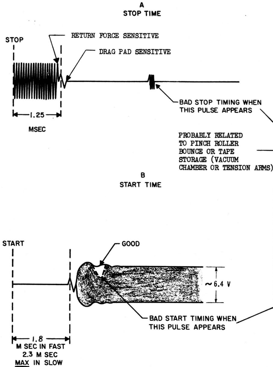
Figure 5. Transport Start-Stop Check Waveforms
