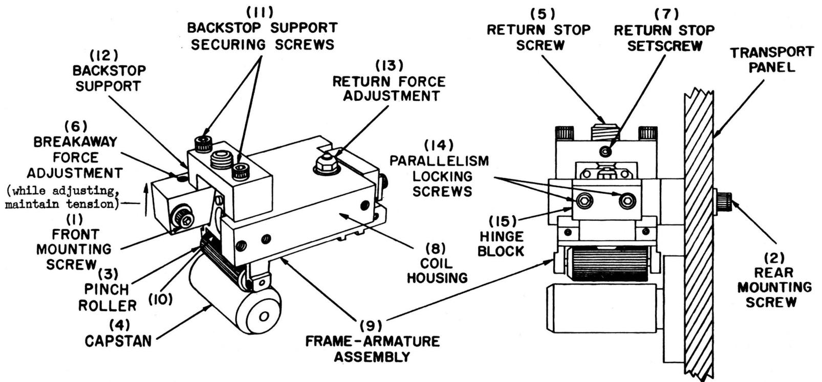
Figure 1. Solenoid Adjustments
