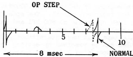
The pulses will be solid at about 8msec for the tape marks which were written in normal mode. For the tape marks written in "OP-STEP" mode, the pulses will bounce back about 0.5 millisecc if the inter-record gap is correct. When the inter record gap is correct the START time is also correct.
