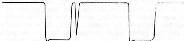
The problem results from cross talk in the chassis wiring and is solved by shortening and re-routing the clock phase wires in the chassis. To check for the possibility of runt pulses, monitor the clock drivers in chassis A12A1 and A12A2, referencing figures 8-92 and 8-93 of PX 3334 volume II.
