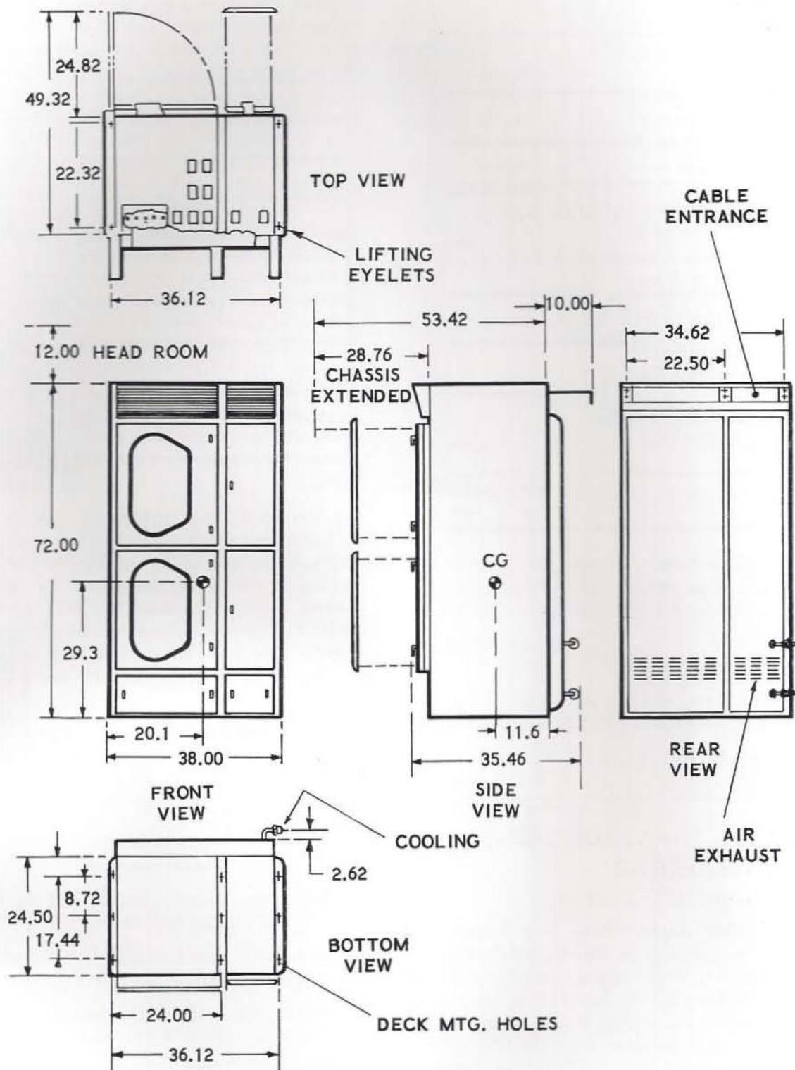
Figure 3. Dimensional Data for 1540 Basic Magnetic Tape Unit (Air-Cooled)
