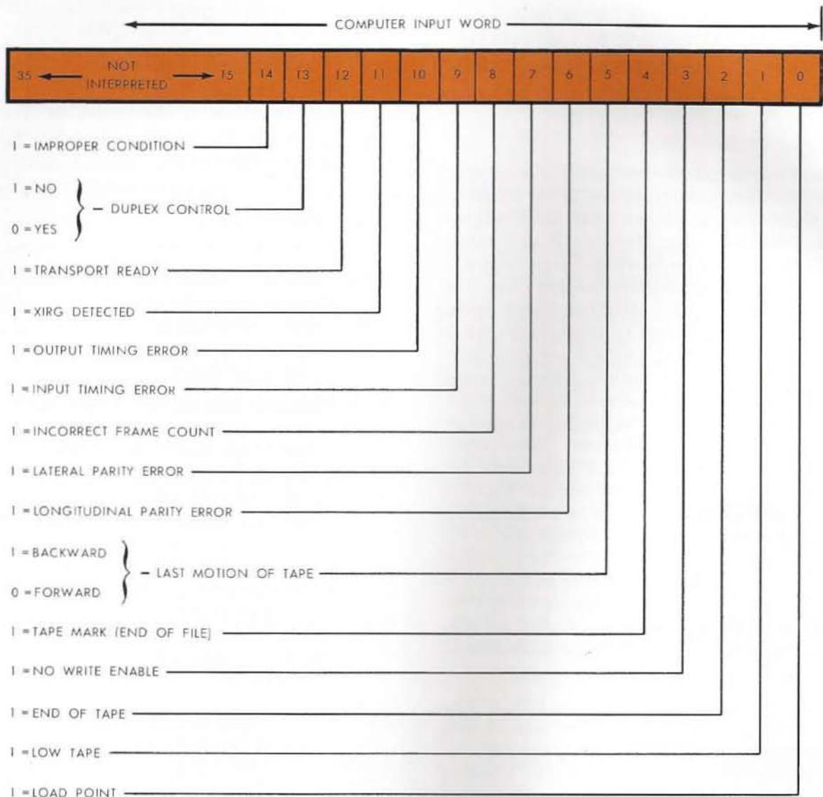
Figure 7. Magnetic Tape Unit – Status Word Format
