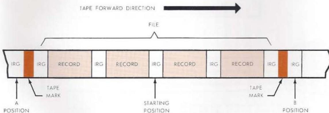
Figure 11. Magnetic Tape Unit – Tape File
