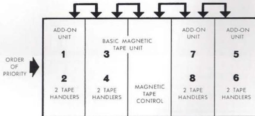
Figure 5. Type 1540 Magnetic Tape System (Maximum Configuration)
