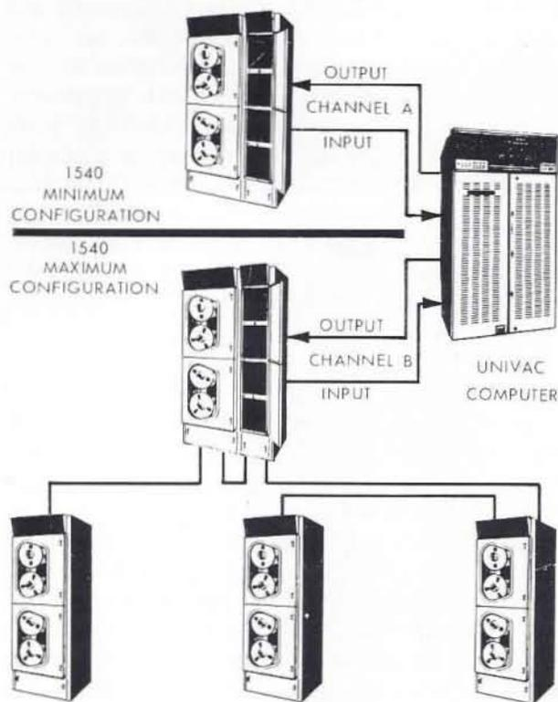
Figure 2. UNIVAC 1540 Magnetic Tape Units and Computer Configuration
