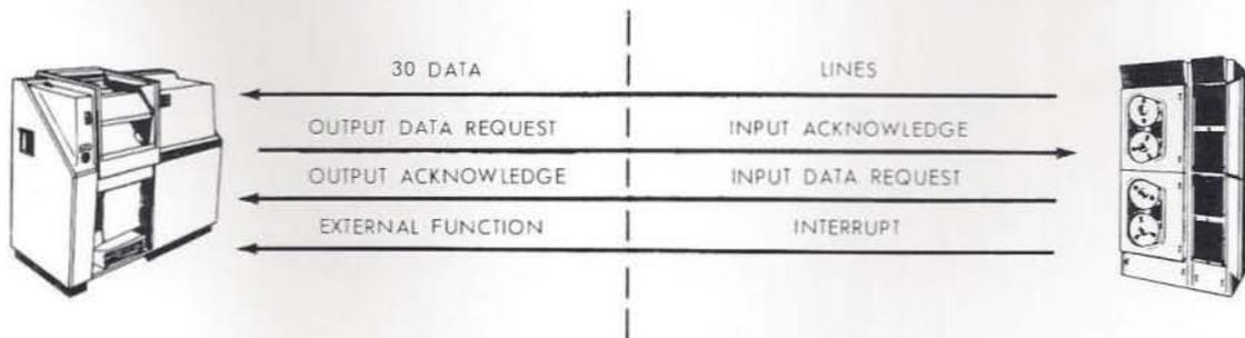
Figure 13. Magnetic Tape - Printer Interface
