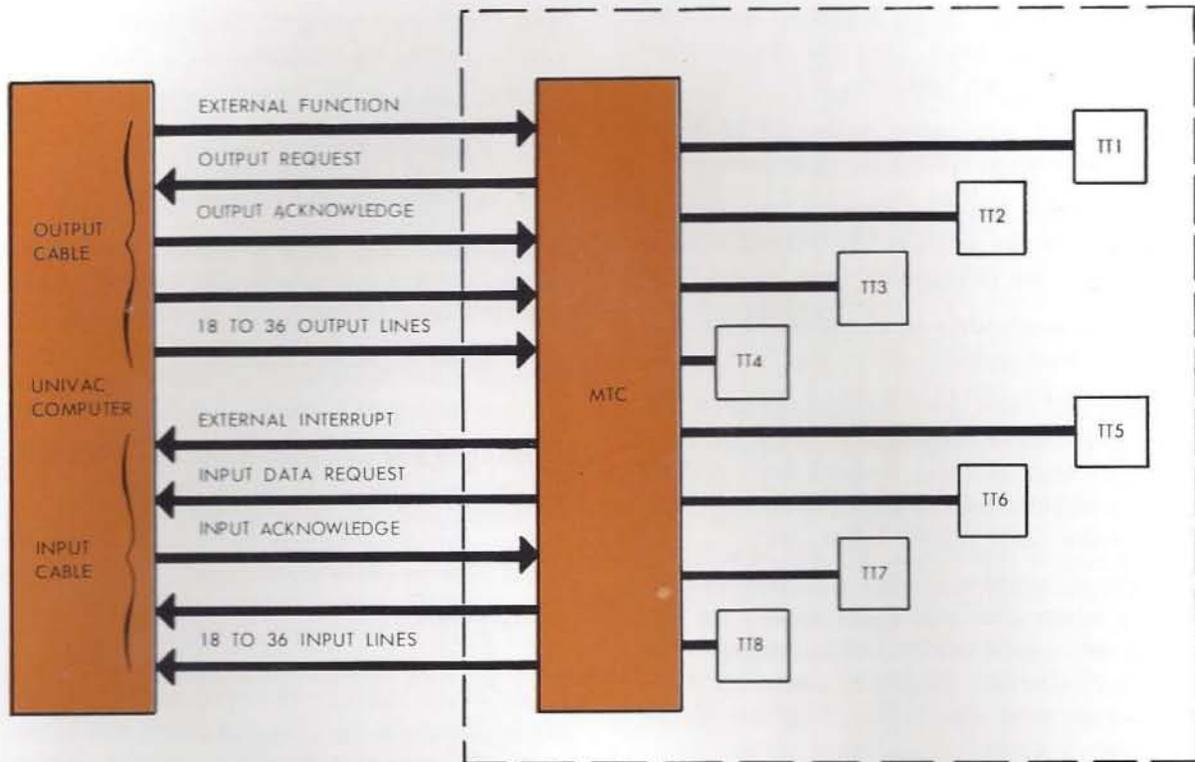
Figure 4. Magnetic Tape Unit - Computer Interface
