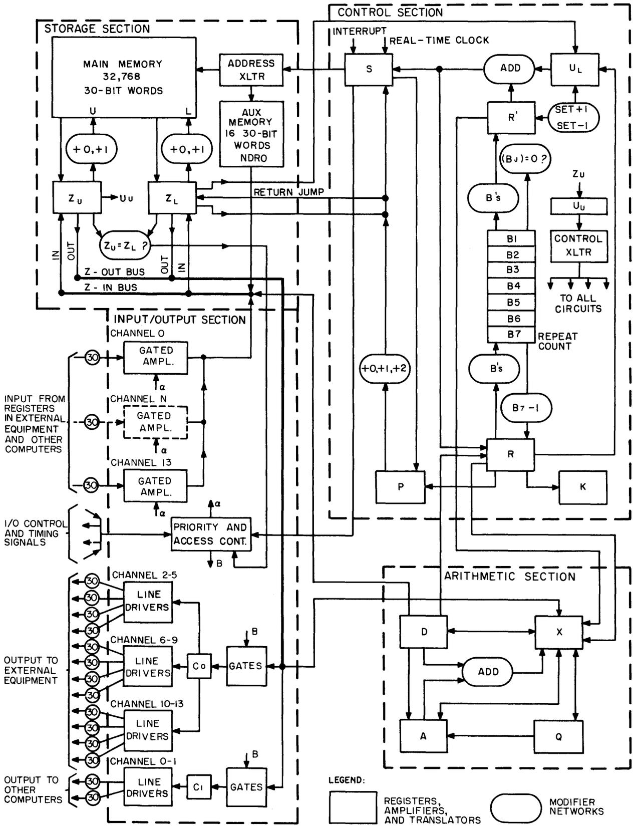
Figure C3-2. Simplified Block Diagram, AN/USQ-20 Unit Computer
