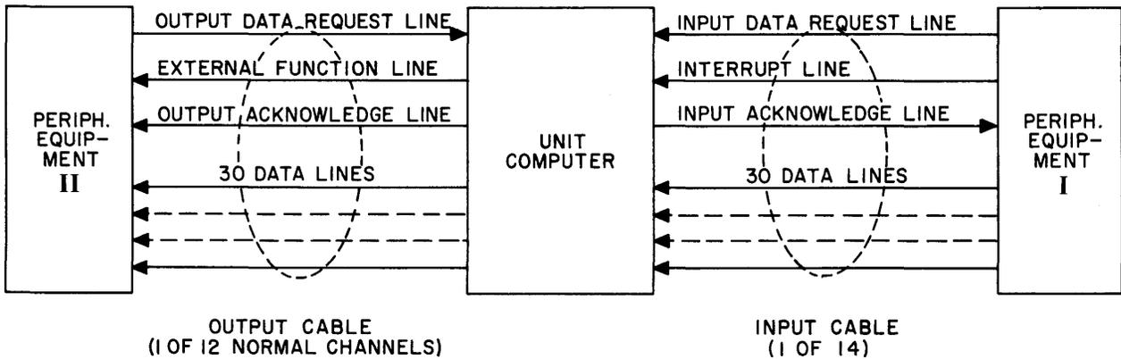
Figure C3-4. Cable Connections
