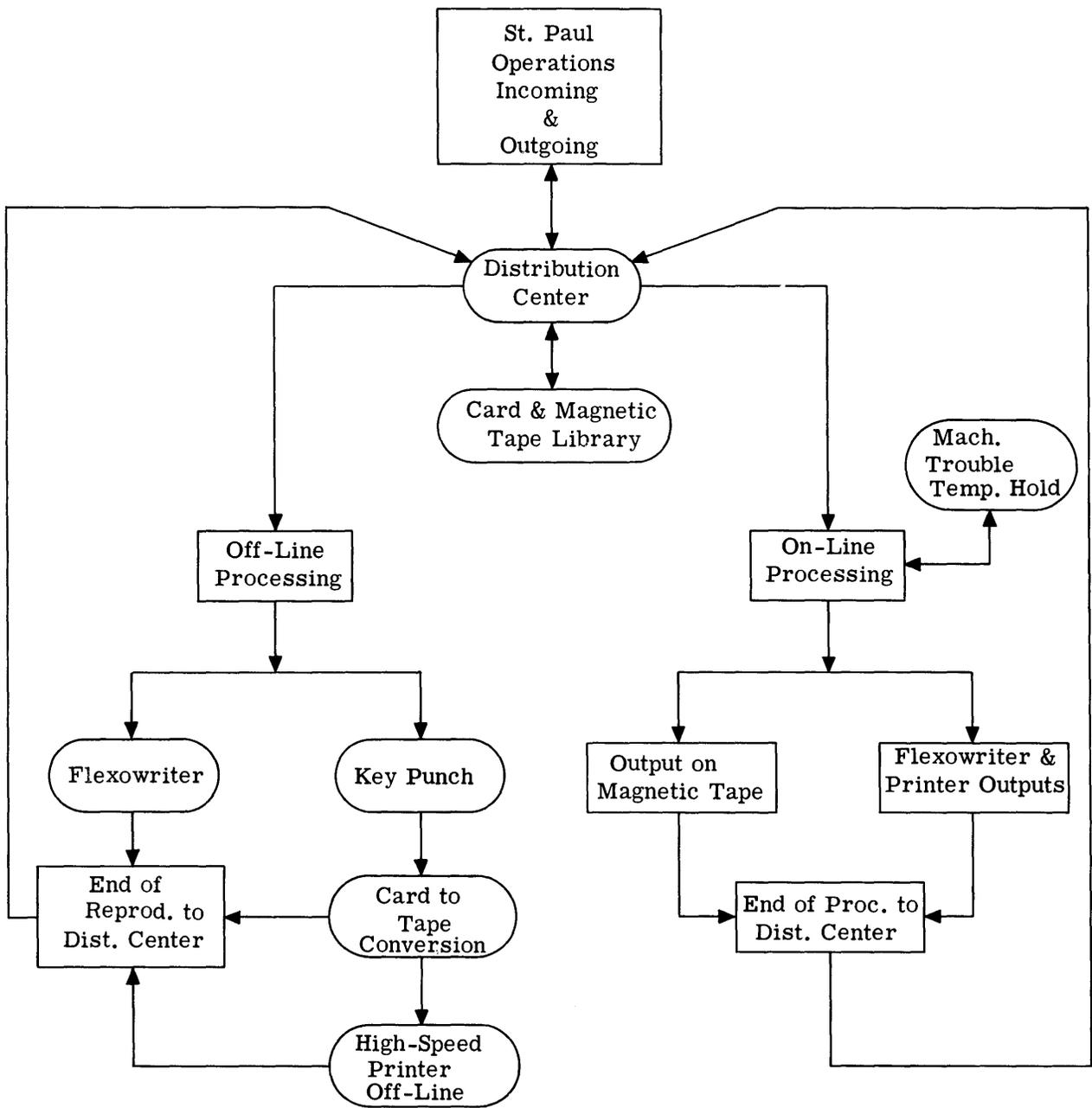
Figure B2-1. Flow of Material - St. Paul Operations Section
