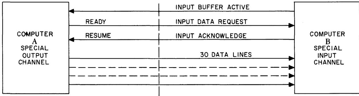
Figure C3-5. Connections from Computer A to Computer B
