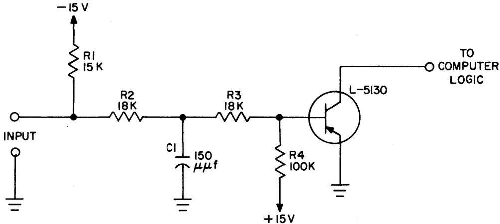
Figure C1-6. Circuit Diagram - Input Amplifier
