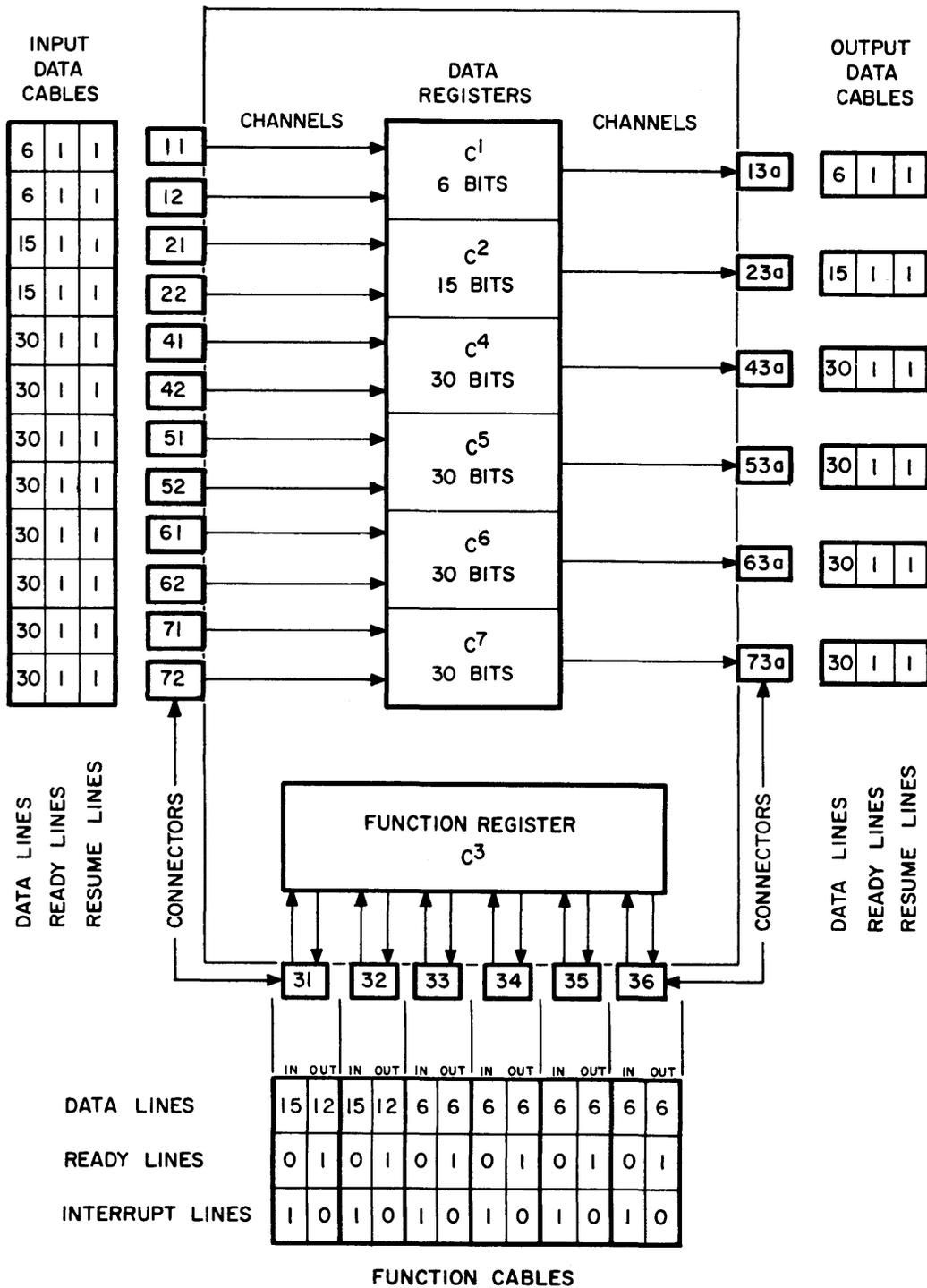
Figure C1-1. Block Diagram - Input/Output Section
