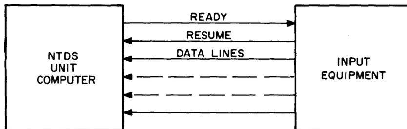
Figure C1-2. Data from Input Equipment to Computer
