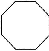
Represents a *stop* in the sequence flow. Any required external notification, associated condition, and/or action should be noted in the octagon when its omission would detract from the clarity of the diagram.
