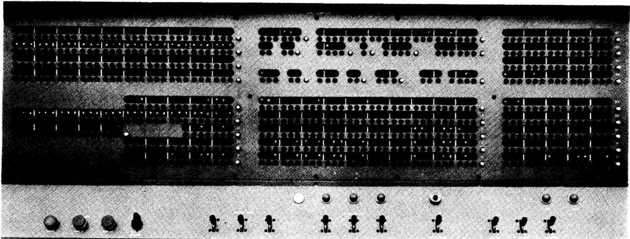
Figure C2-1. Maintenance-Console Panel for Serial 6
