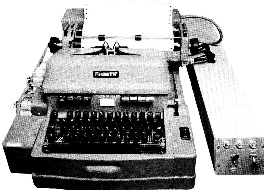
Figure D5-1. Monitoring Typewriter (Flexowriter, Model FL)
