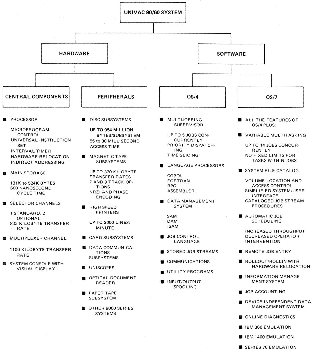
Figure 2-1. Highlights of UNIVAC 90/60 System Hardware and Software
