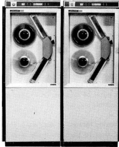
The UNISERVO VI-C Magnetic Tape Subsystem is a low cost magnetic tape subsystem which comprises a control and from two to eight magnetic tape units. The master/slave concept is employed in the logic of the UNISERVO VI-C Magnetic Tape Subsystem. The master unit, having the power supply and control circuitry, governs the functions of up to three slave magnetic tape units. However, all units are treated alike from a programming or operating system viewpoint.
