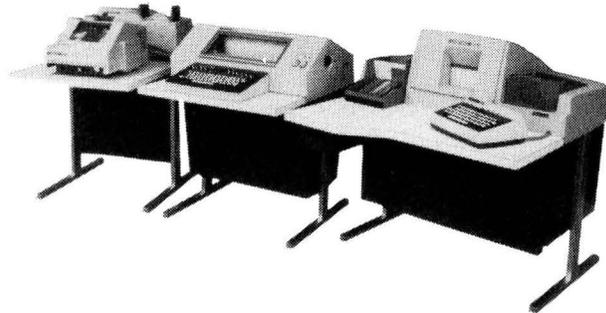
The UNIVAC DCT 1000 Data Communications Terminal is a fully buffered 30-character-per-second incremental printer which can be expanded to include a keyboard, card reader, card punch, paper tape reader/punch, and an auxiliary printer. The DCT 1000 transmits or receives data from a local or remote processor or to a remote DCT 1000 in a conversational or batch mode.
