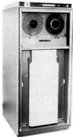
The UNISERVO 16 Magnetic Tape Unit is a higher performance tape unit and can be added to the subsystem individually to a maximum of 16. UNISERVO 16 Magnetic Tape Units are available in 9-track and 7-track models.
