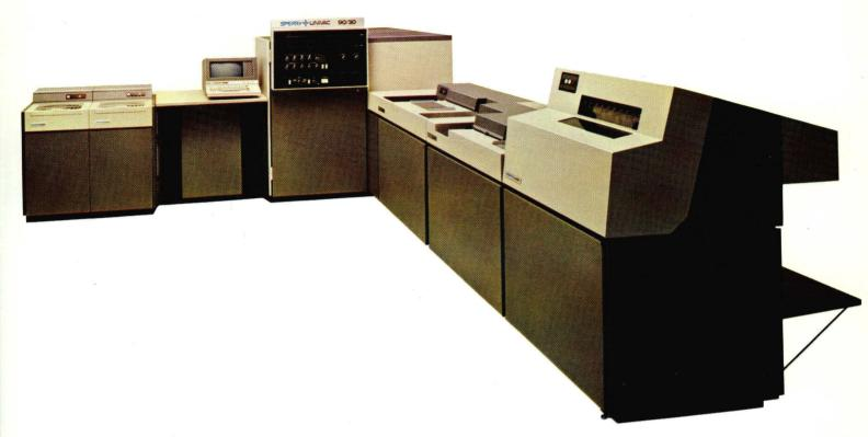
The photo above shows a basic SPERRY UNIVAC™ 90/30 System configuration with central processor, an operator's CRT display console, an Integrated Card Reader (500 CPM), an optional Integrated Card Punch (75-160 CPM), an Integrated Printer (500 LPM) and two Integrated Disc Drives with a capacity of 57.8 MB.
