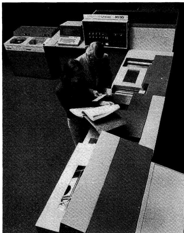
The basic UNIVAC 90/30 configuration includes a processor with 32K bytes of MOS memory, CRT system console, 500-cpm card reader, 500-lpm printer, and two 8418 disk drives with a total capacity of 57.8 million bytes. Also shown here is an optional card punch.
