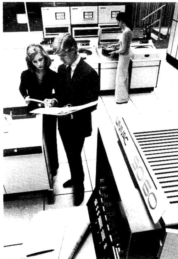
*The UNIVAC 90/60, designed and priced to be an attractive alternative to the IBM 370/135, offers from 131K to 524K bytes of MOS main memory with a cycle time of 600 nanoseconds per 4-byte access. The same memory is used in the faster UNIVAC 90/70.*
