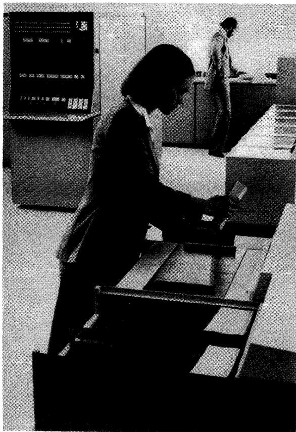
*UNIVAC's large-scale 90/80 computer system is now available in three models, the 90/80-2, 90/80-3, and 90/80-4. The 90/80-3 provides about the same performance level as the earlier single-model 90/80, while the 90/80-2 provides about 25 percent less performance. The 90/80-4 is a high-performance version that includes a high-speed buffer (cache) memory and provides about 35 percent greater performance than the 90/80-3.*
