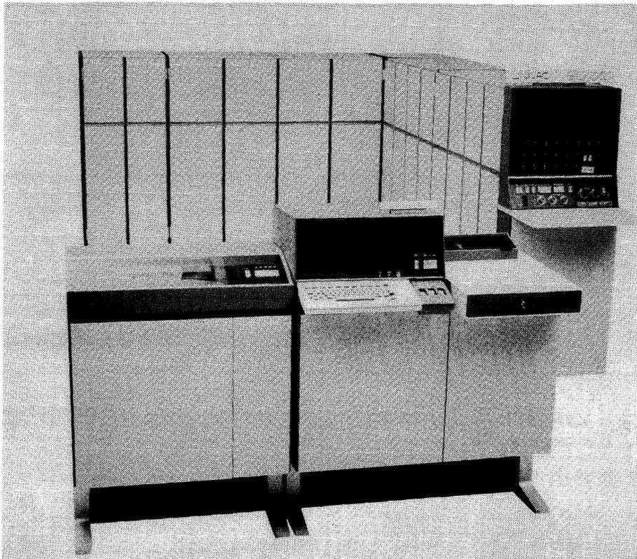
*Univac's 90/60 represents the low end of the company's line of large-scale, byte-oriented computer systems. The 90/60 and the lookalike 90/70 compete with IBM's System/370 Model 148 and the Model 3031 processor.*
