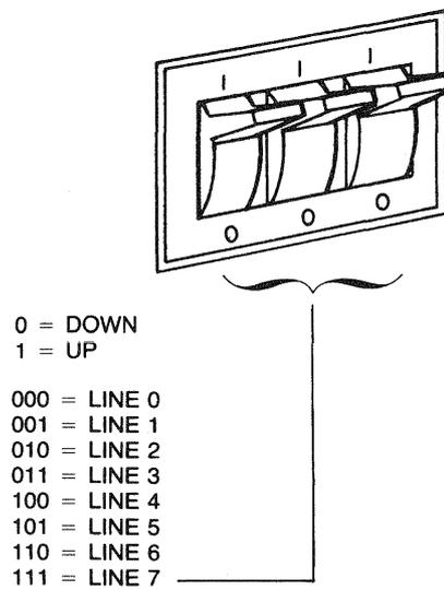
**Figure 1-2. Multiline Select Switch Settings**
