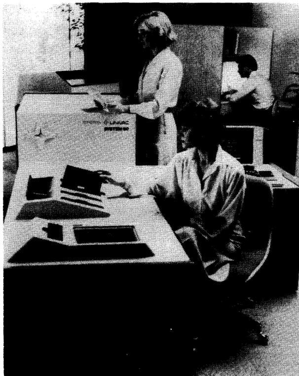
The minimum System 80 configuration consists of a central processor with 262K bytes of main memory and microprocessor-based control units connected to a 118-megabyte integrated disk storage subsystem, console workstation, diskette unit, and printer.
