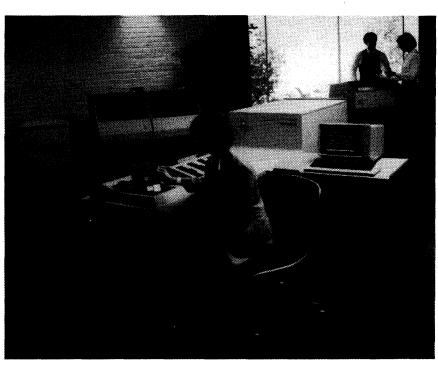
A minimum System 80 configuration consists of a central processor with 256K bytes of memory, a console workstation, an integrated 118-megabyte disk drive, a diskette drive, a printer, and associated control units. Magnetic tape drives, card reader/punches, and additional workstations, disk drives, diskette drives, and printers can be added.
