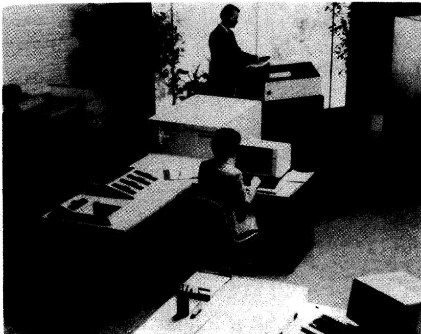
The System 80 equipment is designed for use either in a computer room or in a controlled office environment. In addition to the standard console workstation in the center of the photo, up to 39 CRT workstations such as the one at lower right can be cable-connected to the system at distances of up to 5000 feet.
