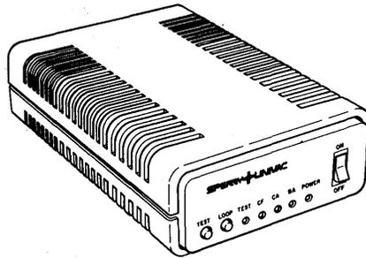
Features of the DCM include switch-selectable transmission speeds, the capability of operating with an internal or external clock, and patchable operational options.
