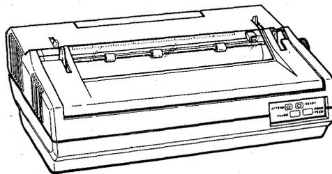
Pressure-sensitive switches are located conveniently on the front control panel. The plastic daisy-wheel print mechanism can print up to 96 different characters in various fonts and pitches. Eight character sets are available: U.S.A., United Kingdom, France, Germany, Italy, Denmark/Norway, Sweden/Finland, and Spain.
