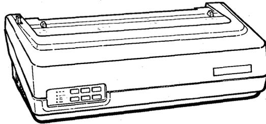
The printer can operate at 6 or 8 lines per inch vertical spacing and at 10, 12.5, or 16.6 characters per inch horizontal spacing. This printer includes the following international character sets, which are operator selectable: U.S.A., United Kingdom, France, Germany, Italy, Sweden/Finland, Denmark/Norway, and Spain. For more information, see the Model 25B printer general description, UP-10693.
