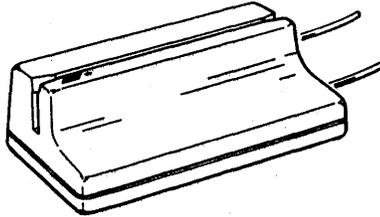
A device address code is not required for the magnetic stripe reader because the data is treated as keyboard entry. Input from the reader to the UTS 30 cannot be activated by a host processor, since operator intervention is required to generate the input data.
