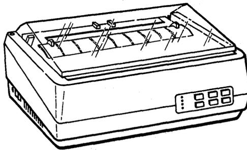
The printer prints at 10, 12.5, 16.7, and 20 characters per inch. It can also print at 5, 6.25, and 8.3 characters per inch. Line spacing can be set at 6 or 8 lines per inch. The printer prints a 96-character set with special characters for the following international character sets: U.S.A., United Kingdom, France, Germany, Italy, Denmark/Norway, Sweden/Finland, and Spain. For more information, see the Model 15 printer general description, UP-10201.
