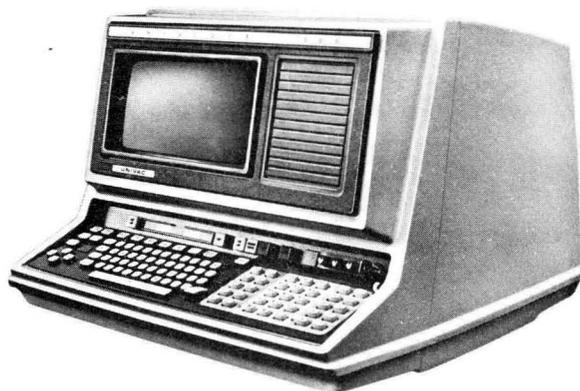
Figure 1-1. UNISCOPE 300 Visual Communications Terminal
