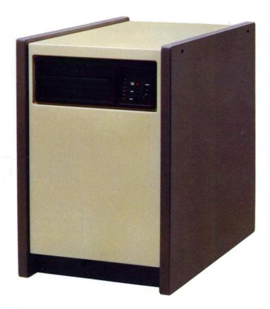
The SPERRY UTS 4020 is a microprocessor-based cluster controller designed for real-time, on-line interactive processing and local processing. Inasmuch as it allows user program and peripheral device sharing, systems with optimal cost performance can be configured to satisfy a wide range of application requirements. The basic components and expansion features of the UTS 4020 are:
