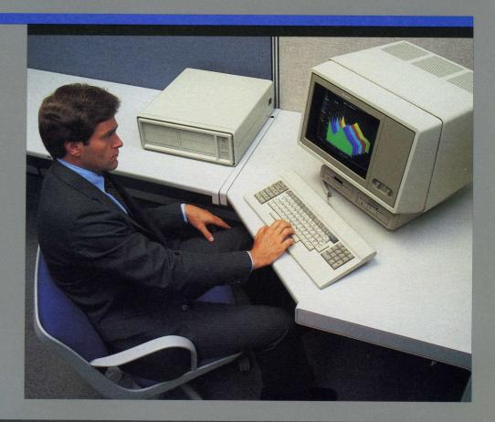
The UTS 60 programmable terminal provides outstanding color and graphics at extremely fast speeds. It uses the 16/32-bit Motorola MC68000 microprocessor as its central processor and the Zilog Z80 as a secondary processor to control the peripherals and the video section of the system.
