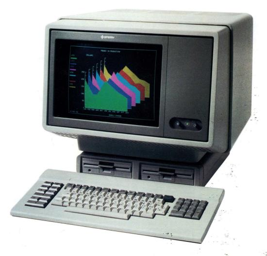
The SPERRY UTS 60 display station is a powerful and versatile color/graphics terminal system. It offers up to 2M bytes of memory and is totally programmable, making the UTS 60 an extremely useful interactive color/graphics terminal and stand-alone business computer.
