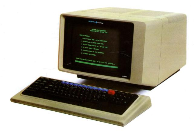
The SPERRY UNIVAC UTS 40 is a microprocessor-based intelligent communications terminal which is user programmable with up to 64K bytes of user memory. It supports a wide range of peripheral devices including printers, diskette subsystems and magnetic stripe reader. Programming of the UTS 40 is accomplished easily, using COBOL. Hence, this device combines the attributes of a data communications terminal with many features of a desktop computer.
