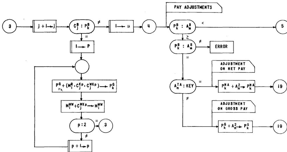
③ to ④ checks whether additional clock-card items pertain to the employee. ④ to ⑤ determines whether or not an adjustment item is present for this employee, and, if so, makes this adjustment on net or gross as indicated by the type-of-adjustment key.
