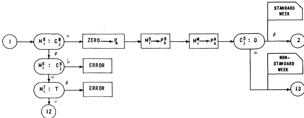
The first two operations serve to match the master file item with its appropriate clock-card item, and then to determine whether a standard work-week applies. The alternatives labelled "error" occur whenever a master-file item of a non-terminated employee has no clock-card item, or vice-versa.
