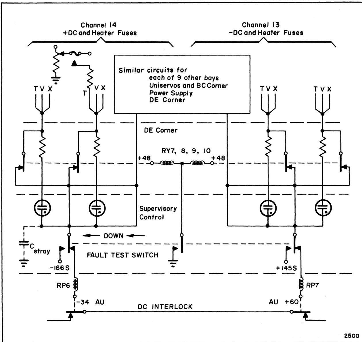
**Figure 2-37. D-C and Heater Secondary Fuse-Fault Circuit**
