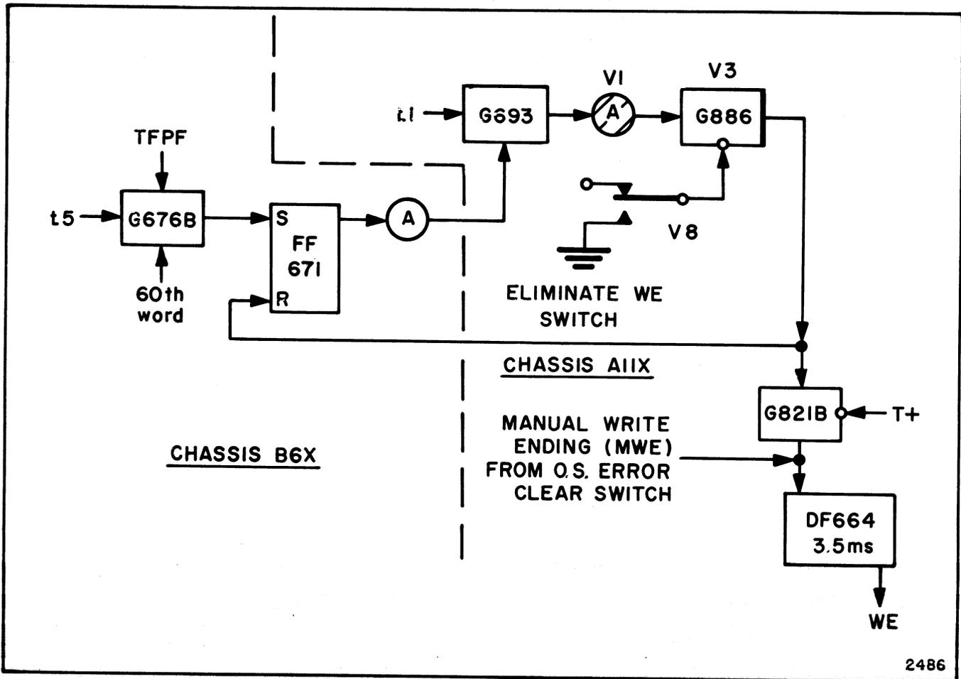
Figure 2-22. Write-Ending Circuit
