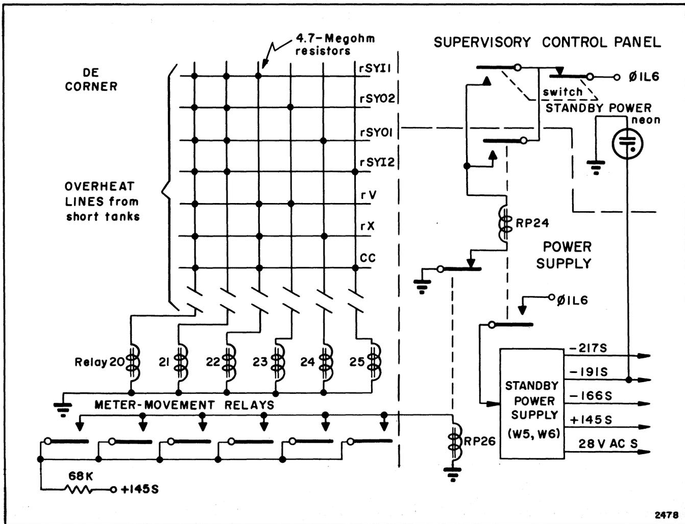
Figure 2-14. Short-Tank Overheat System, Schematic
