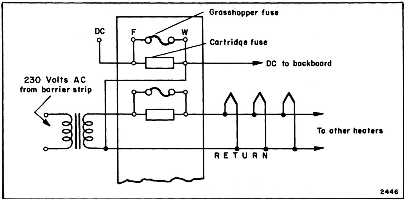
Figure 1-12. Minimizing of Heater-to-Cathode Arcing
