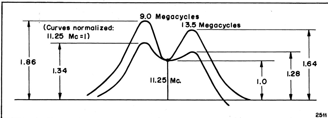
Figure 3-4. Frequency-Versus-Amplitude Plot for Amplifier Response Check
