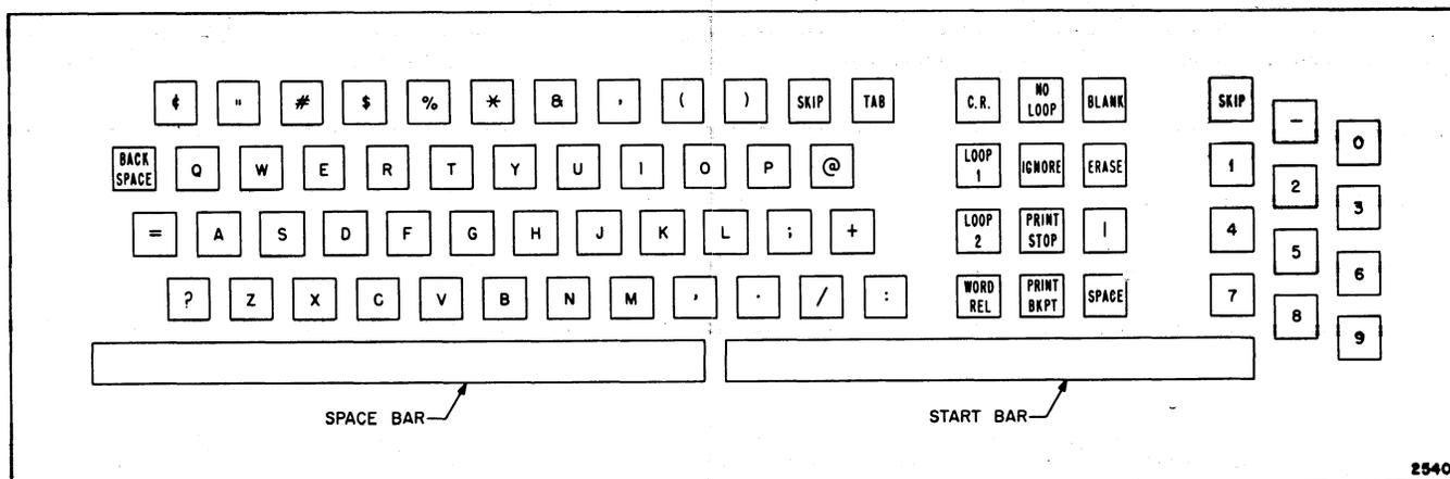
**Figure 5-2. Supervisory Control Panel Keyboard**
