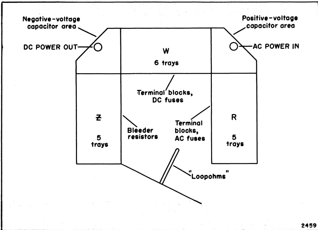
Figure 1-25. Power-Supply Layout
