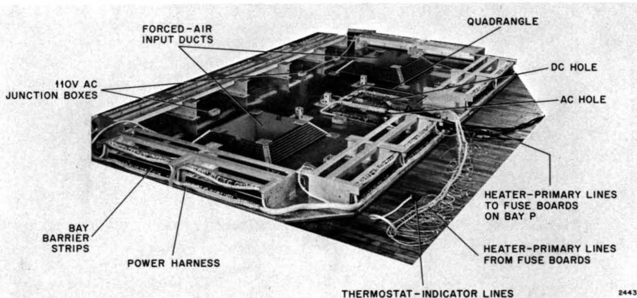
Figure 1-9. Sub-Floor Assembly
