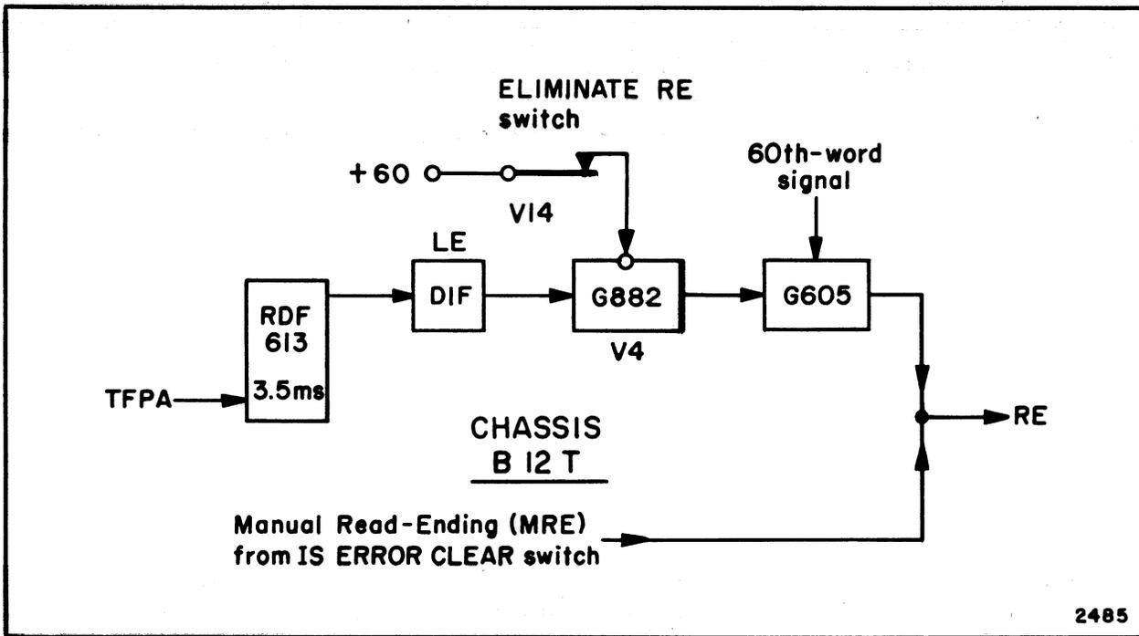
Figure 2-21. Read-Ending Circuit and ELIMINATE RE Switch
