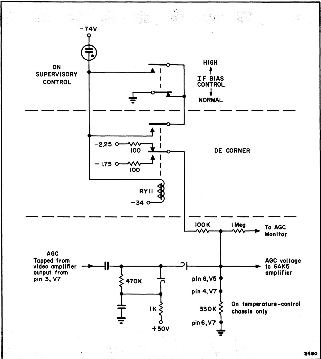
Figure 2-16. Bias-Shifting Circuit
