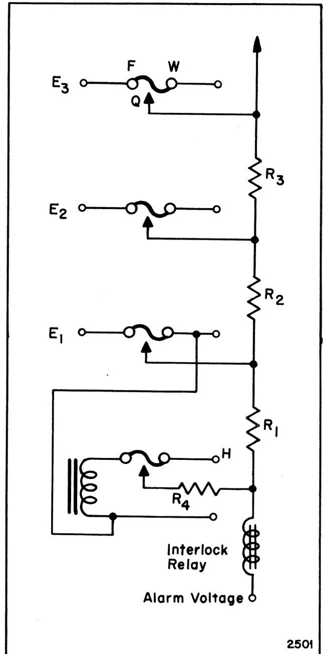
Figure 2-38. Constant-Current Circuit
