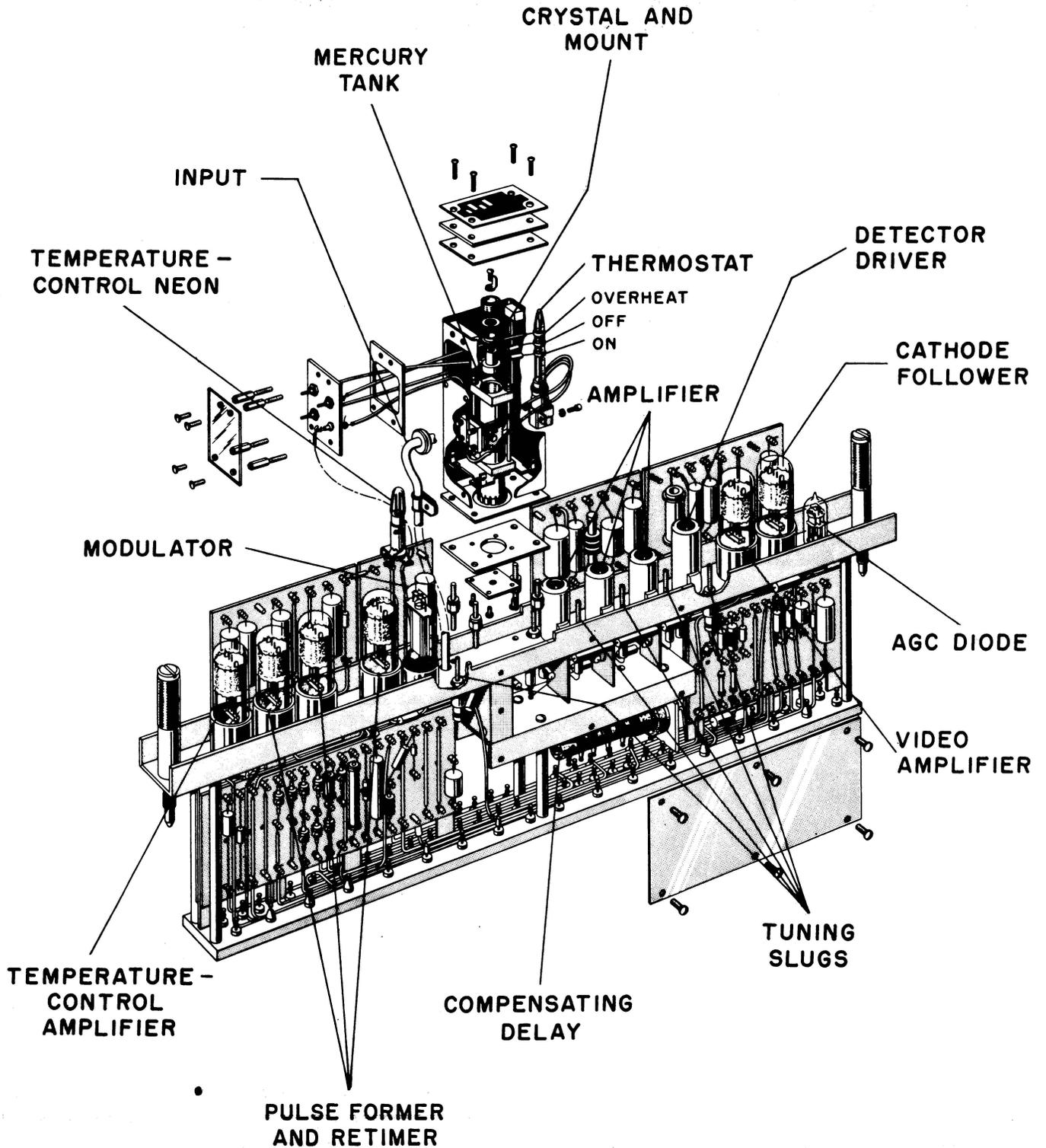
Figure 2-11. Short-Tank Register Chassis
