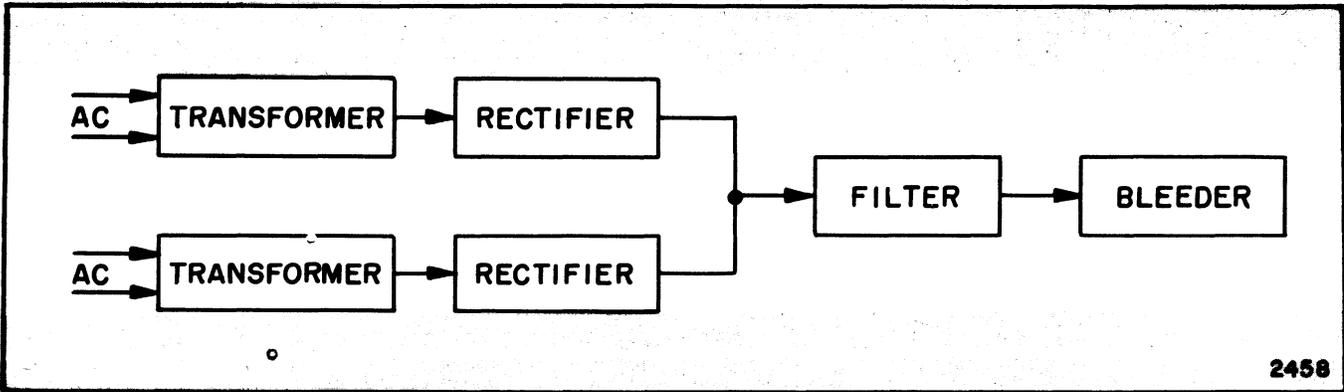
Figure 1-24. Power-Supply Rectifier Circuits
