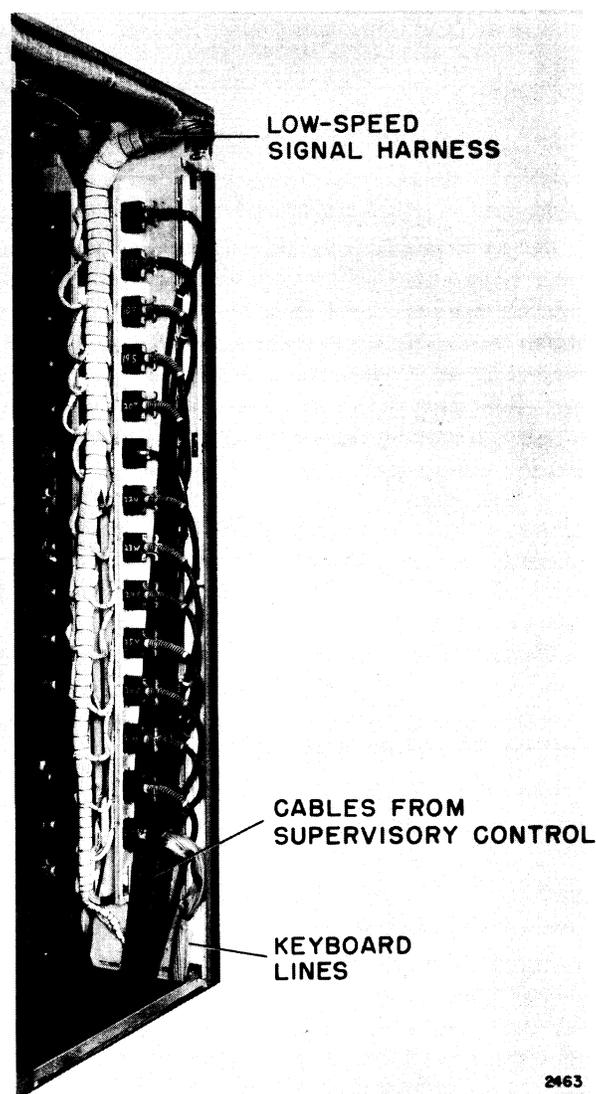
Figure 1-29. Supervisory Control Panel Connections to Bay A
