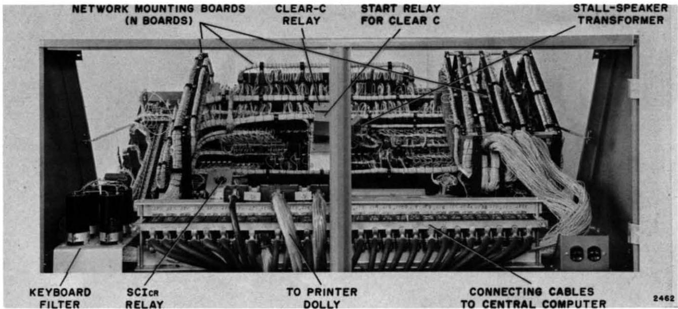
Figure 1-28. Supervisory Control Panel Wiring, Rear View
