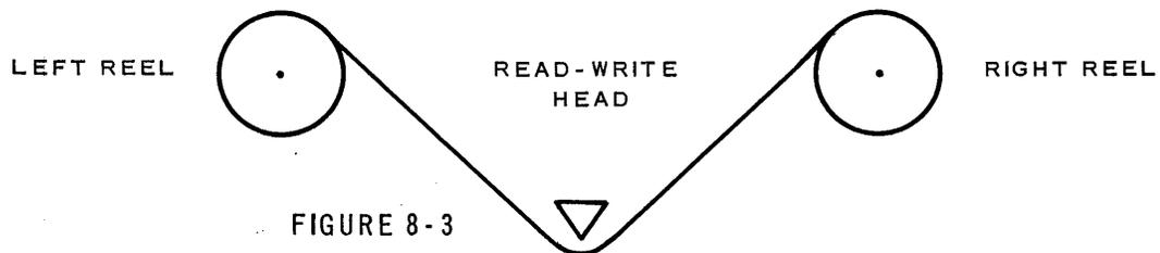
Since the right hand reel is permanently fixed, a tape to be read from or written on is mounted on the left hand reel. The tape is connected to a pre-threaded leader which is fastened to the right hand reel. Because of the pre-threaded leader, removal of a reel and the mounting of a new reel takes only one half minute.
