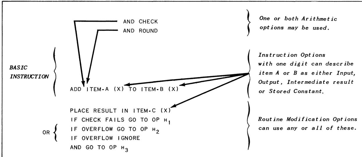
Another good example is the power and flexibility of the Compare instruction. In this case, with one FLOW-MATIC statement, the programmer can code up to 25 equality-magnitude comparisons by merely using the conditional transfer options.
