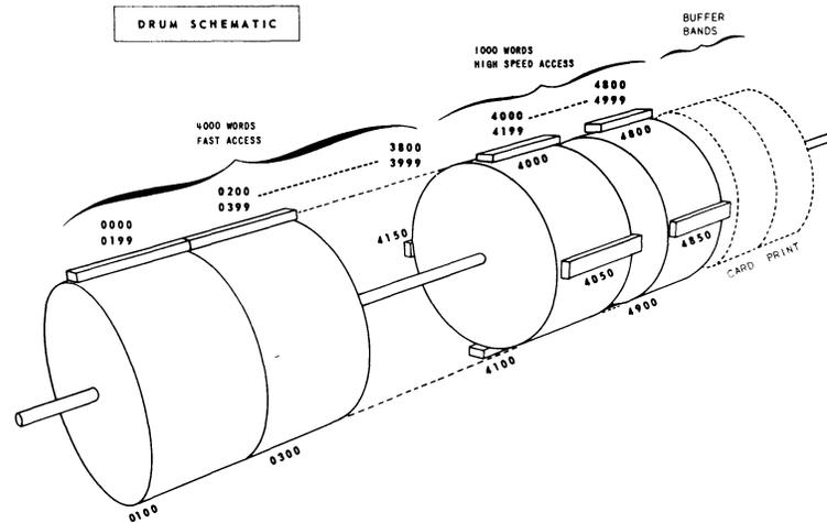
*The Fast Access Area* -- consists of 20 bands of information for a total of 4,000 words. Average access time to information in this area is 1.7 milliseconds. Programs and tables are normally stored in this area.
