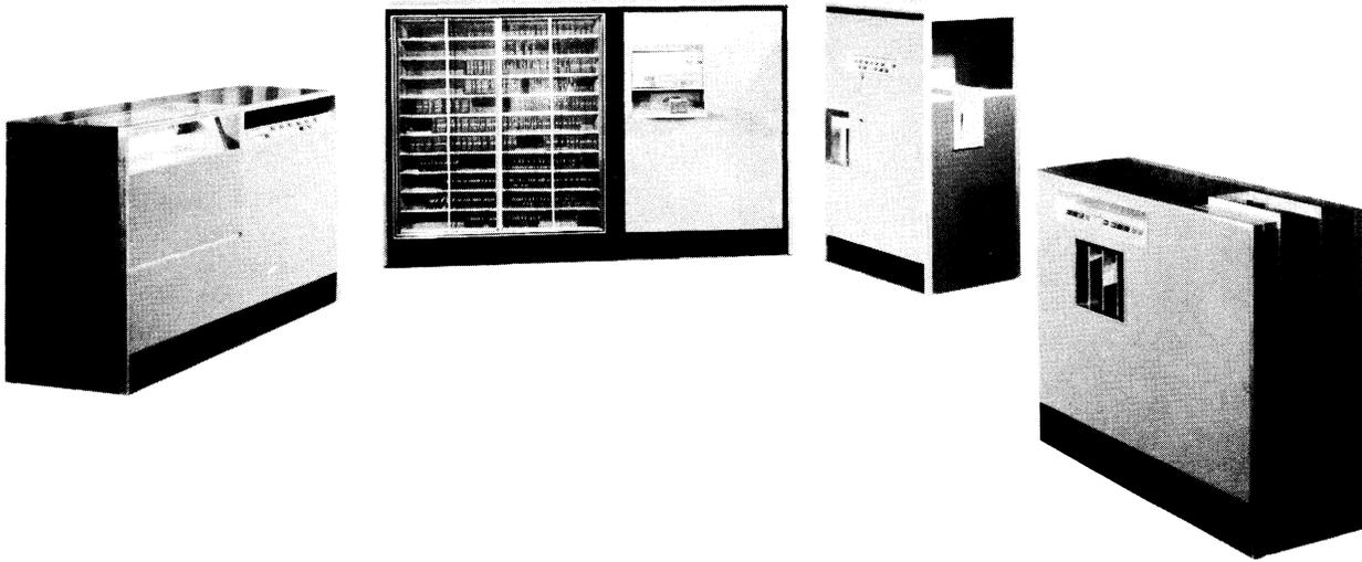
The UNIVAC Solid-State Computer is a general-purpose, alpha-numeric, digital, punched-card computing system. It is composed of four individual units: a Central Processor, a High-Speed Reader, a Read-Punch Unit, and a High-Speed Printer. The units are connected to form a completely on-line, balanced data-processing system.
