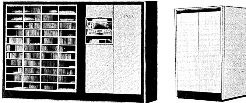
Figure 3-1. Central Processor and Core Storage Unit
