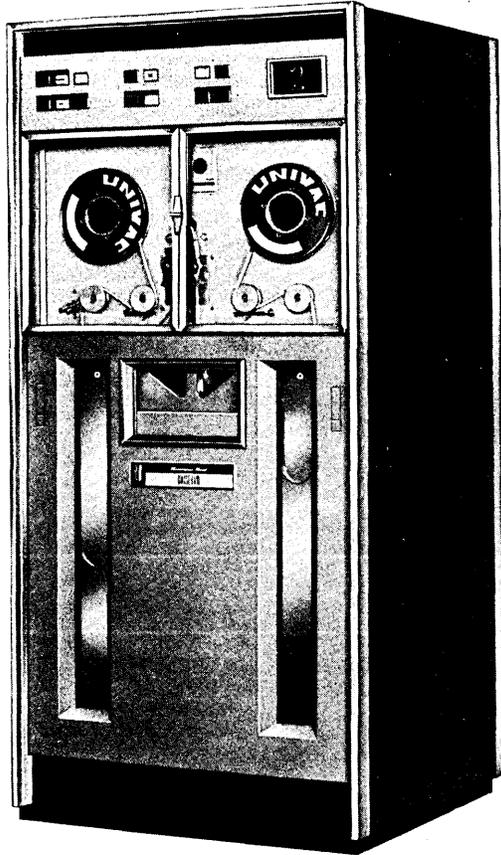
Figure 3-2. UNISERVO Tape Unit
