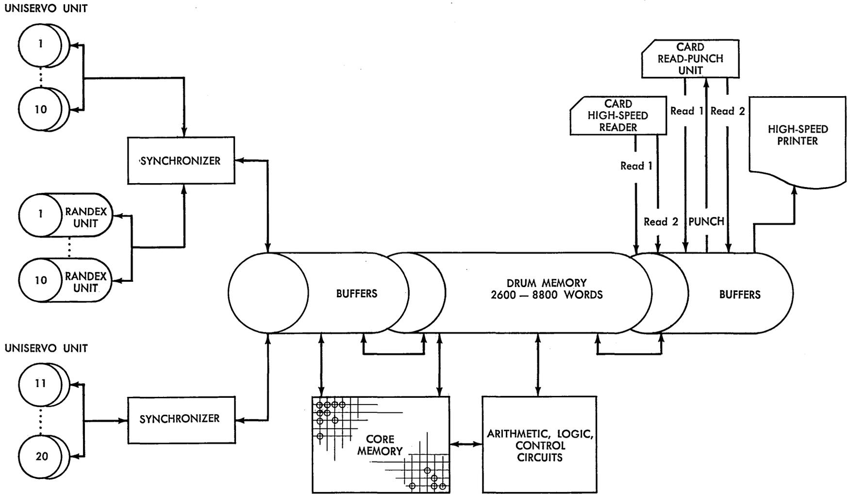
Figure 5-1. Schematic, Data Flow
