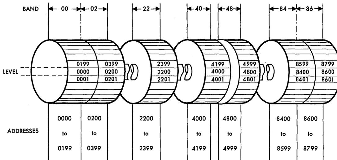
Figure 4-5. Schematic, Magnetic Storage Drum
